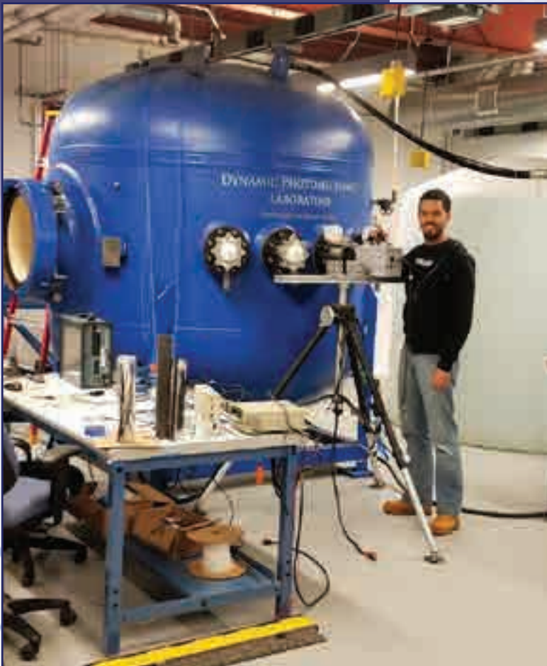
Graduate student, and now a full-time employee at NUWC Newport, preparing the high-speed cameras for experiments on the implosion process of hydrothermally degraded composite tubes.
