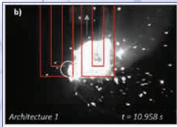
Images captured with a high-speed camera of a lateral thermite ignition initiation on a serpentine RMA in a time span of 0,7 s.
