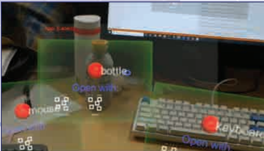
AR overlays on automatically recognized objects on the HoloLens (left), and system architecture for the planned AR equipment maintenance application (right).
