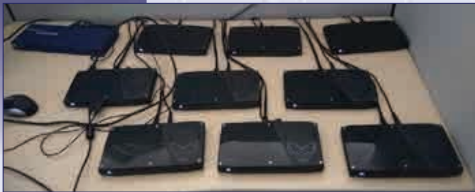
Figure 1: The Mandrake edge cloud, consisting of nine Intel NUC6i7KYK NUCs and a Netgear GS116 gigabit switch.
