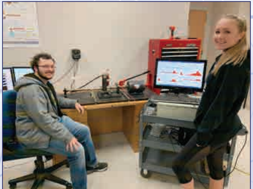
Graduate student and undergraduate student working on the bearing degradation test bed which incorporates both an accelerometer and acoustic emission sensors.
