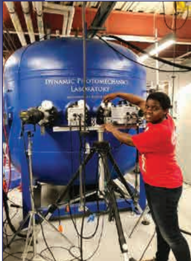
A 2.1-m-diameter semi-spherical pressure vessel, with a maximum pressure rating of 1000 psi. Vessel is used to simulate the open ocean environment at different depths. Implosion and UNDEX behavior of weathered elastomeric coated cylinders are investigated using this facility.
