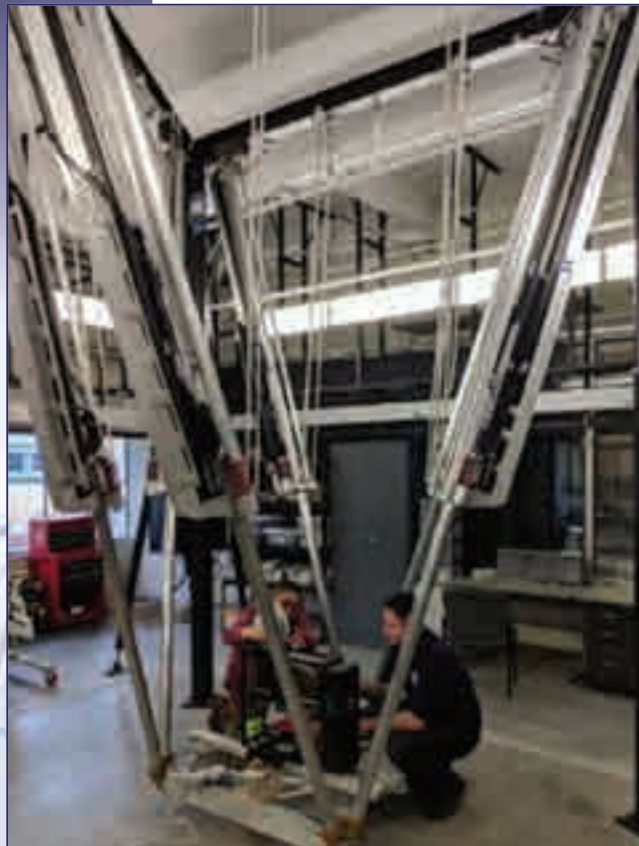
Mounting the Lutzbot Taz 6 on the Reverse Stewart Platform.
