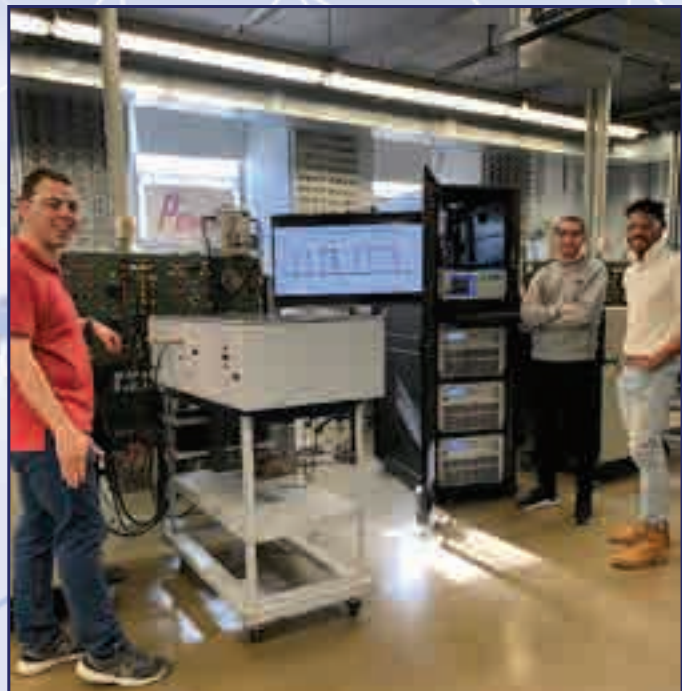
Laboratory testing of the AC/DC microgrid, one-rack setup where different combinations of types and amounts of controllable loads are varied and subsequent actuation delays are captured. Platform and repeatable test procedures are developed by graduate students.
