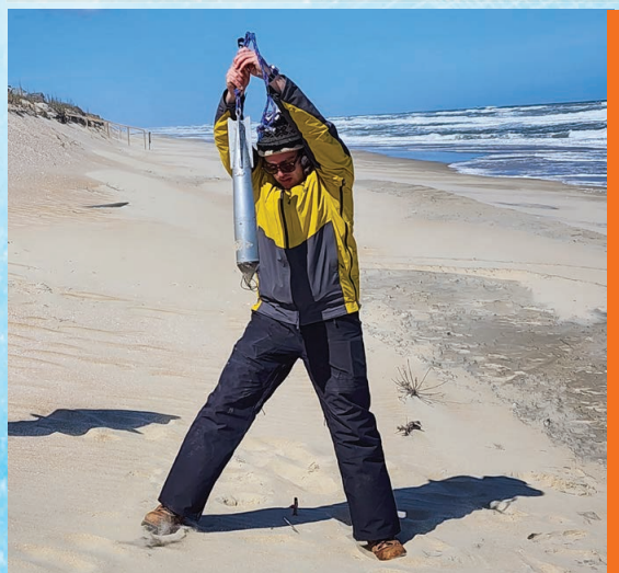
VT student dropping the PFFP BlueDrop on a windy day in Duck, NC.
