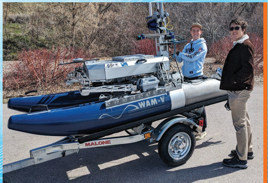
NEEC students getting ready to deploy a Wave Adaptive Modular Vessel (WAM-V) for experimentation.
