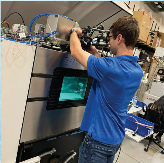
PhD candidate setting up the IR camera on the EOS M290 DMLS machine
