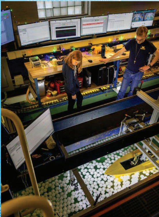
Students running the destroyer bow model through a simulated broken ice field in the Aaron Friedman Marine Hydrodynamics Lab at the University of Michigan.
