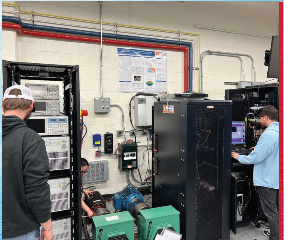
Students monitoring flywheel-coupled motor generator sets for power quality measurements under various pulsed load conditions.
