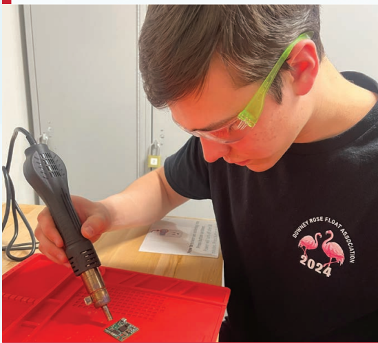
Student soldering components for the synthetic aperture radar (SAR) camera.
