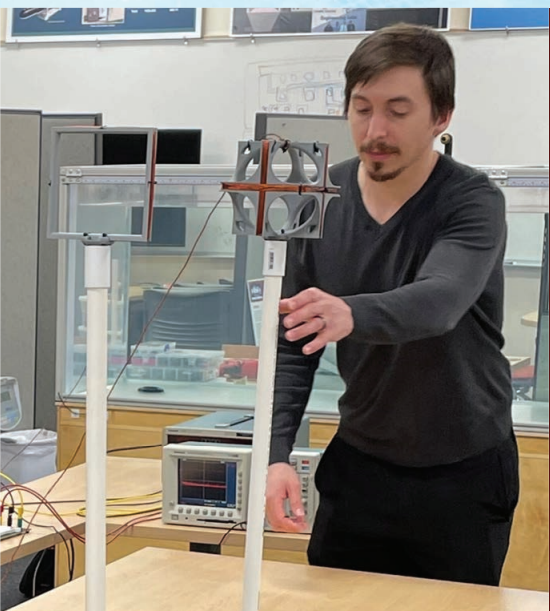
Student adjusting the orientation of Magnetic Induction Coils.
