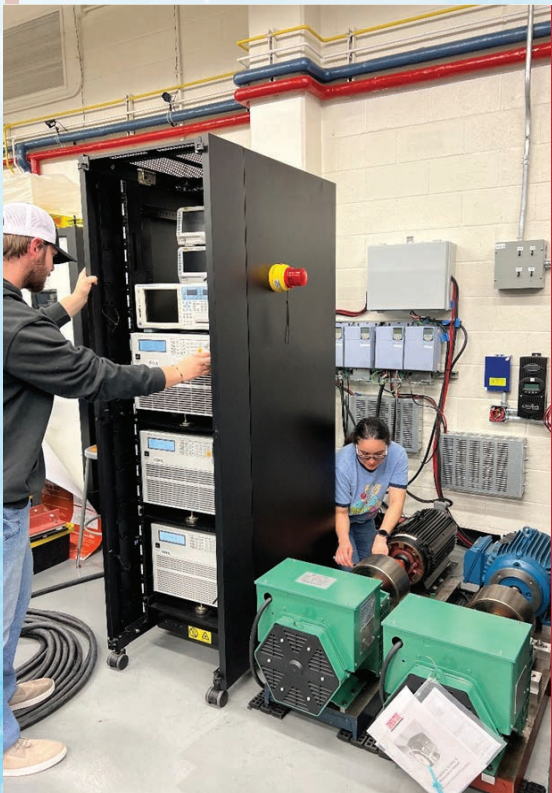
Student connecting a flywheel-coupled multi-output generator's controller to synchronize with UTA's test bed.
