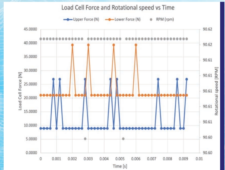
Plot showing the computed force and the computed rotational speed from the voltage signals.
