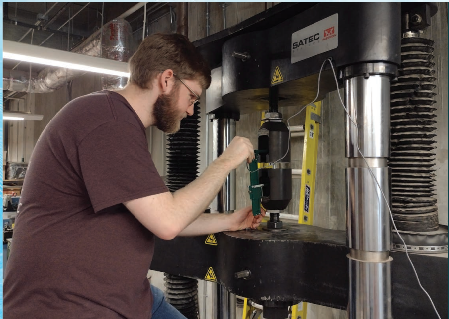
Master's student preparing a bolt tension test.
