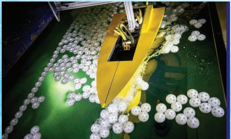
The destroyer bow model under test in the simulated ice field (wiffle balls).
