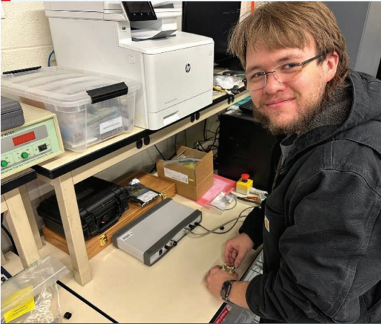
Student collecting permittivity data using a vector network analyzer (VNA)
