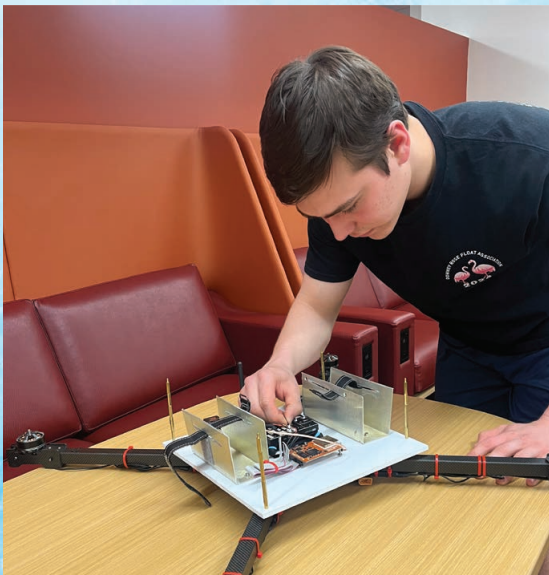
Student working on the custom drone that will carry the synthetic aperture radar (SAR) camera.
