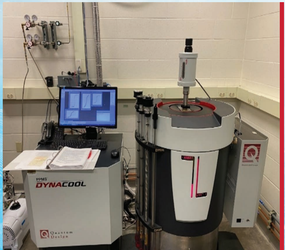
Experimental setup for in-plane vibrating sample magnetometry measurements.
