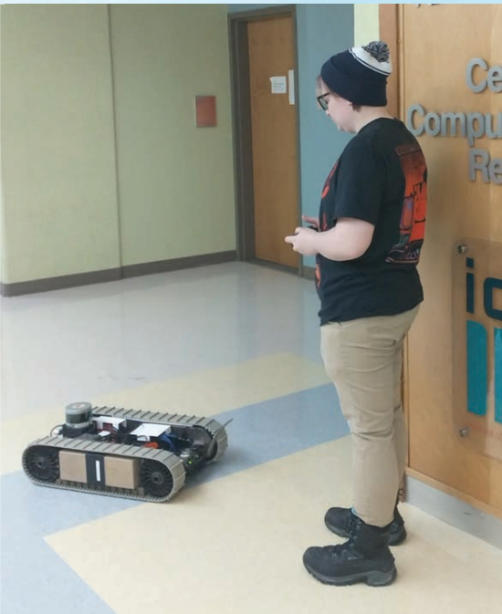
Michigan Tech student performs an indoor SLAM experiment using the GVRbot.
