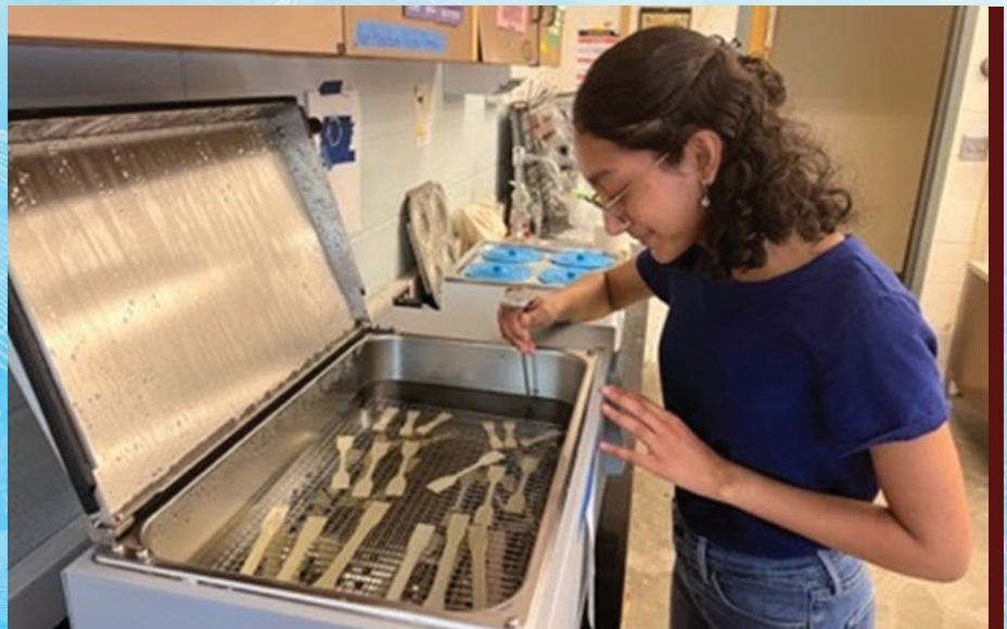
Undergraduate in Materials Science and Engineering student, extracting samples from the marine aging bath
