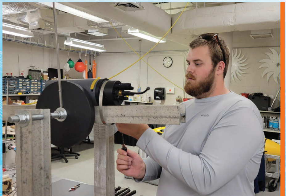
FAU NEEC student is developing a test rig for testing a vehicle attitude sensor package he has developed.
