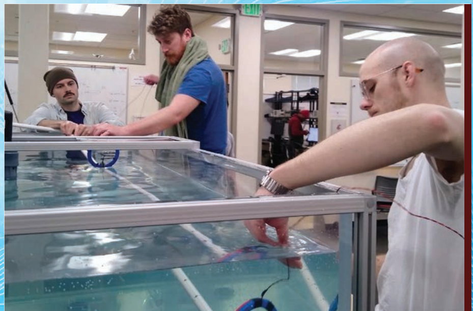
Students working on MI communication in saltwater tank. The communication coils are at two ends of the tank.
