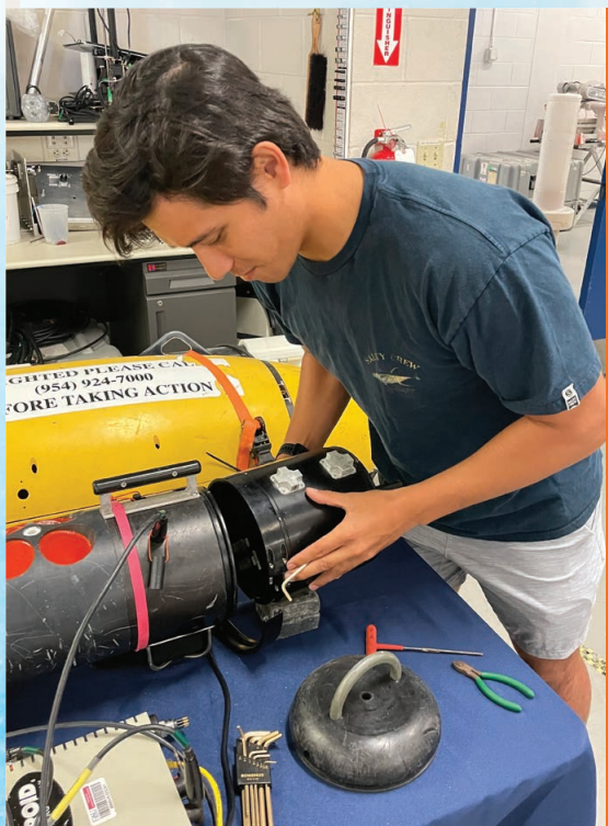
FAU NEEC student checking the alignment of a sensor package on a REMUS AUV.
