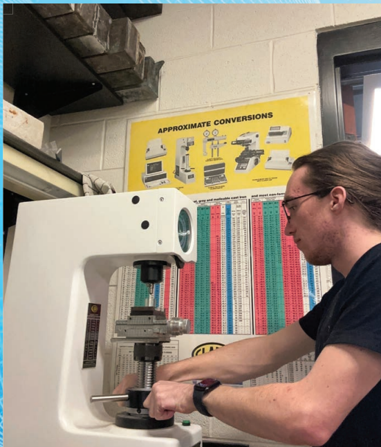
Undergraduate student performing harness testing on bolt sample.
