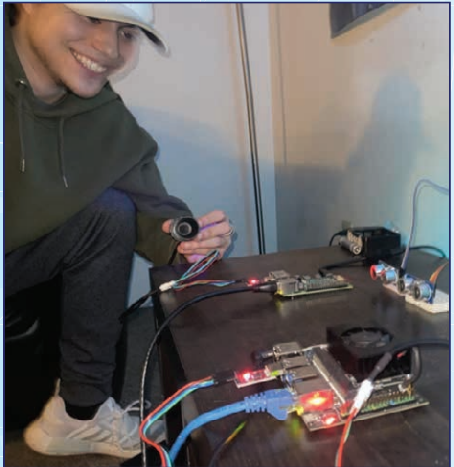
Student working on his senior design project: side-channel sensing of an embedded system with peripherals like a sonar transceiver.
