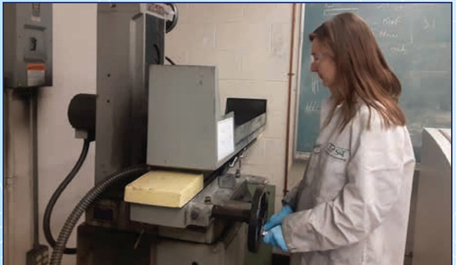
Graduate student operates a diamond wheel surface grinder to prepare densified ceramic matrix composite specimens for characterization and testing.
