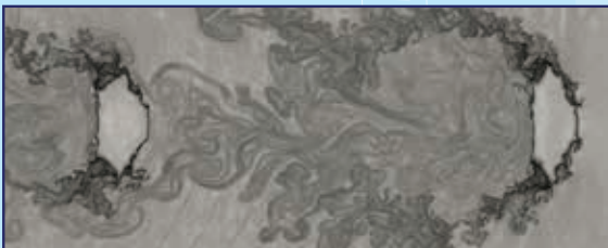
Interactions between shock wave traveling at a Mach number of 1.47 and two water droplets separated by a distance of 6.8D (contours show density gradients).
