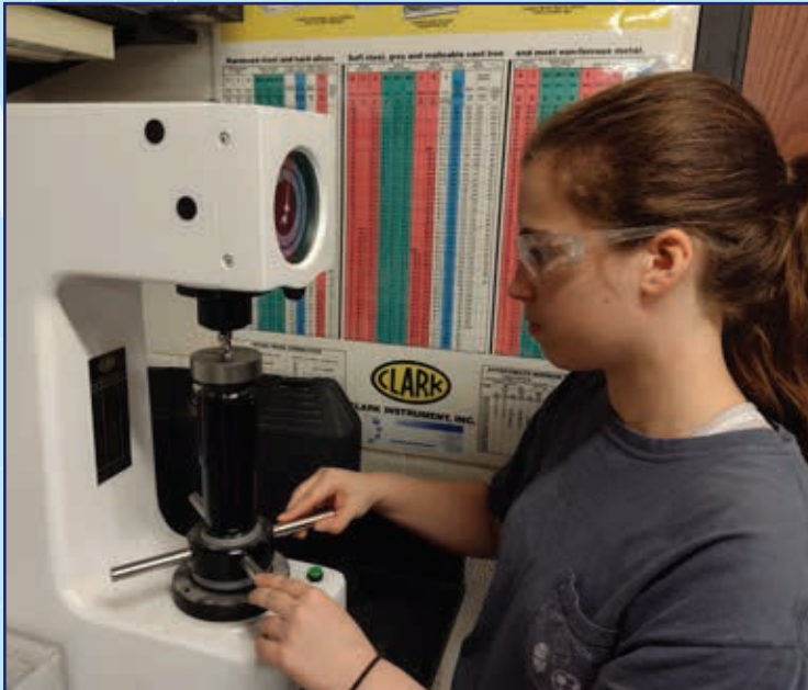
Undergraduate student performing harness testing on bolt sample.
