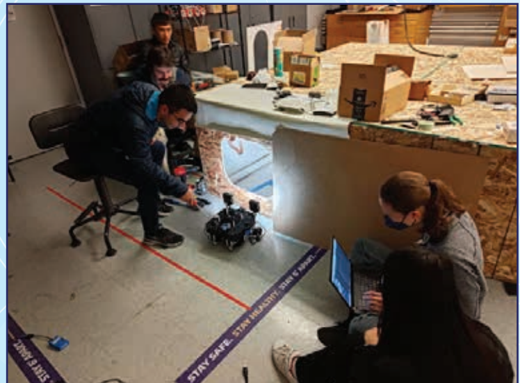
Senior capstone project team working on testing a low-cost robotic inspection system for a scaled-down water tank in a dry docked vessel.
