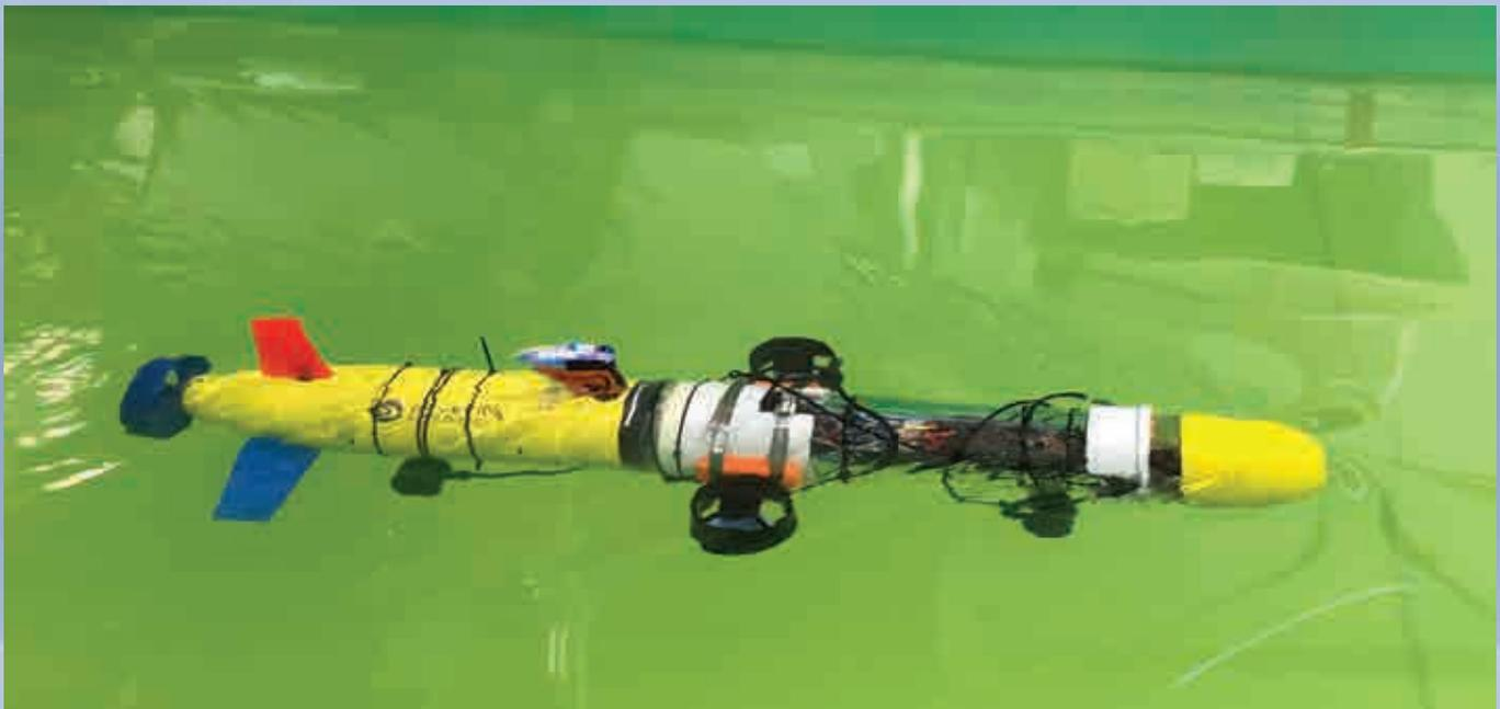
Micro-AUV testbed with added cross-body thrusters and buoyancy control engine for in water testing of over-actuated depth control algorithms.
