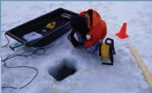
Student running an experiment to localize an under-ice ROV using its acoustic signature in the middle of the Keweenaw Waterway at Great Lakes Research Center.
