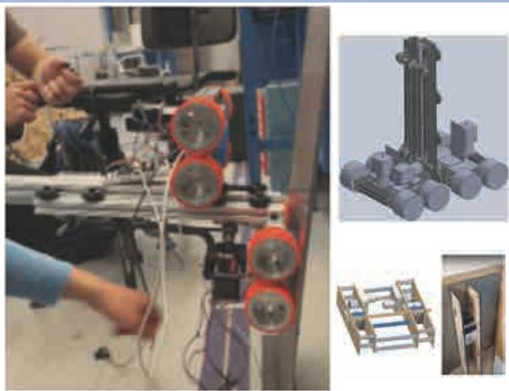
Magnetically actuated wall climbing robot designs and prototypes developed by two UW Mechanical Engineering senior undergraduate capstone project teams.
