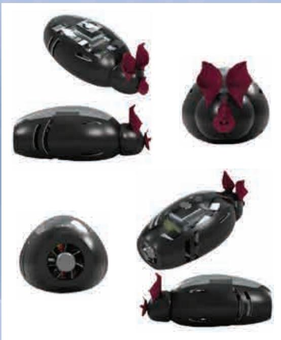
Rendering of the CAD model for the shell and interior for the next-generation prototype of the biomimetic sonar head with soft-robotic, tension-driven actuation.
