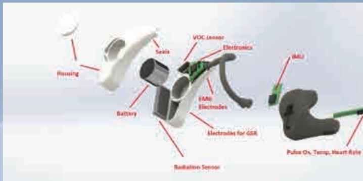
Schematic of device design.
