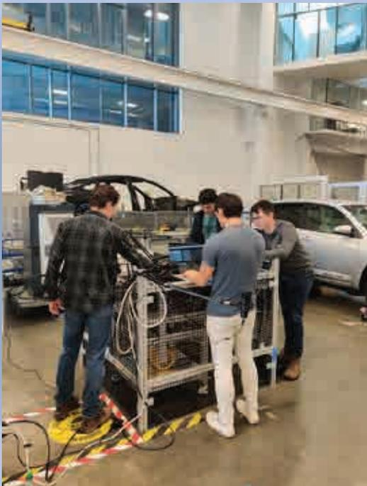
Graduate students working on the COVIA project collecting failure data from a bearing test rig at the Clemson University International Center of Automotive Research.
