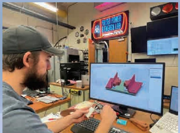
Masters student works on a solid model of this surface flashover test stand.
