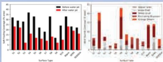
Left: Hard fouling coverage on brush-functionalized SEBS elastomers (S1-S10). Control samples were a bare fiberglass panel (“blank”), unfunctionalized elastomer (SEBS), and elastomer functionalized with 1-2 mol% dopamine (SEBSDA). Right: Soft fouling coverage for the same samples, before and after cleaning with a water jet (calibrated to reproduce 11 knots).
