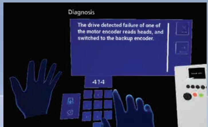
Right- and Left-handed user Hand Menus for inputting error codes while using a Hololens 2 device.
