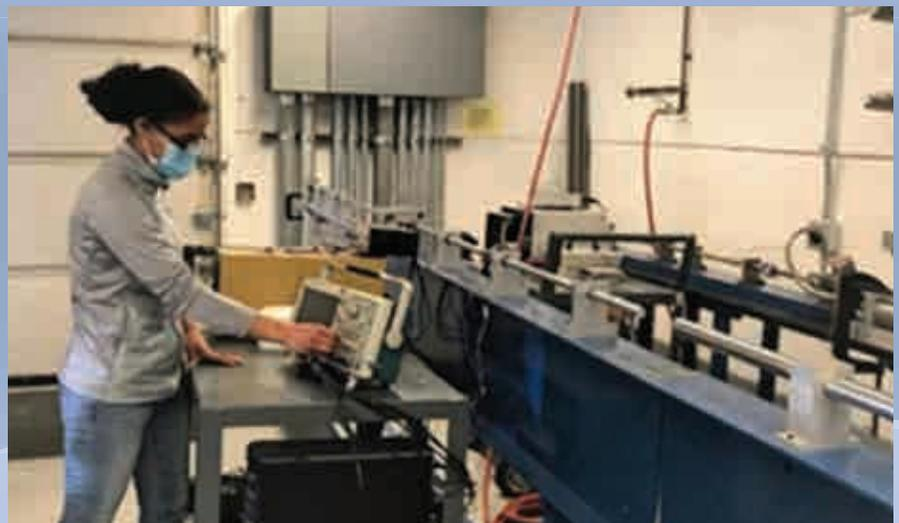
Undergraduate student in the department of mechanical engineering, conducting experiments on the Split Hopkinson Pressure Bar (SHPB) setup in the Dynamic Photo Mechanics Laboratory, URI. The SHPB setup is used for material characterization under dynamic loading conditions.
