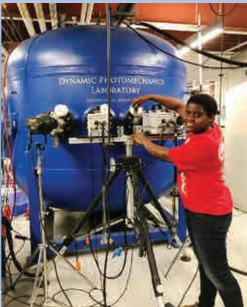
Dr. Irine Chenwi, setting up high speed cameras for implosion experiments in the pressure vessel. This tank is a unique facility in the Dynamic Photo Mechanics Laboratory – URI, which simulates an open ocean environment. It is designed to withstand pressures up to 1000 psi and experiments in task 3 of this project are conducted in this facility.
