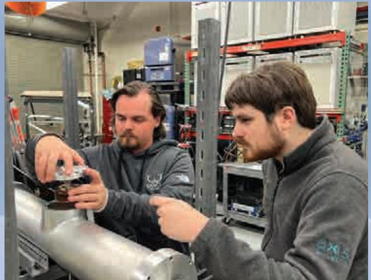
PhD students load an epoxy dielectric sample into the pulsed load section.
