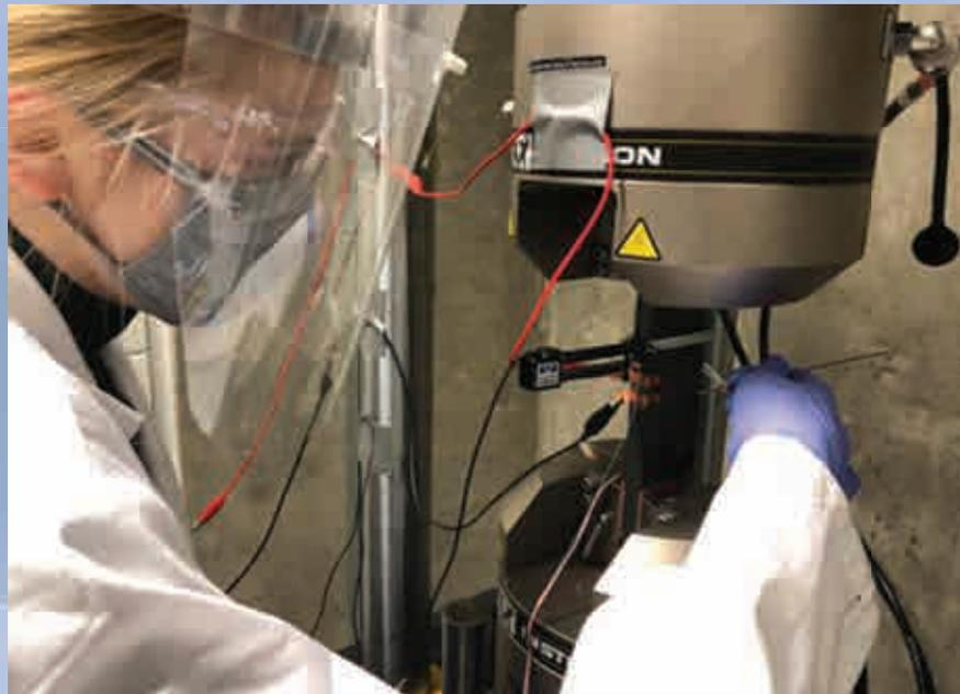
Undergraduate student performing mechanical testing to characterize the piezoresistive response of 3D printed components..
