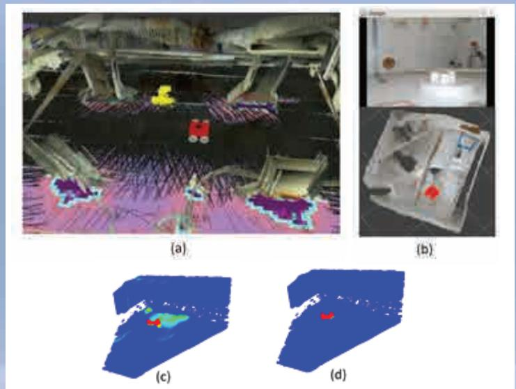
Visual simultaneous localization and mapping (SLAM) inside a poorly-illuminated confined space (water tank) in a marine vessel. (A) SLAM in progress for a ground robot in a simulated tank. (B) SLAM in progress for a robot in a physical mock-up tank. (C) Anomaly (power drill left behind in the tank by mistake, as shown in yellow) detection by training on a nominal CAD model. (D) Anomaly detection by training on an empty tank point cloud map.
