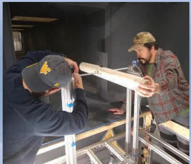
NSWC Dahlgren Division Scientist Graham McConnell and a WVU Graduate student work to install a missile model in preparation for wind tunnel testing at WVU.
