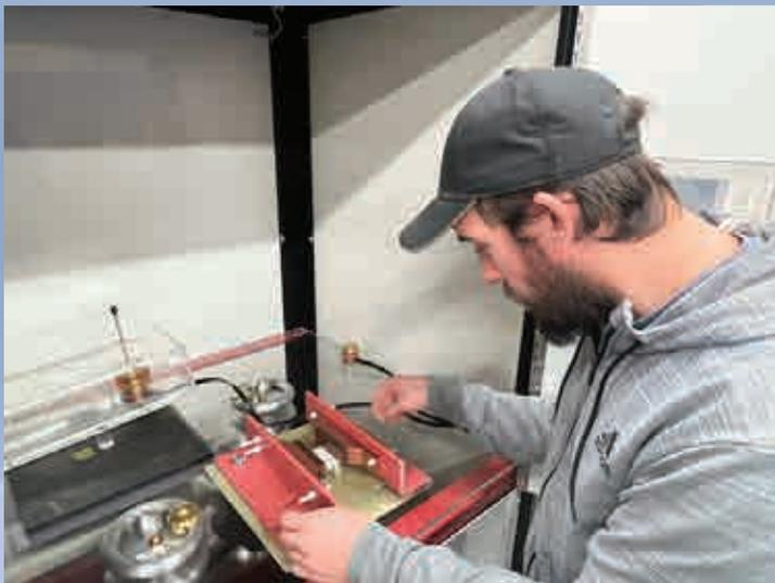
Masters student installs the physical flashover test stand into a dielectric hi-pot tester for experimentation.
