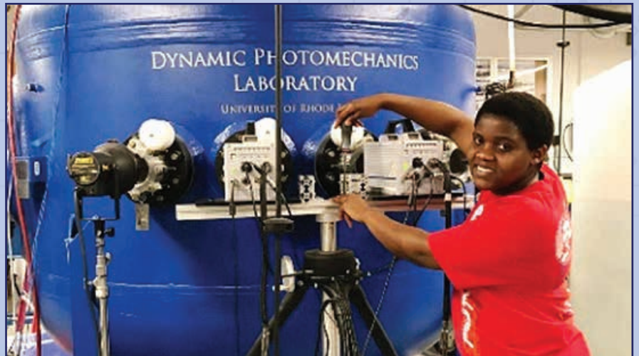
Student setting up high-speed cameras for implosion experiments in the pressure vessel. This tank is a unique facility in the Dynamic Photo Mechanics Laboratory, URI, which simulates an open ocean environment. It is designed to withstand pressures up to 1000 psi, and experiments in task 3 of this project are conducted in this facility.
