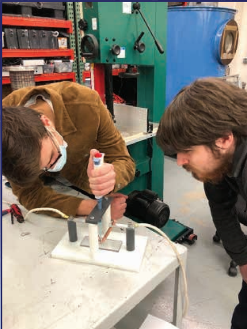
Students working with the testbed designed to replicate the International Electrotechnical Commission (IEC) 60112 standard.
