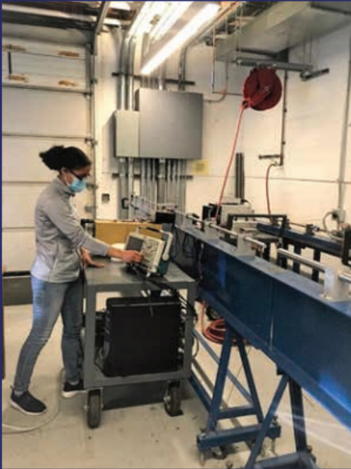
Our undergraduate student, in the department of mechanical engineering, conducting experiments on the Split Hopkinson Pressure Bar (SHPB) setup in the Dynamic Photomechanics laboratory, URI. The SHPB setup is used for material characterization under dynamic loading conditions
