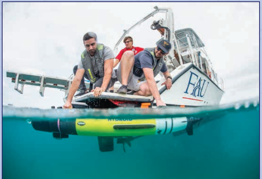
Students launch a REMUS 100 vehicle from a research vessel in order to conduct a magnetic navigation experiment.
