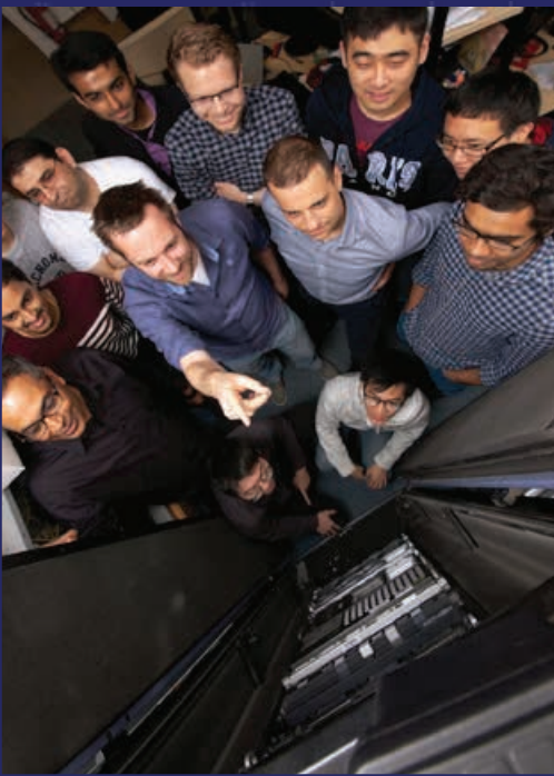
SSRG students including NEEC students and faculty members inspecting their rack-scale server testbed running Virginia Tech's Popcorn Linux operating system (NEEC-supported project).
