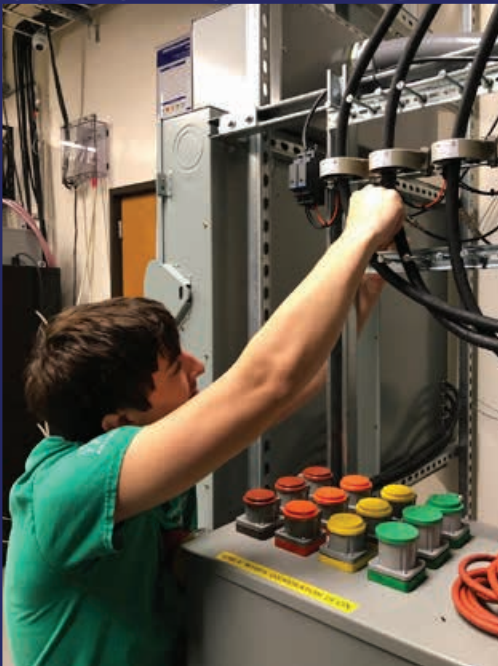
Student working on sensors attached to the output of a 150-kW electric motor-generator set.
