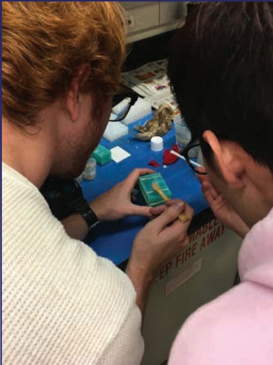
Making a flexible soft-robotic pinna using a silicone mould.
