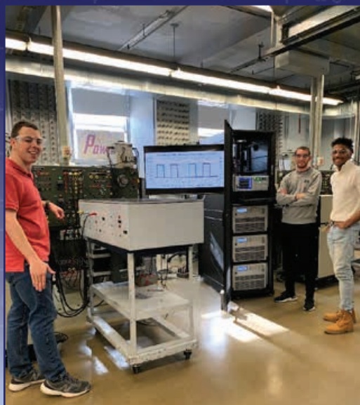
Laboratory testing of the AC/DC microgrid, one-rack setup where different combinations of types and amounts of controllable loads are varied and subsequent actuation delays are captured. Platform and repeatable test procedures were developed by graduate students.
