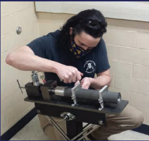
MS graduate student in Aerospace Engineering working on his new design of a ballistic launcher for unstable flight articles. This is a blend of a 40-mm grenade launcher and a Mann barrel with additional safety features incorporated into the design. It will eventually be used to launch test articles that have an unstable flight trajectory, and the flight data will be recorded with a system of Vicon cameras.
