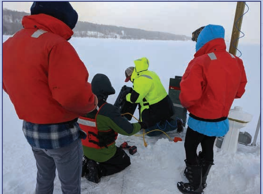
Michigan Tech students deploy the acoustic sensing unit for taking measurements of on-ice traffic outside the Great Lakes Research Center.
