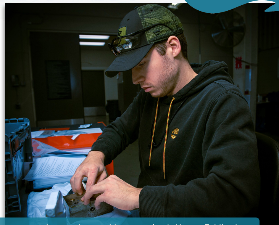
TRFB team member, marine machinery mechanic Hunter Feldbush reassembles a hydraulic actuator at TRFB.
