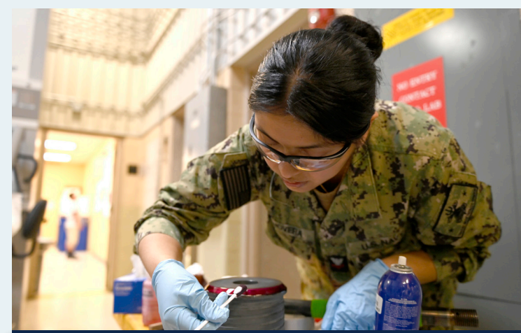
HT2 Andrea Pamo performs liquid penetrant testing for quality assurance.
