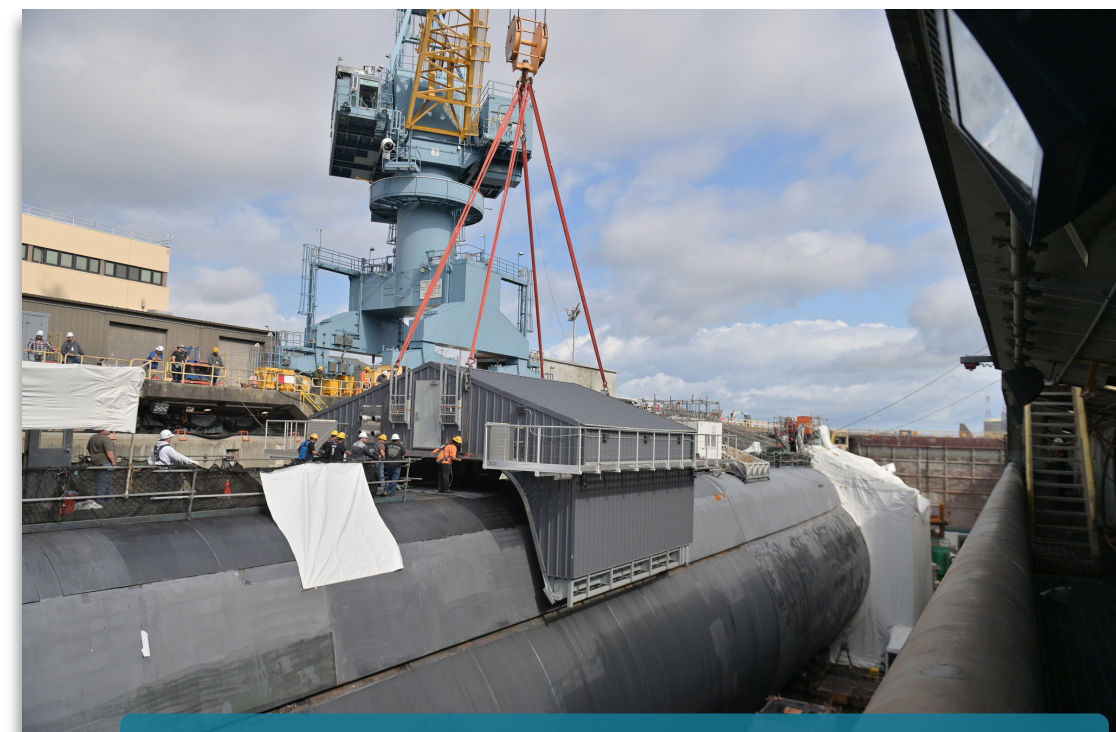
TRFB Lifting and Handling team members test a new paint enclosure on Delta Pier at TRFB.
