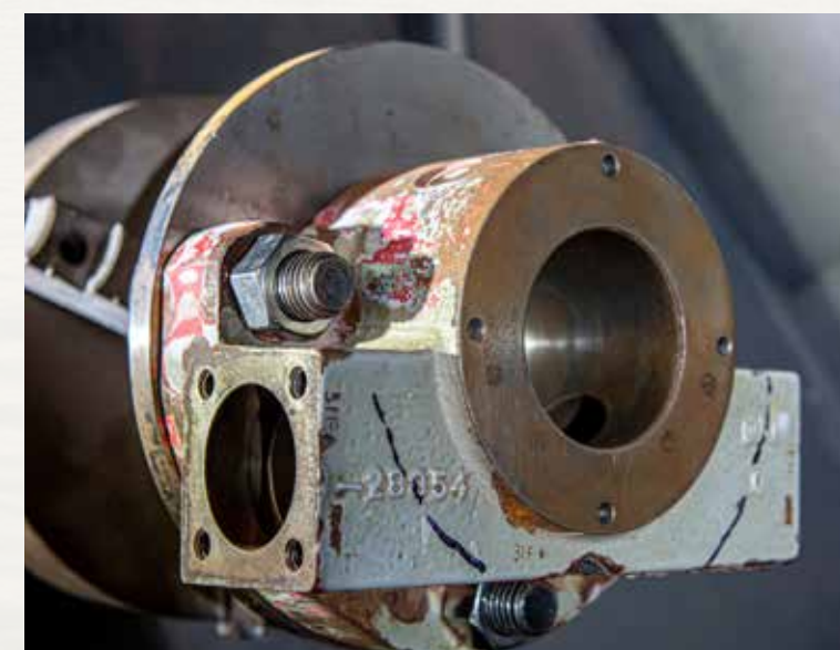
The actuator body component from Norfolk Naval Shipyard was repaired via cold spray at Penn State Applied Research Laboratory by shipyard machinists.(U.S. Navy photo by Shelby West)
