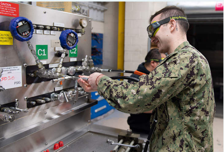
TRFB Sailor Machinist Mate 2nd Class Dakota Overturf tests a hydraulic activator while participating in the Navy Afloat Maintenance Training Strategy (NAMTS) program.
