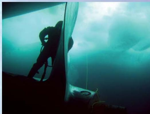
*Diver working on starboard CPP propeller.*
