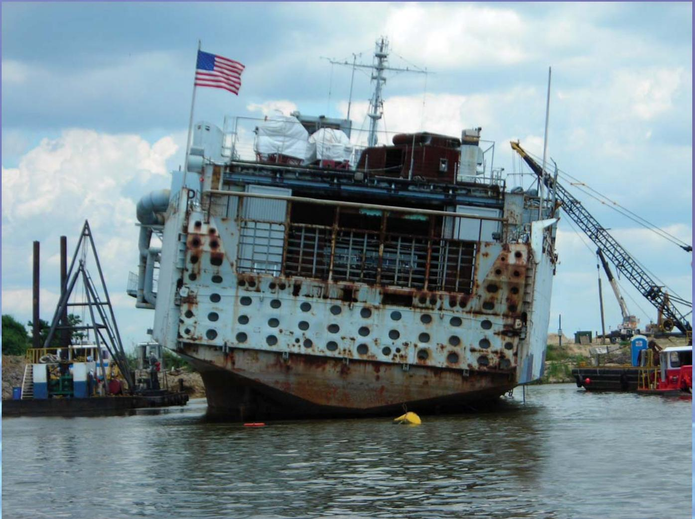
*View of EX-SHADWELL (LSD 15) stern as dredge work proceeds on the port and starboard side of hull. Note channel created on port side to facilitate salvage work to refloat ship.*
