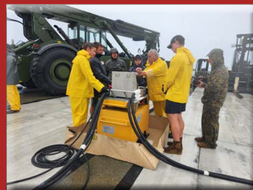
ESSM personnel familiarize MDSU divers with the controls for the linear pullers prior to use.
