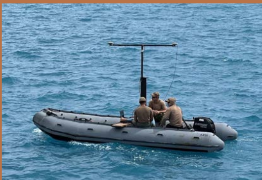
Hydrographic survey technicians from Underwater Construction Team TWO complete a bathymetric survey in the Diego Garcia harbor.
