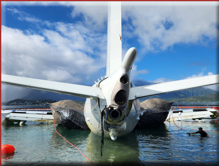
Tail view of P-8A after being rotated to the proper position for removal. After being floated via roller bags this orientation was achieved by tightening and slacking mooring lines.
