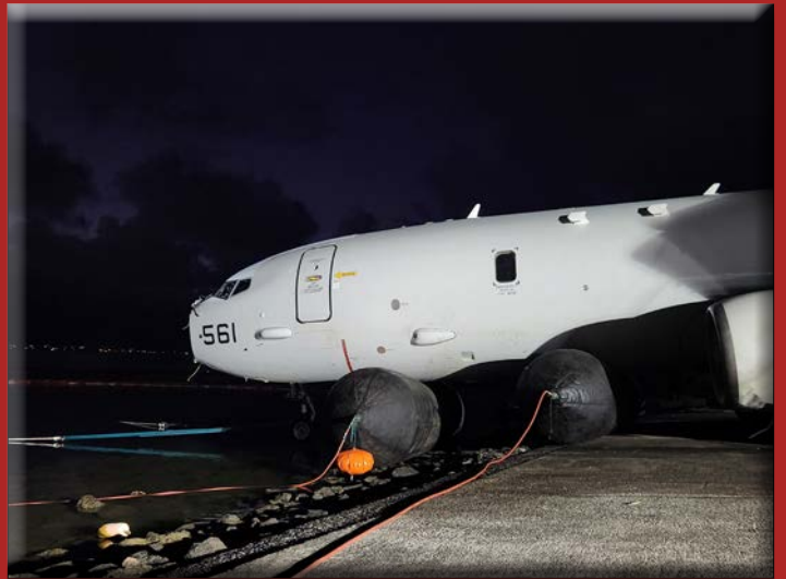
Placement of roller bags on the nose was particularly important to avoid damaging aircraft further due to the slope at the end of the runoff.
