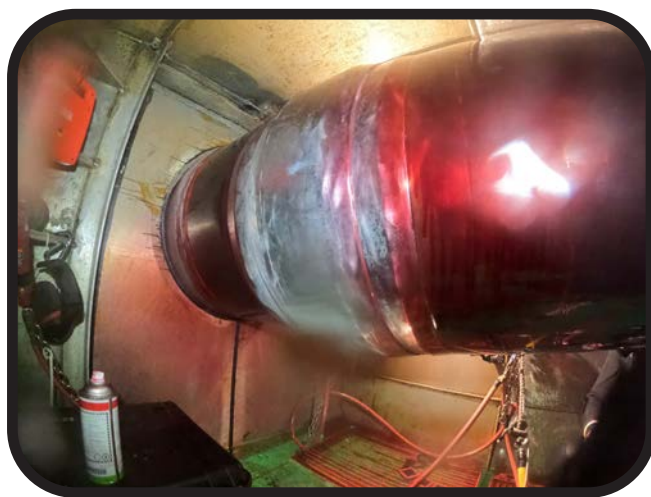
NDT in process on the propulsion shaft, this portion is located under the fairwater.
