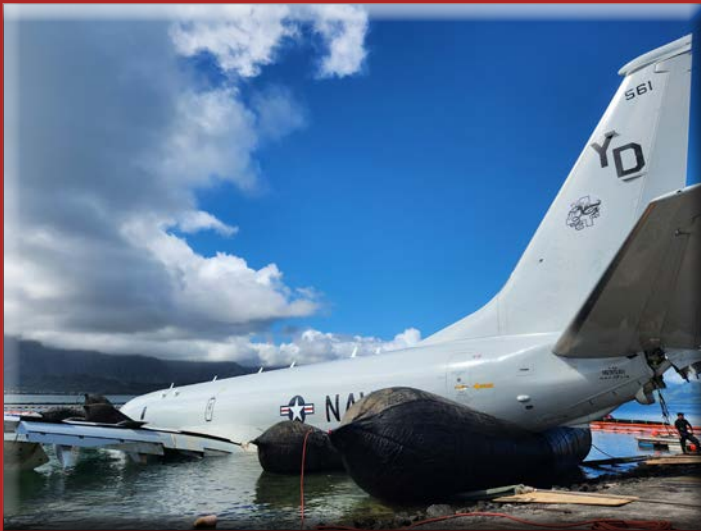
First stages of removing aircraft from the water utilizing roller bags and linear pullers.
