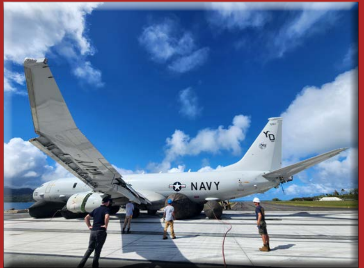
Roller bags strategically placed to continue moving aircraft to a safe location on the runway.
