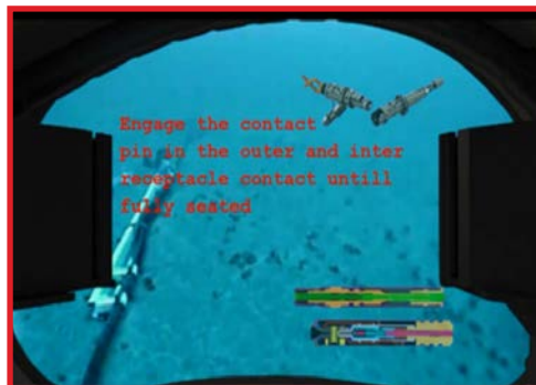
Diver's view while using the DAVD prototype on a dive mission (sector sonar image, Augmented Reality (AR) overlay image). Data and photos by Mr. Dennis Gallagher, NSWPCPD.
