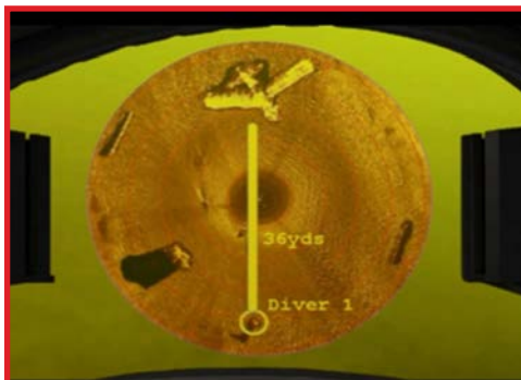
Diver's view while using the DAVD prototype on a dive mission (sector sonar image, Augmented Reality (AR) overlay image). Data and photos by Mr. Dennis Gallagher, NSWPCPD.
