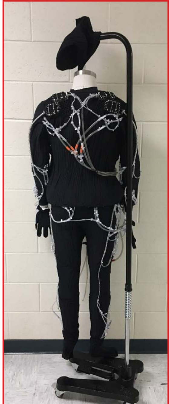
Second generation calorimetry suit. Data and photos from Dr. John Florian at NEDU.
