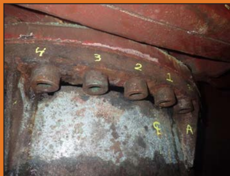
MER2 MCP Sea Chest Pipe to Flange Deterioration.
