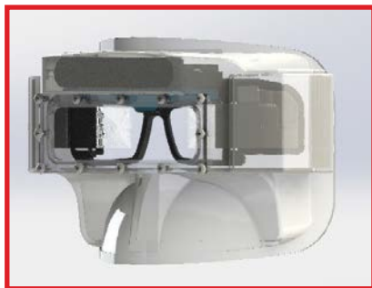
DAVD FFM Version Design Identical optics to the Kirby Morgan 37/97 design are used in the DAVD MK20 FFM version, with a custom faceplate designed to house them.
