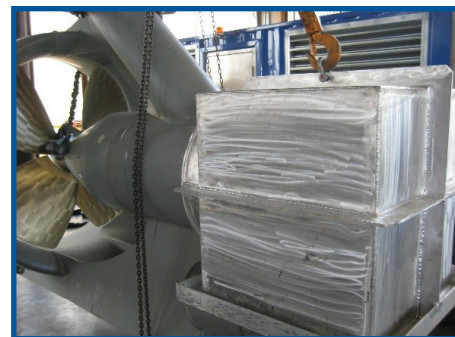
Open Bottom Cofferdam Installed in Place of End Cover (image from testing)
