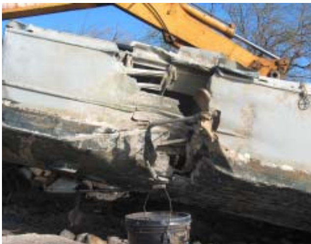
A view of the damage to the starboard aft engine room during the initial grounding.
