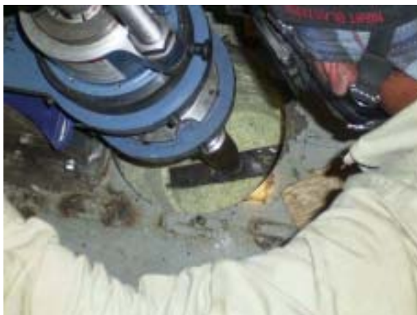
Creating second of two hull cuts.
