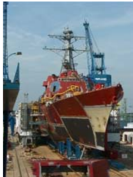
Land Level Ship Construction.
