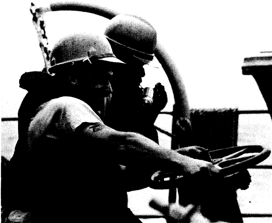
A boatswain's mate on the forecastle releases the brake on the anchor chain as the ship anchors for the night.
