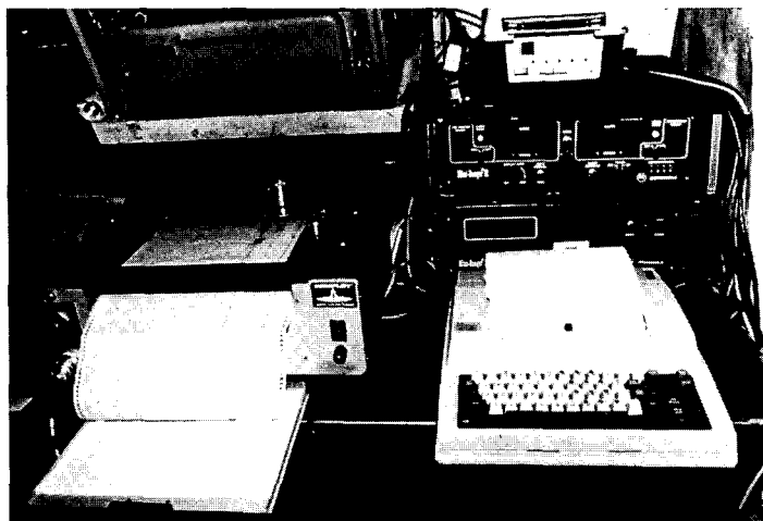
System components. Left — track plotter. Right (top to bottom) — data cassette recorder, range console, computer and terminal.
