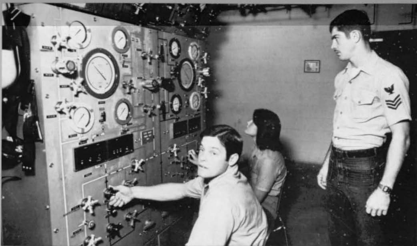
Above: Practical training at the hyperbaric chamber console. Students are thoroughly indoctrinated in all support equipment and the use of air and helium/oxygen decompression tables. Below: The "salvage hulk," used for practical salvage training.
