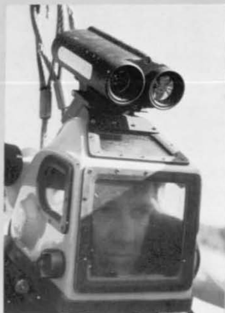
DHMTS was used to inspect damage 100 feet inside a 12-foot-by-12-foot culvert at a depth of 78 feet.
