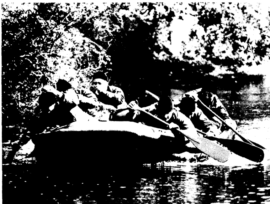
MARS, a versatile craft developed for Marine Corps reconnaissance and swimmer missions, can be locked-out of a submarine, helo-cast, or air-delivered to operational sites.
