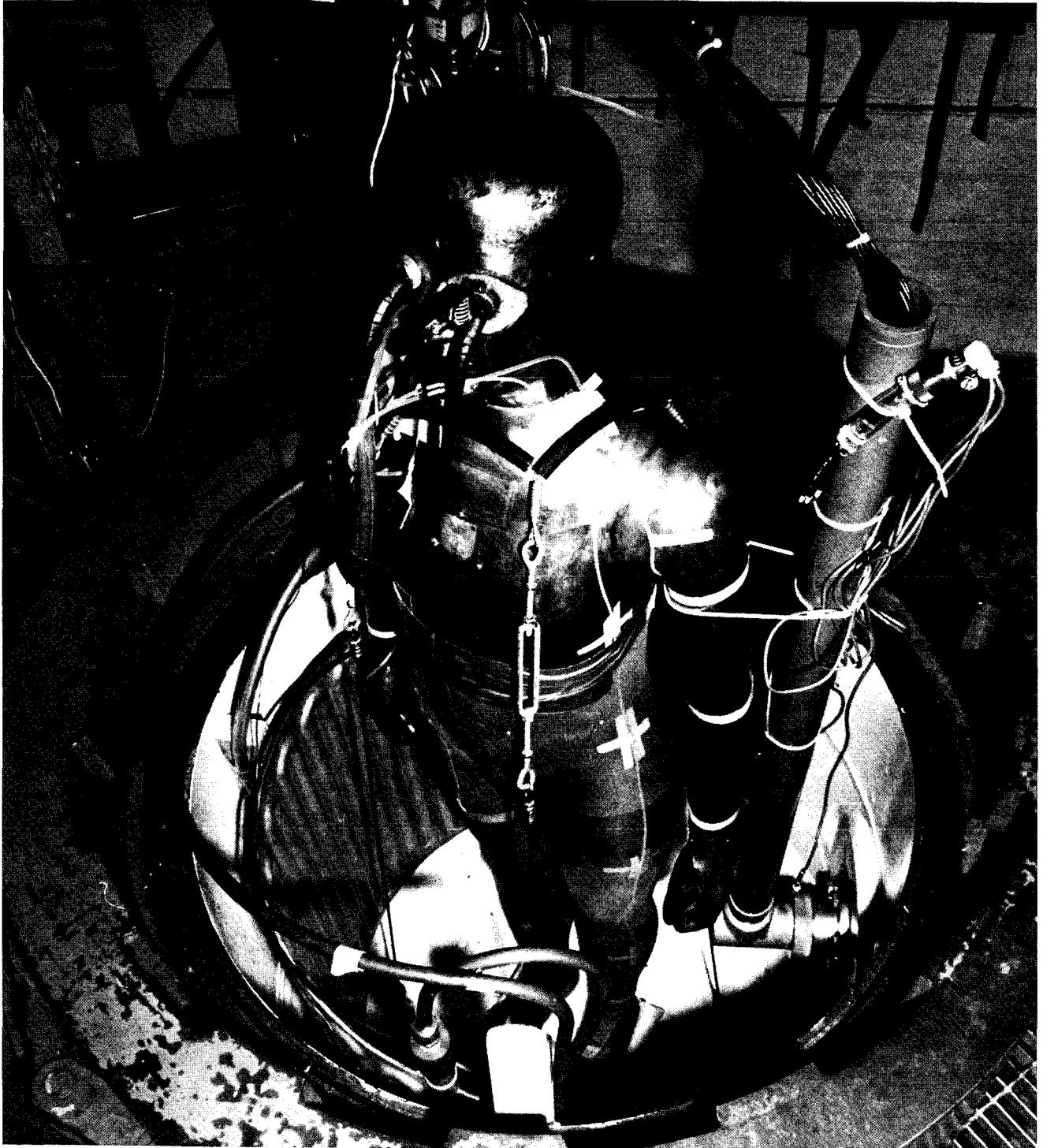
Above: ARIEM's copper manikin in hyperbaric test chamber. Right: Manikin is dressed in dry suit for NCSC diver thermal protection tests.
