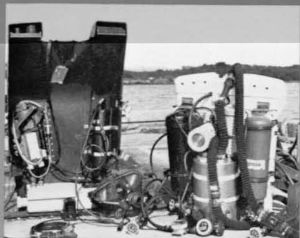
Mk 10 UBA with Mod 5 backpack. Backpack contains: UHF Radio (left); UDC (right); AN/PQC-4, with push-to-talk switch modification (bottom). Mk II Mask (in front of AN/PQC-4).
