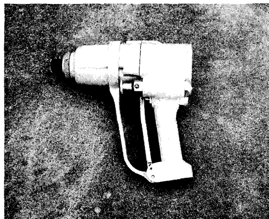
A 4 HP hydraulic impact wrench.
