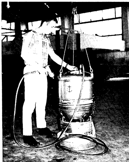
Submersible, cryogenic module for pneumatic tools; rated at 20 cfm, 90 psi.
