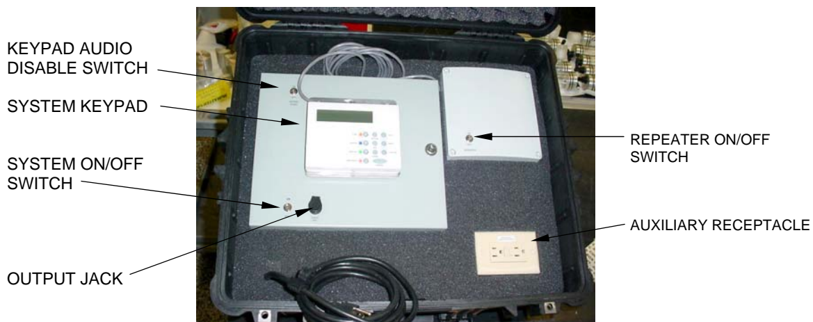
Figure 1. The Cofferdam Alarm Control Station
