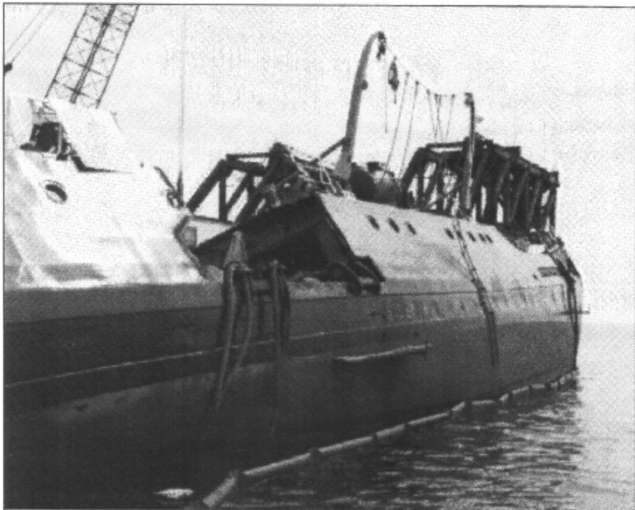
Figure 3-17. Hauling Lines Attached to Lift Pads Prior to Parbuckling the Wreck to Even Keel.
