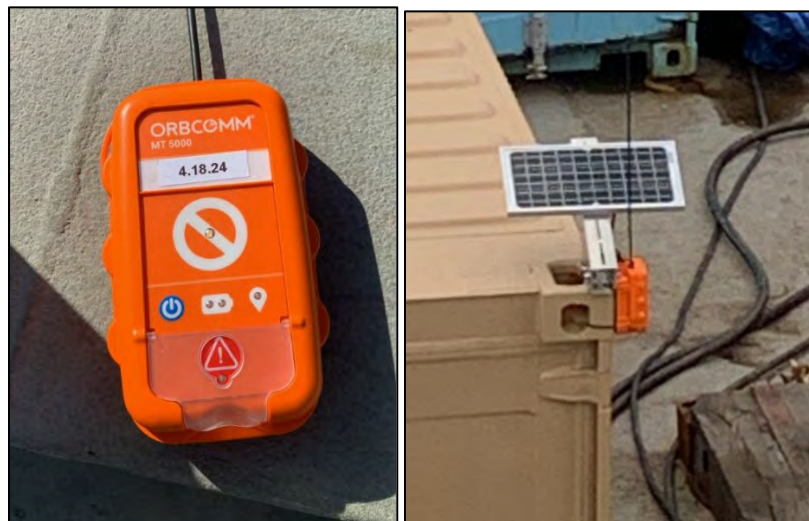
Figure 6-6 ORBCOMM AIS transmitter (closeup) and an AIS transmitter mounted along with a 25W solar panel providing a standalone solution for non-powered vessels.
