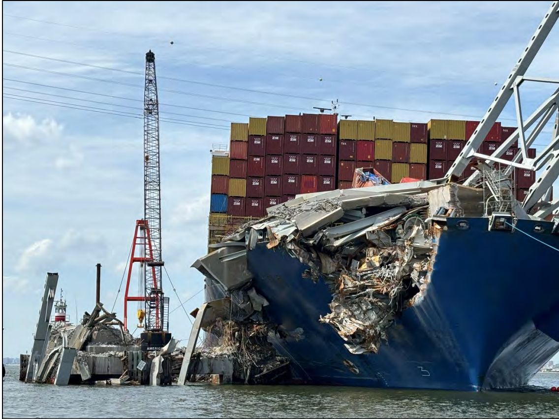
Figure 7-19 DALI's starboard bow after the large section of span 17 was removed.
