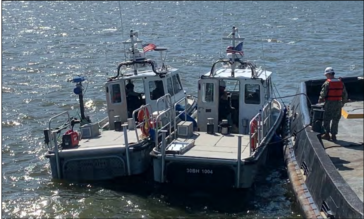
Figure 5-4 ESSM Boom Handling boats tied alongside a Donjon tug. Note the outboard vessel has CODA Octopus system boom mounted midships on its port side.
