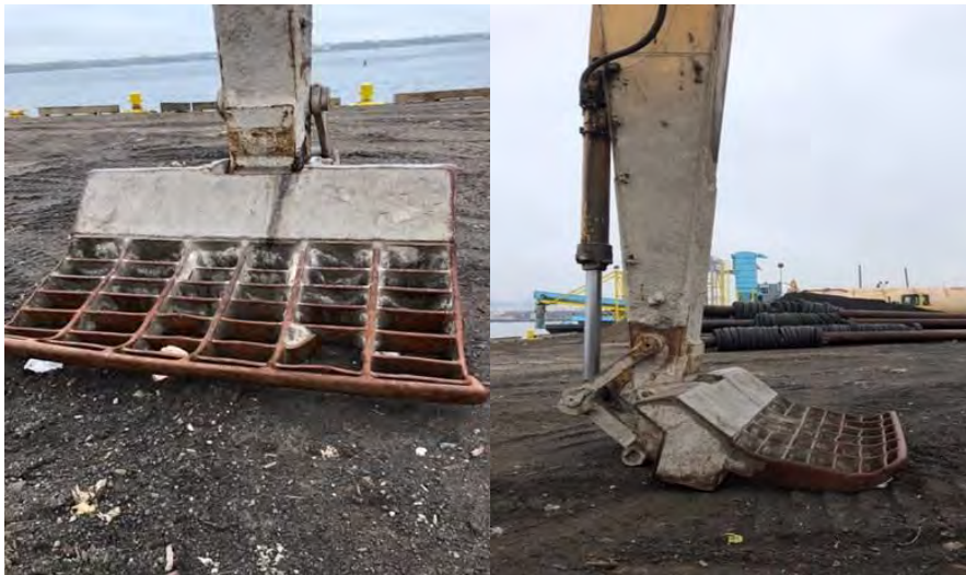
Figure 2 Grapple on Excavator assist mixing mud/concrete Specs: 7'4" Wide X 6'6" long with 12" spaces.
