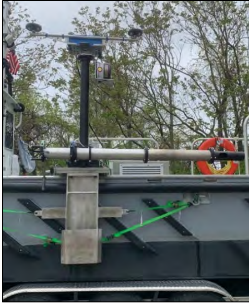
Figure 7-3 CODA Octopus sonar system mounted on an ESSM boat. Note GPS receivers on top, and the CODA Sonar, swung aft, out of the water for transiting.
