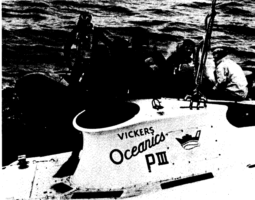
First crewman from PISCES III is assisted into a GEMINI rubber boat. Note that additional lines from CABOT have been attached to main lift point of PISCES.
