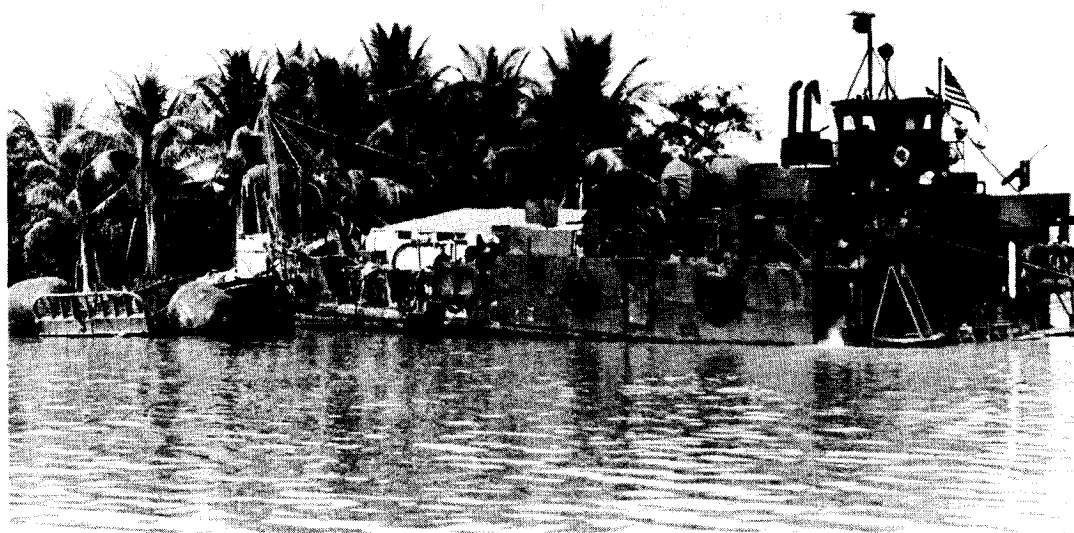
YLLC-1 lifts wrecked LCM-6 up onto the shore of the Song Vam Co Dong near Ben Keo during one of its many SALVOPS in 1970. Note 8-ton salvage balloons to keep bow afloat.
