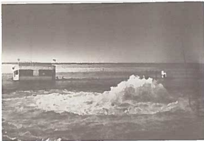
PHOTOGRAPH 30. Flapper valves continue to vent as starboard side rises from the bottom (Phase Three).
