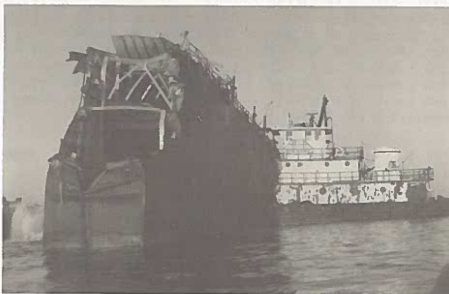
PHOTOGRAPH 26. Damage to machinery throughway and Tank 20 (below safety deck) on aft section wing wall.
