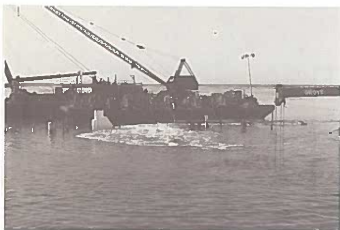
PHOTOGRAPH 10. Air leakage from damaged plate on inboard wing wall.
