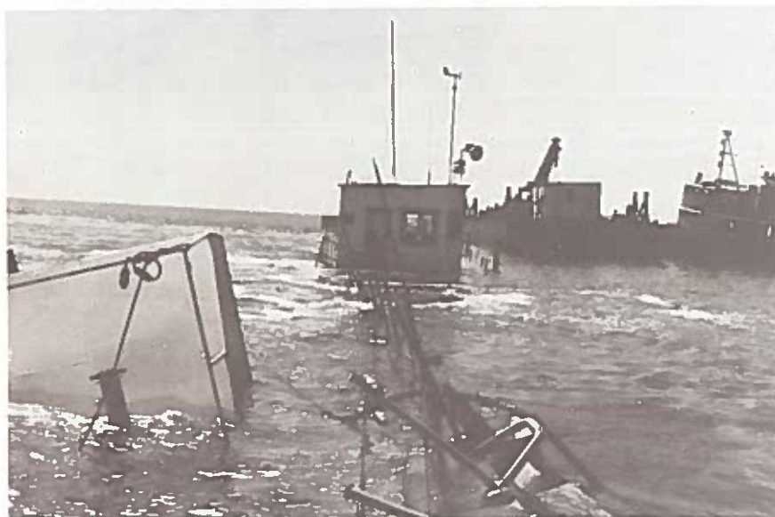
PHOTOGRAPH 21. Aft section now completely afloat. Tugs pulling section from beneath forward section overhang.
