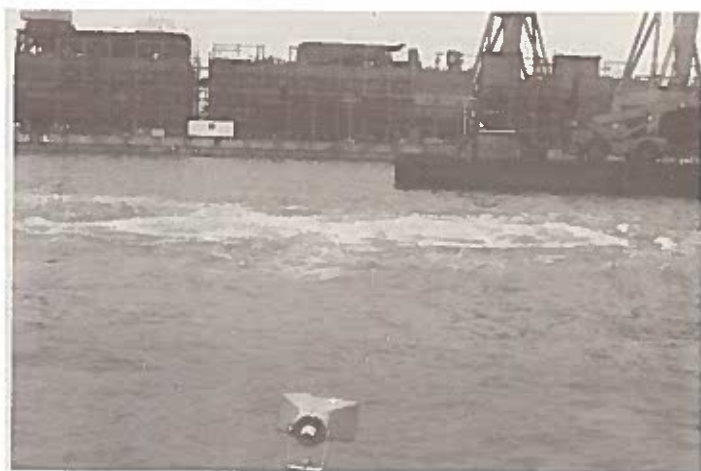
PHOTOGRAPH 9. Air leakage from propeller pits.
