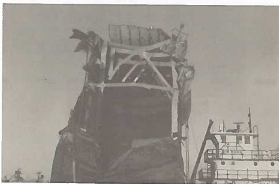
PHOTOGRAPH 27. Closer view shows extensive damage which precluded patching and pumping of Tank 20.
