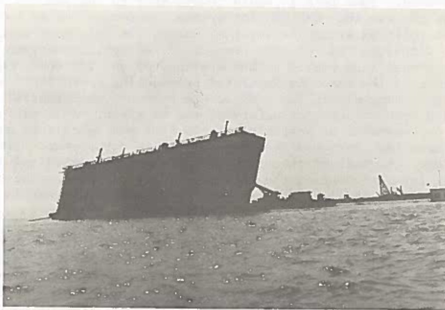
PHOTOGRAPH 13. Starboard side of aft section successfully rotated using four-inch sub pumps supplemented with compressed air.
