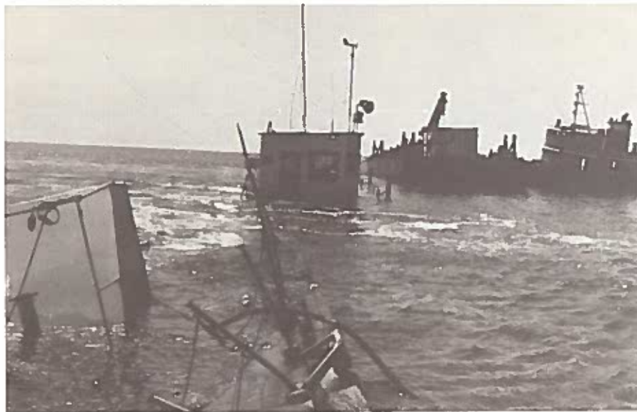
PHOTOGRAPH 20. Breakout of forward port corner of aft section. A trim of 20 feet was being experienced at this time.
