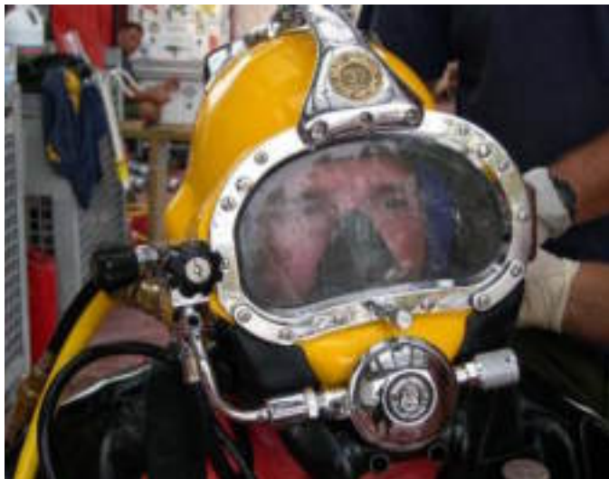
Figure 5-1. Kirby Morgan 37 dive helmet used by MDSU TWO divers in contaminated water operations.
