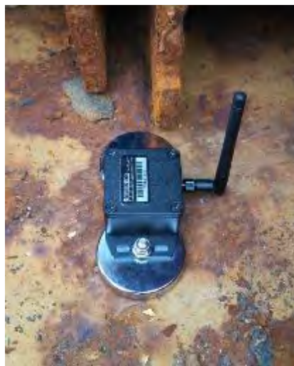
Figure 3.2 – Accelerometer installed at the fore section of the MV TREASURE pontoon deck.
