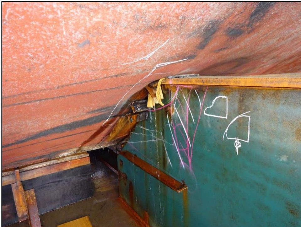
Figure 5-16. Port side damage due to interference with grillage, also found on starboard side
