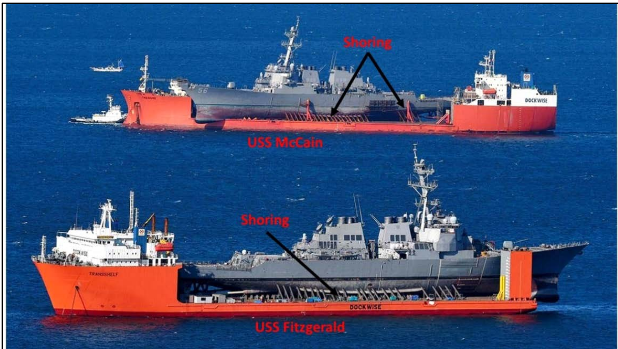
Figure 4-8. USS John S. McCain and USS Fitzgerald in Tokyo Harbor. With two ships in the same image, a comparison of the number and arrangement of shore stays is possible.
