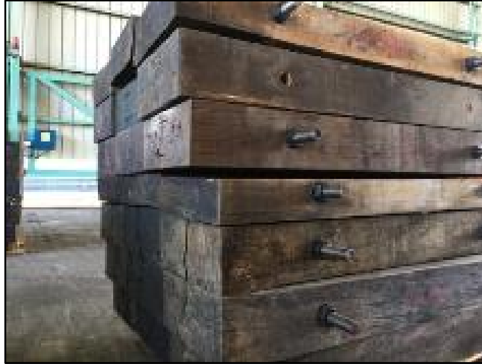
Figure 4-14. Typical hardwood blocks before machining flat.
