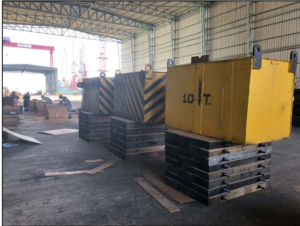
Figure 4-16. Preloaded block with plywood between layers
