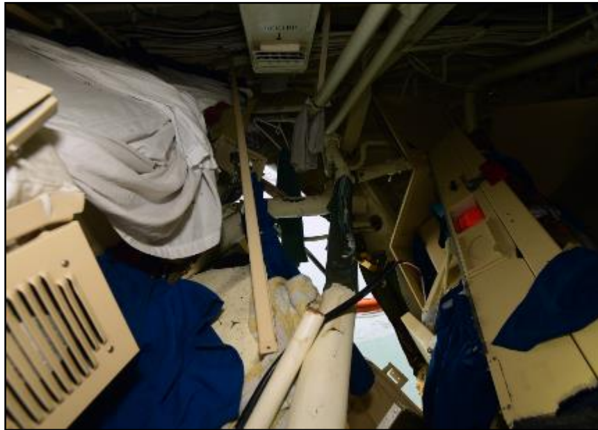
Figure 3-1. Berthing 3 damage similar to that seen underwater in Berthing 5.
