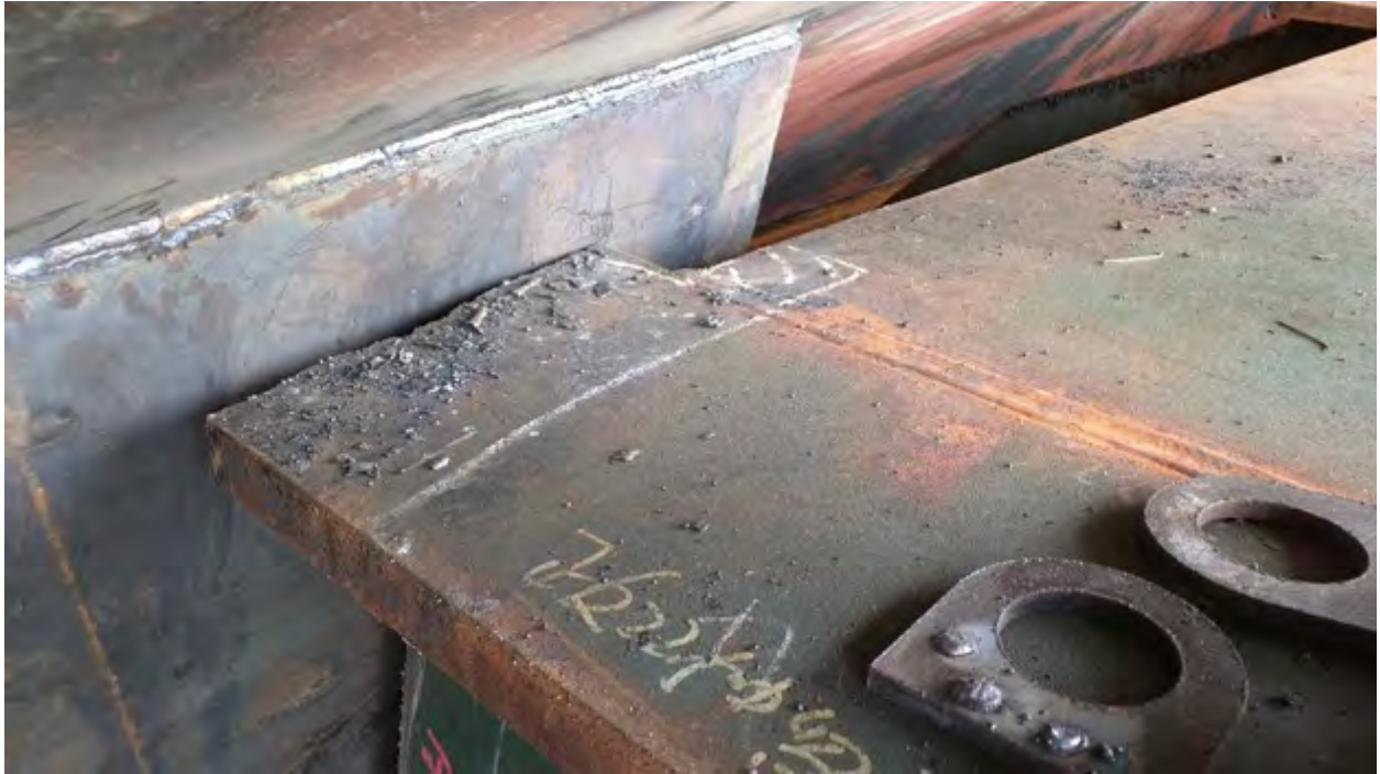
Fig 11. Grillage beam in contact with the box patch on the cargo hull's port side.
