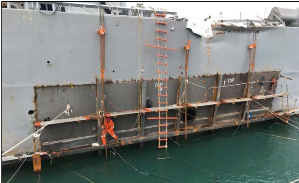
Figure 3-7. John S McCain's patch during installation.
