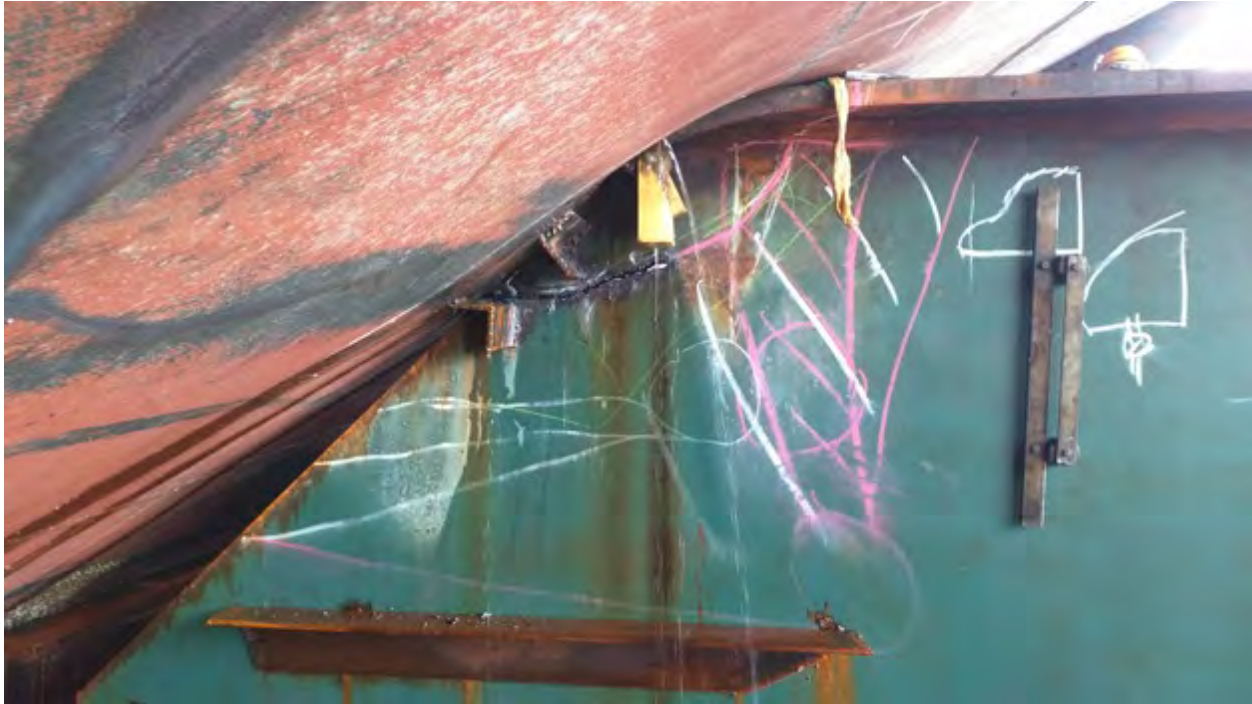
Fig 7. Cargo port side hull puncture resulting from contact with grillage at HTV frame 88.
