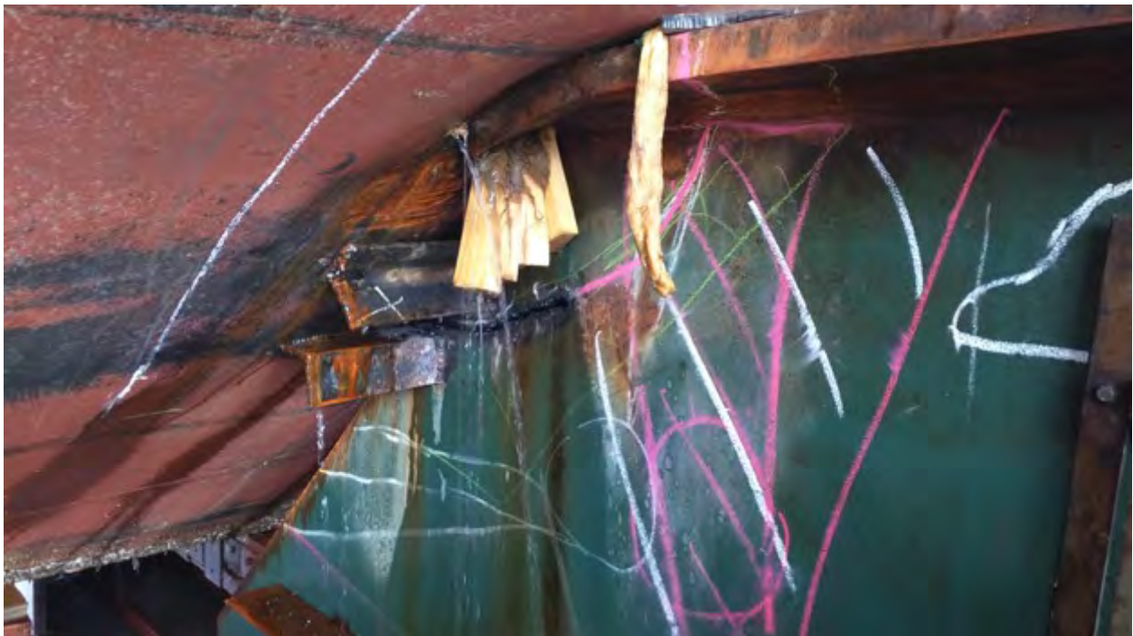
Fig 6. Cargo port side hull puncture resulting from contact with grillage at HTV frame 88.
