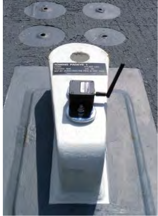
Figure 3.4 – Accelerometer installed on the bow of the USS JOHN S MCCAIN
