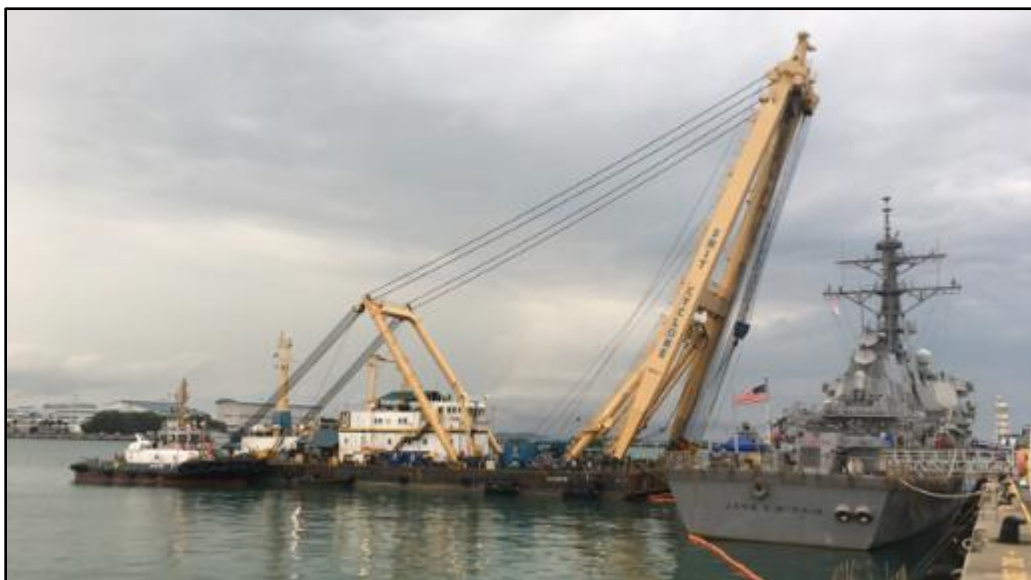
Figure 3-6. SMIT Cyclone with shear leg crane
