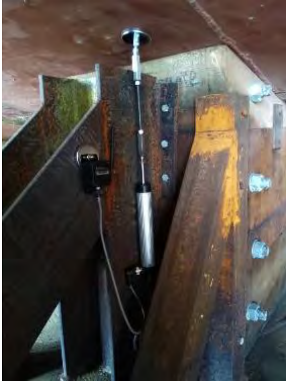
Figure 3.3 – Displacement sensor installed on the hull of the USS JOHN S MCCAIN
