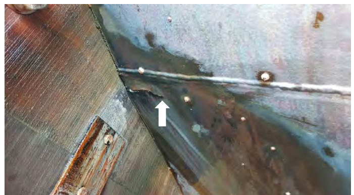
Fig. 6 – Linear indication under the docking block
