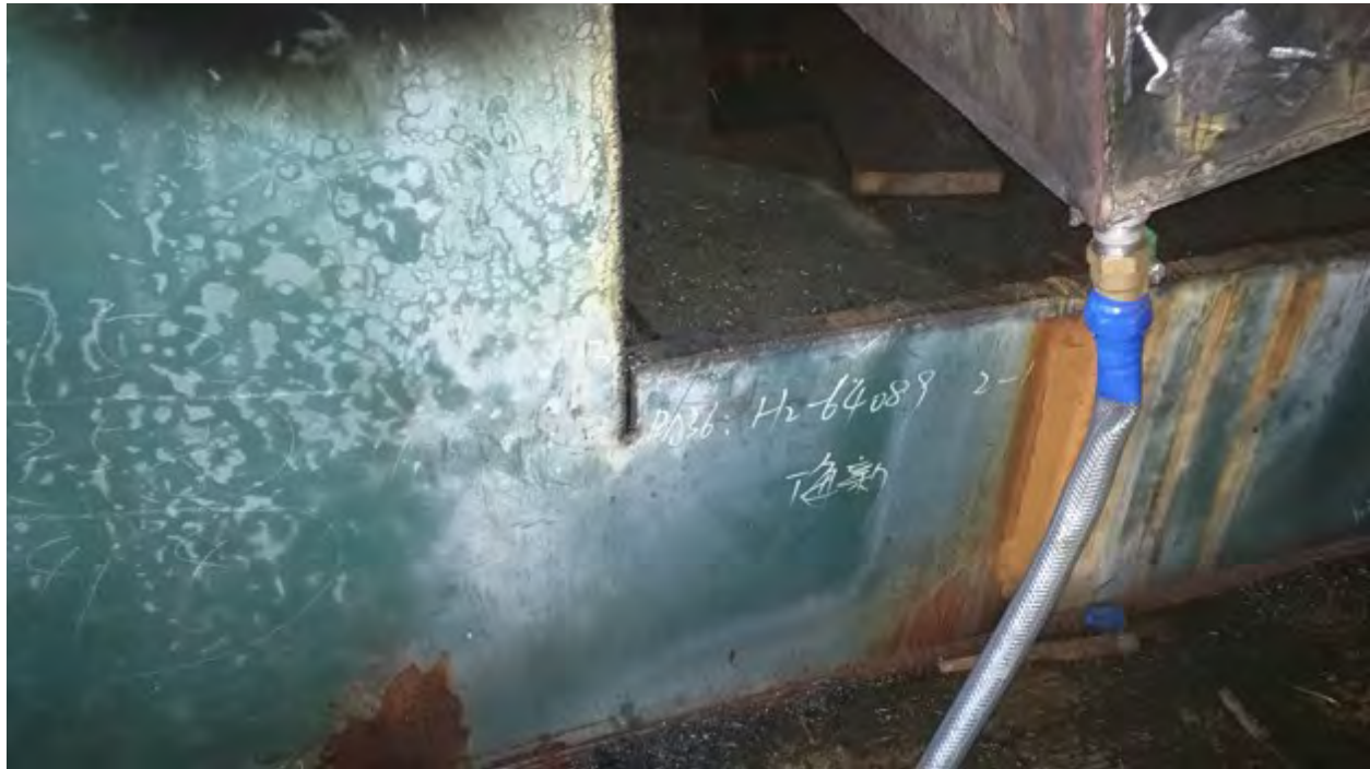
Fig 10. Overcut of the beam under the cargo starboard side box patch.
