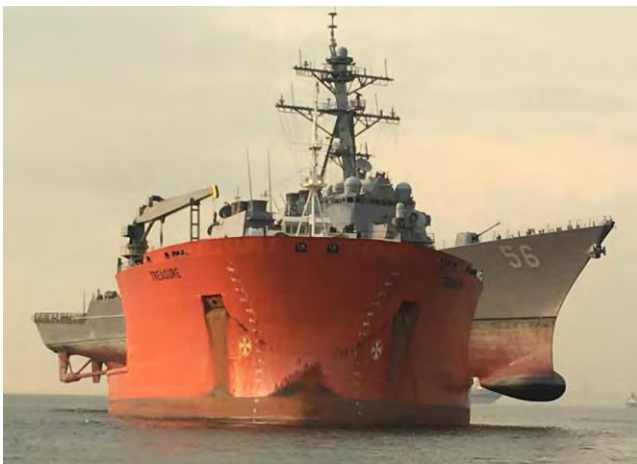
Fig 3 – Bow view of the cantilevered USS John S. McCain loaded aboard the MV Treasure
