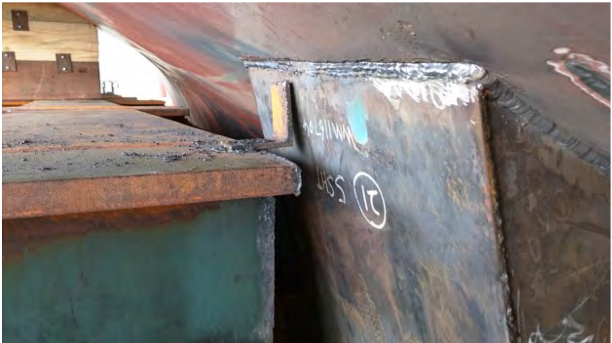
Fig 12. Grillage beam in contact with the box patch on the cargo hull's starboard side.
