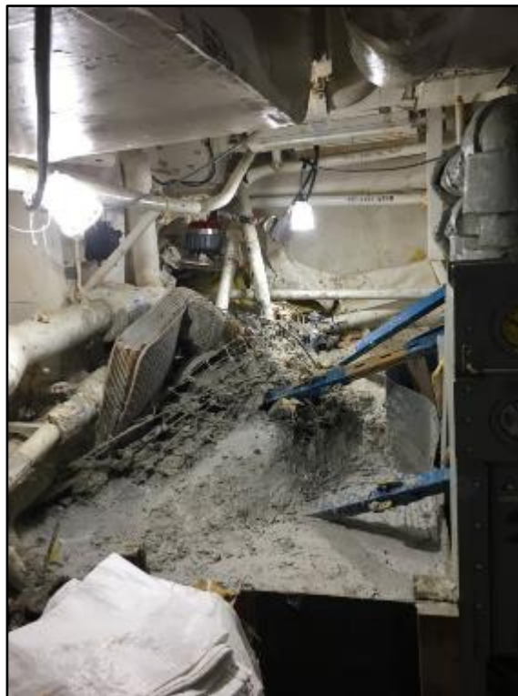
Figure 2-3. Auxiliary Machinery Room 1 salvage patch after application of cement
