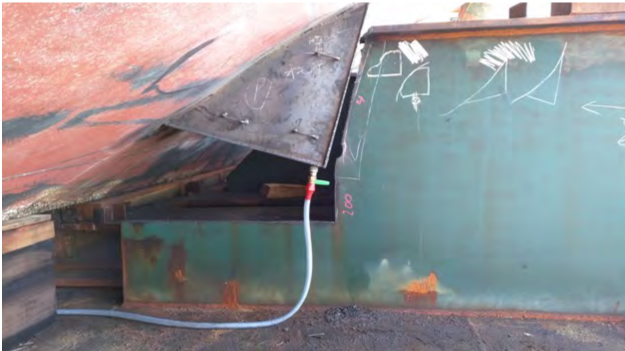
Fig 9. Cargo port side hull puncture box patch.
