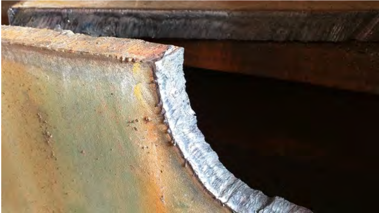
Fig 15. Surface finishing on the rounded grillage cut angle on the cargo hull's port side.
