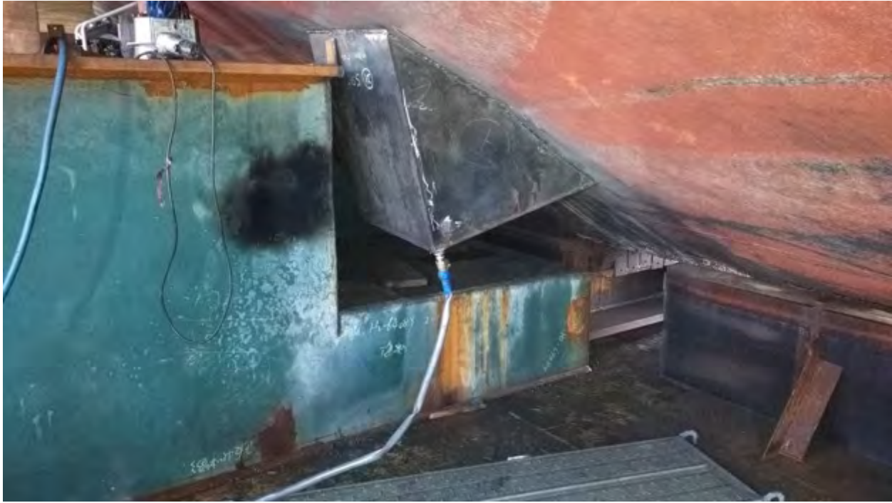
Fig 8. Cargo starboard side hull puncture box patch.
