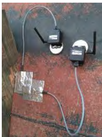
Figure 3.7 – Strain gauges installed on the hull of the USS FITZGERALD.
