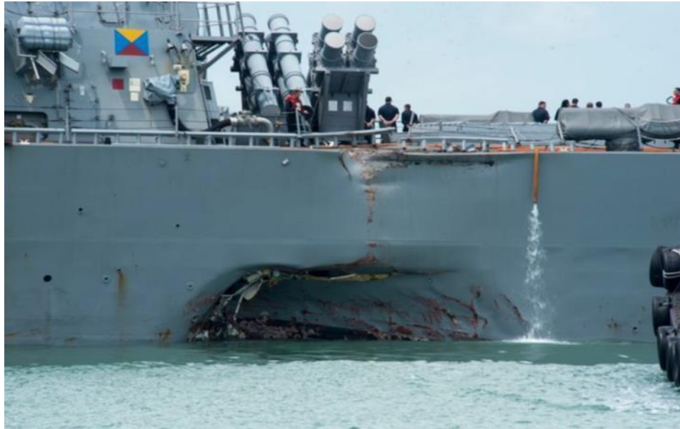
Figure 1-4. Photograph of the damage to the port side of John S McCain extending from frame 308 to frame 342.
