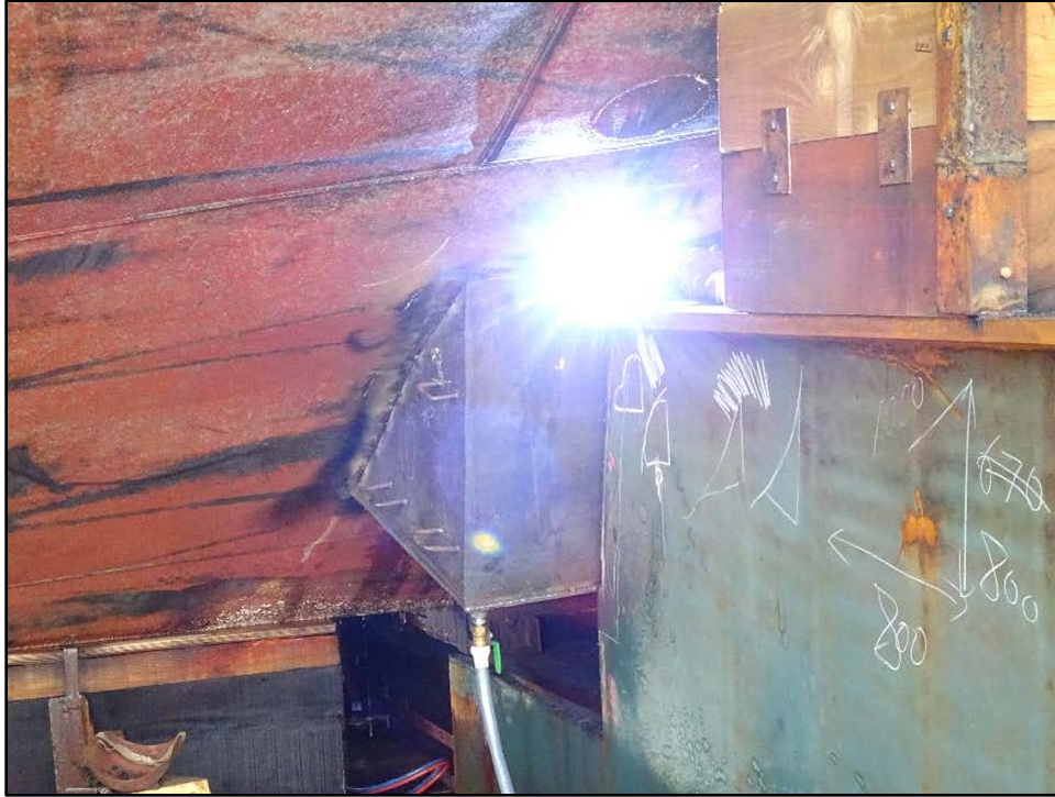
Figure 5-17. Portside box patch being welded to USS Fitzgerald hull
