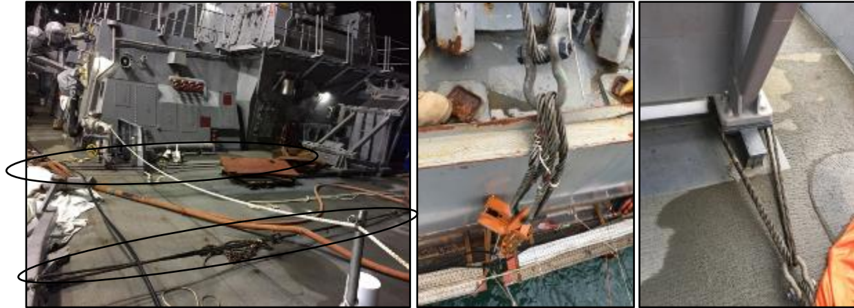
Figure 3-8. Rigging patch to hardpoints on USS John S McCain's deck.
