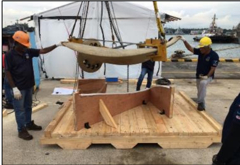
Figure 3-11. The first blade is lowered onto newly constructed blade box. Boxes were built to keep the blades safe during their shipment back to Yokosuka.
