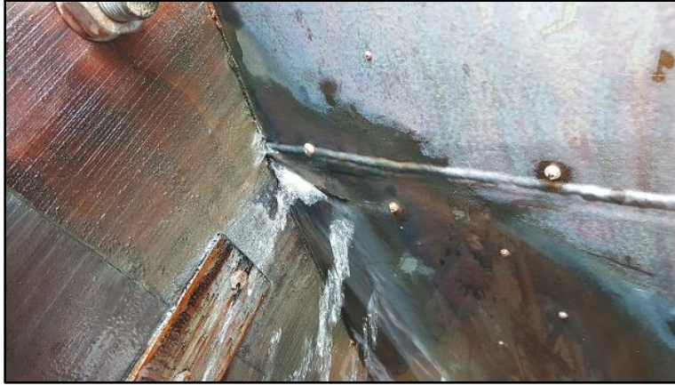
Figure 4-10. Crack at frame 268, port side
