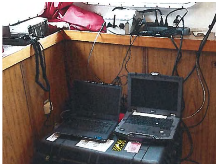
Figure 3.6 – Control station setup on the bridge of the MV TRANSSHelf for the strain sensor system and smart TOW deployed for the USS FITZGERALD heavy lift transport.
