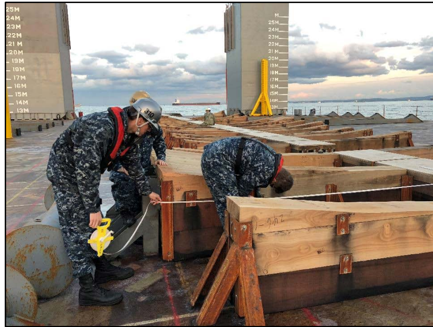
Figure 5-11. Heavy Lift Team Measuring and Repairing Onload Blocking
