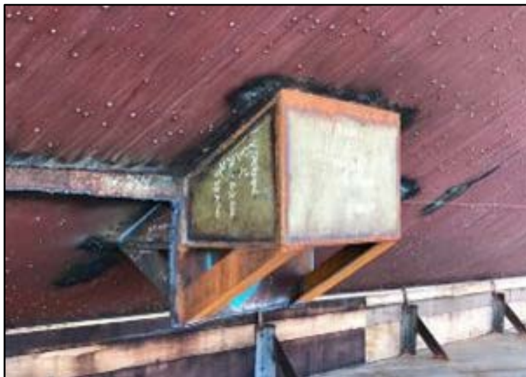
Figure 4-22. Concrete filled box patch around Fathometer Trunk
