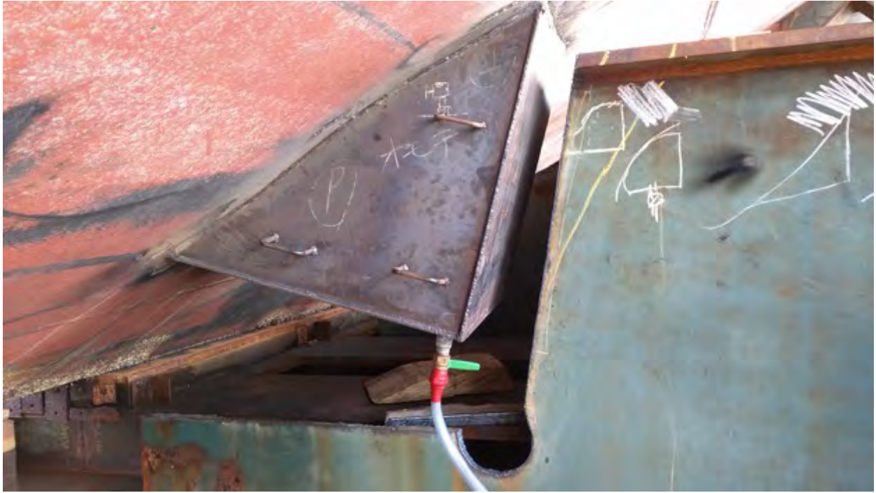
Fig 13. Revised grillage cut on the cargo hull's port side.
