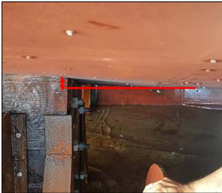
Figure 4-11. Hull deflection of approximately 15 mm at block interface
