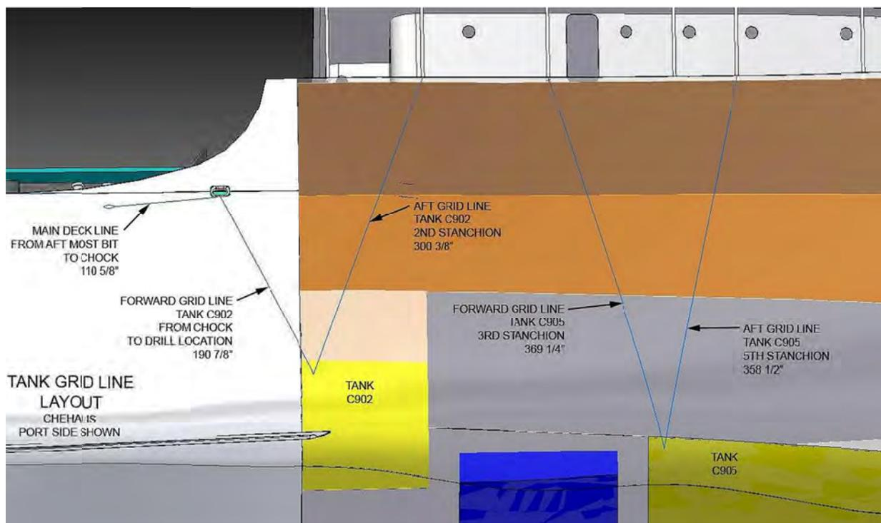
Figure 5-4. Ex-USS *Chehalis* Tank Grid Line Layout
