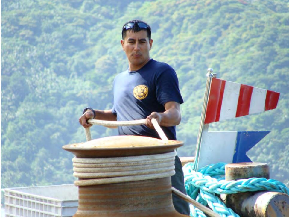
Figure 17. Tending the Divers Stage Line on an ESSM Capstan
