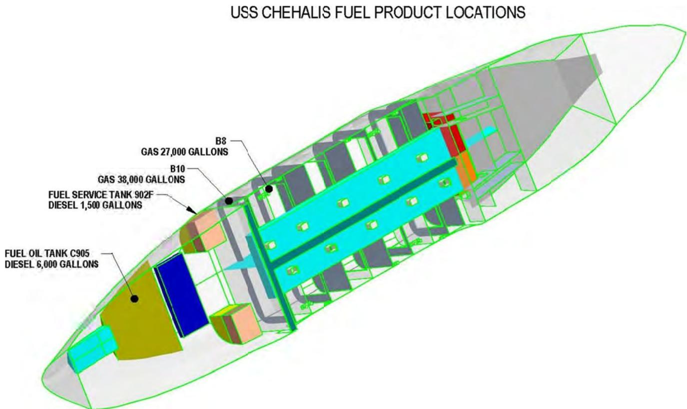
Figure 1. Ex-USS *Chehalis* Showing Tanks with Pumpable Petroleum Products
