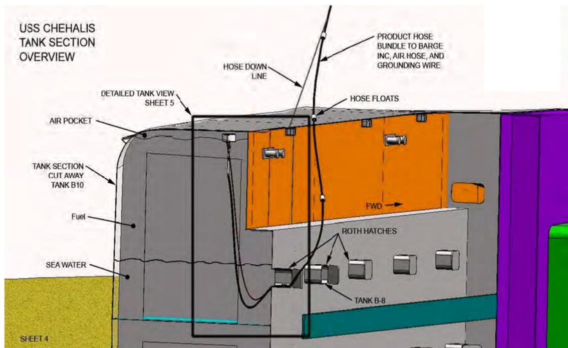
Figure 5-10. Ex-USS *Chehalis* Tank Pumping Overview
