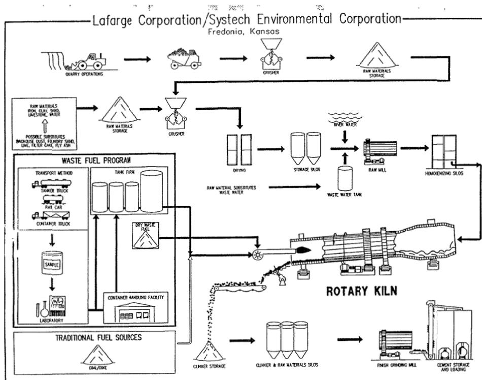
Figure 6-6. Systech Environmental Waste Fuel Processing
