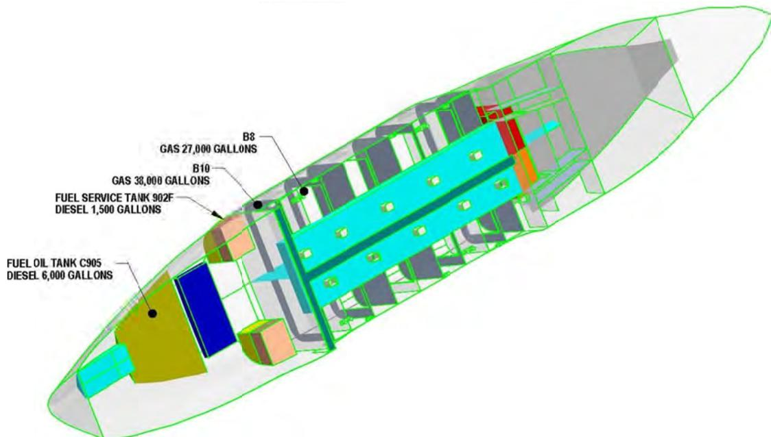
Figure 1-1. Ex-USS *Chehalis* Showing Tank Locations and Expected Fuel Volumes
