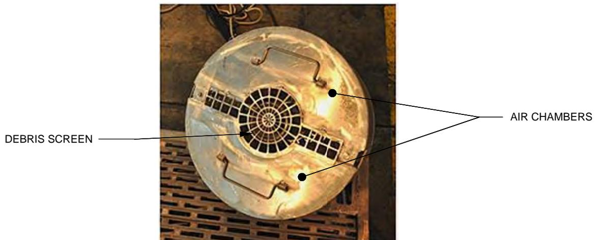
Figure 5-12. Suction Head (Top View)
