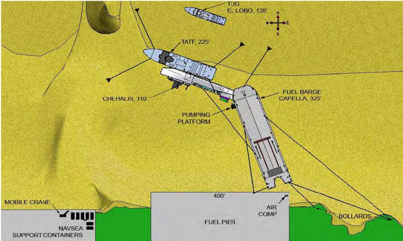
Figure 2. Notional Ex-USS *Chehalis* Pumping Platform Configuration
