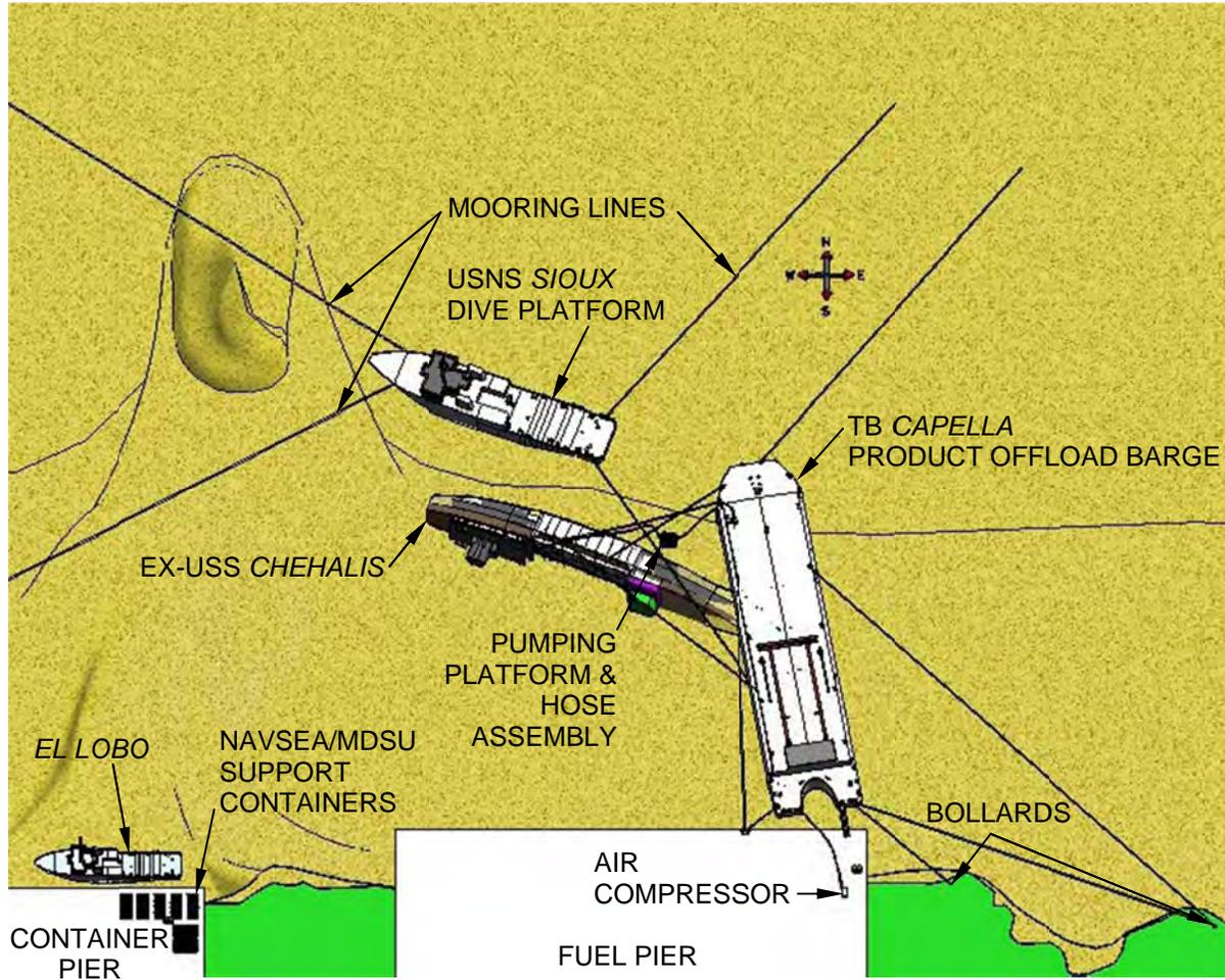
Figure 5-1. Ex-USS *Chehalis*' Mooring Plan
