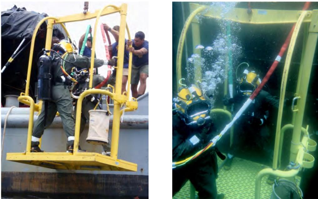
Figure 5-23. Left: Lowering the Divers' Stage into the Water, Right: Divers Shackling in the Stage to the Down Line Leading to Ex-USS *Chehalis*
