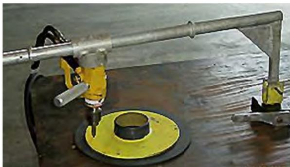
Figure 5-6. “Bubba Bar” and Drill in Position over Flange
