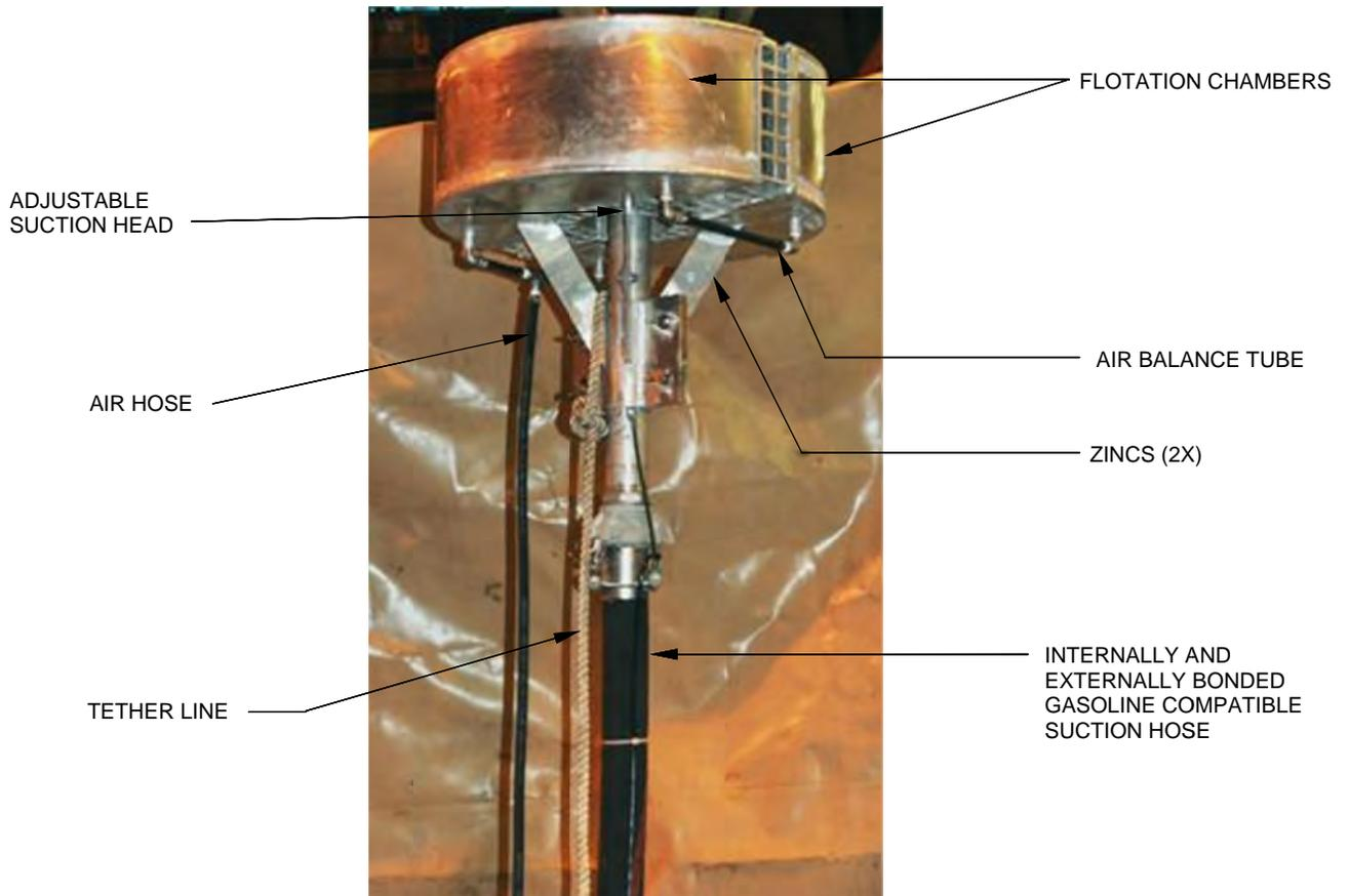
Figure 5-11. Suction Head (Side View)
