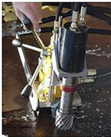
Figure 5-13. Hydraulic Boring Machine
