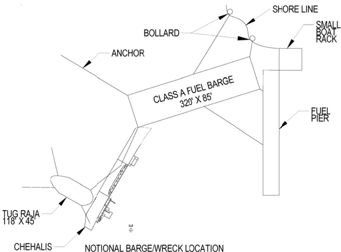
Figure 1. Ex-USS *Chehalis* Notional Barge/Wreck Concept
