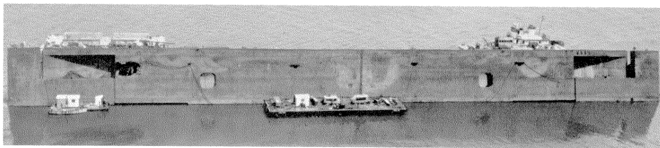
MOST SERIOUSLY DAMAGED WINGWALL , with oval-shaped hole (left), is shown at Stage XI. Salvage plan called for this wall to be placed offshore during the parabuckling operation so that the hole would be above water while the drydock was being rolled.
