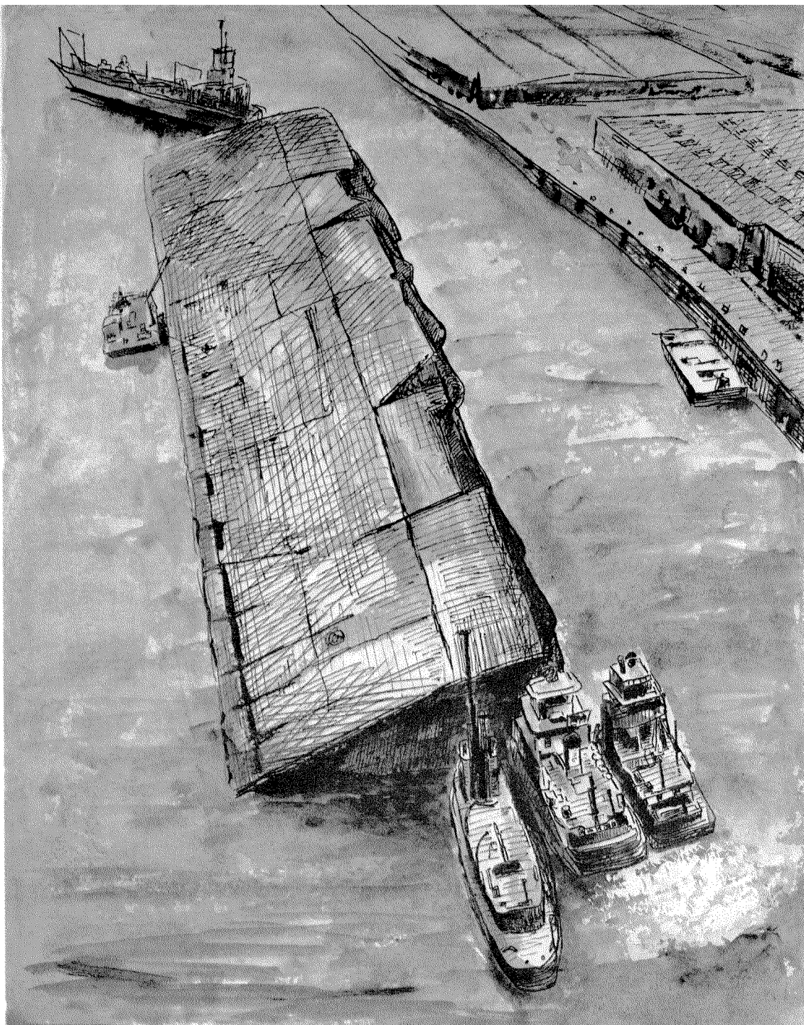
RETURNING DRYDOCK to salvage site on west bank required the services of three Navy ships—salvage ship CURB and lift ships SALVAGER and WINDLASS—and nine tugs. Plan called for AFDM-2 to swing pendulum fashion on four lines fastened to anchors dropped in mid-river as ships pulled and pushed her across. Anchors slipped, however, and move was completed under alternative plan.
