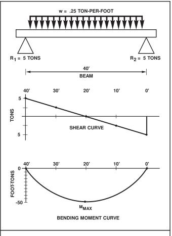
Figure 5-6. Bending Moment and Shear Curves for Example 5-3.
