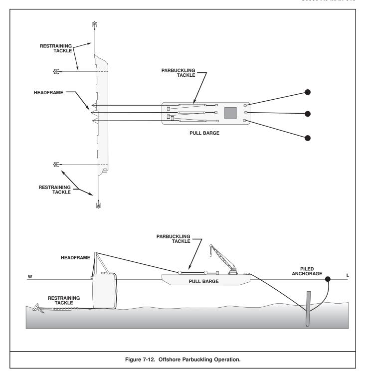
**7-6.4** Offshore Operations. A ship that is capsized and sunk a considerable distance offshore presents several problems. The problems are rarely insurmountable, but can add greatly to the cost and time of the operations. Some of the most common offshore or exposed-location righting difficulties are:
