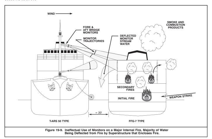
Figure 19-9 shows how a large percentage of water stream projected by monitors is wasted against steel superstructures and impenetrable barriers on a smaller combatant.
