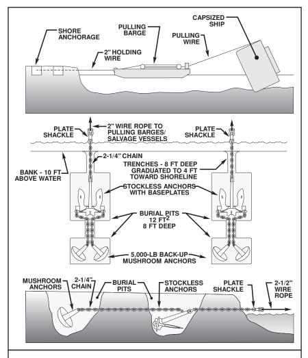
Figure 7-23. Anchorage for Small Righting Job.
