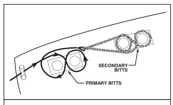
Figure 9-2. Wire Rope Backed Up by Chain on Secondary Bitts.
