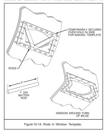
template. The window, shown in Figure 10-13, is large enough to enclose the hole and, when possible, to land on the shell plating clear of the major damage. The window is constructed of light wood with the periphery drilled at regular intervals to accept adjustable dowels
