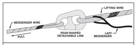
Figure 12-26. Wire Messengers Connected with Detachable Link.
