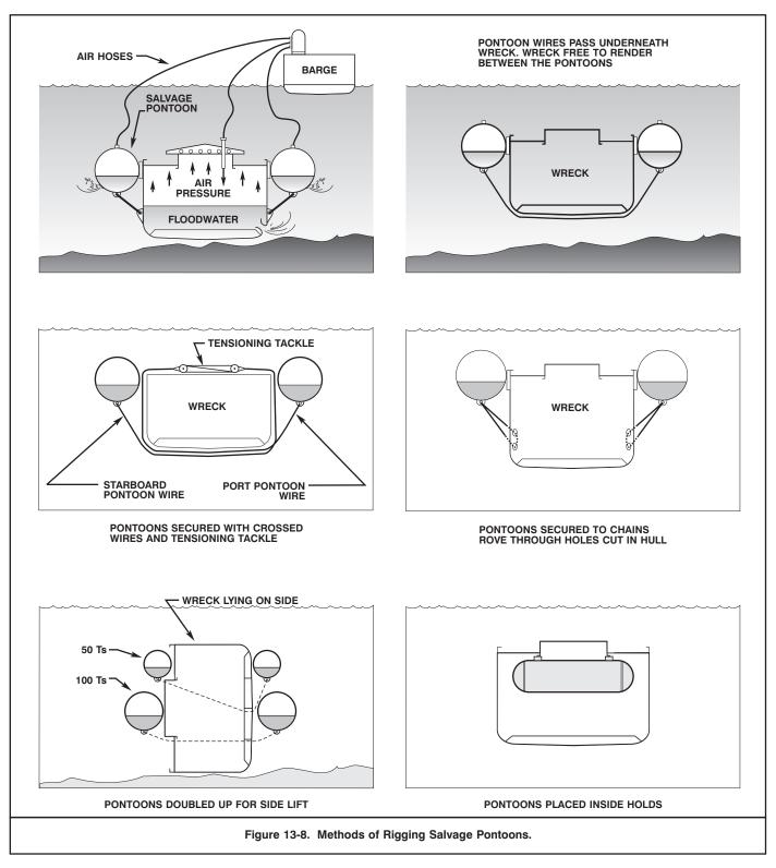
For strength and lift balance reasons, pontoons are best rigged in pairs. Each pair should be connected by chains or wire ropes passing, under, through, or attached to the sunken ship. Figure 13-8 shows some typical ways of rigging pontoons to sunken ships.
