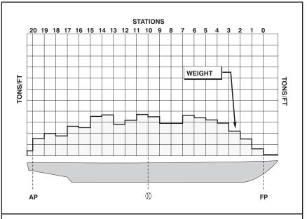
Figure 14-2. Weight Curve for Frigate.
