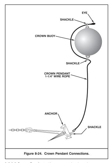
**8-5.2.5 <u>Crown Pendant</u>**. The crown pendant is used to recover or reset the ground leg anchor.
