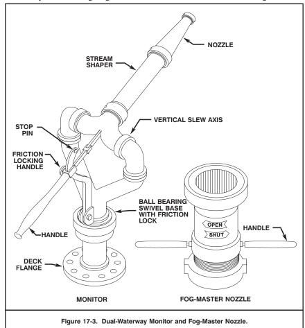
**17-3.2.1** <u>Monitors</u>. Typically, naval and commercial salvage tugs have fixed fire monitors. Monitors allow the salvage tug to project large amounts of water or foam on the exterior of the casualty. The
