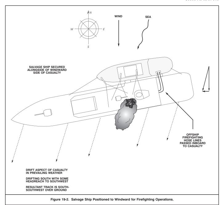
Figure 19-2 shows an assisting vessel moored alongside the windward side of a drifting small combatant, using both monitors and offship fire hoses for fire control and extinguishing. The decision as to whether the assisting vessel should make up to the casualty, as shown, or stand off depends on several factors:
