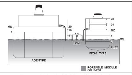
Figure 20-1. Relationship of Work Boat to Casualty Vessels and Staging of Portable Pumps.
