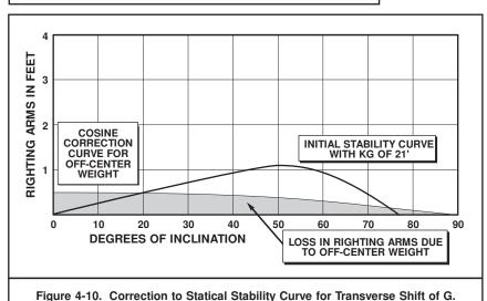
**4-2.9.3** Off-Center Weight Correction. When there is off-center weight and the center of gravity is no longer on the centerline, a list results and there is deterioration in the stability characteristics,
