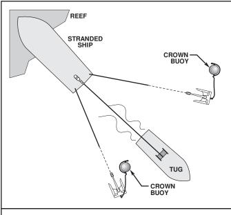
Figure 9-4. Pulling with Beach Gear and Tug Combination.
