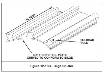
Figure 12-18A shows a bilge bolster with a series of roughly shaped 12×12-inch timbers. This type of bolster is made from plate of between ½-inch and 1-inch thickness, rolled to a radius that varies between 24 and 36 inches, depending upon the chine configuration of the vessel being lifted. Figure 12-18B shows a field-fabricated bilge
