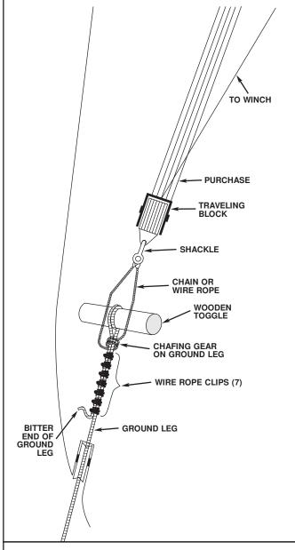
Figure 8-27. Toggle Bar Used as Stopper on Ground Leg.
