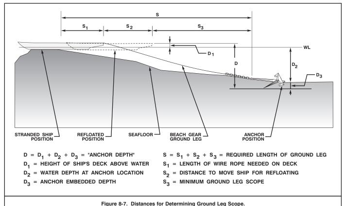
**8-3.4.4 Ground Leg Catenary.** For an anchor to develop its maximum holding power, the shank of the anchor and the pull on the shank must be parallel to the seafloor when the maximum pulling force is applied. Even a slight angle will seriously reduce the anchor's holding power. A six-degree angle will reduce holding power by 15 percent, a twelve-degree angle by 38 percent, and a twenty-degree angle by 50 percent. Figure 8-8 shows the chain holding the anchor shank parallel to the seafloor.
