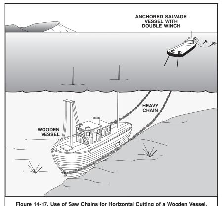
In conventional (vertical) chain cutting, salvage cranes exert lifting and tearing forces against their own buoyancy as in normal lifting operations. The cranes are usually designed to lift 400 to 1,000 tons on their main tackles. Total vertical component pulls of 300 to 400 tons for chain cutting do not materially affect the barge or require special anchorages.
