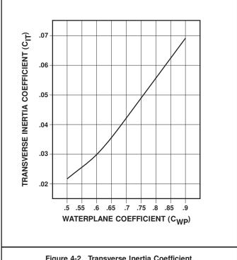
Figure 4-2. Transverse Inertia Coefficient.
