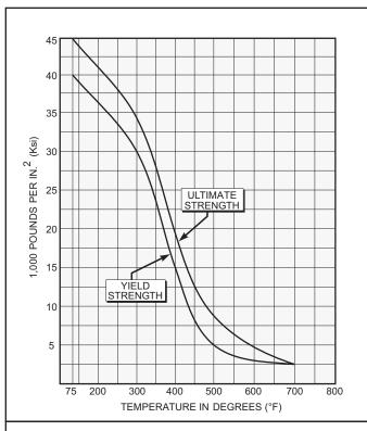
Figure 16-2. Temperature Effects on Aluminum (6061-T6).
