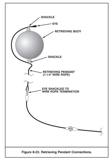
**8-5.2.4** Retrieving Pendant. The retrieving pendant is a length of wire rope longer than the water depth used to retrieve the ground leg. One end of the retrieving pendant is connected to the shoreward end of the ground leg wire rope; the other end is suspended from a buoy.
