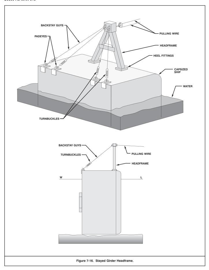
**7-8.2.2** Stayed Girder Design. In the stayed girder design (Figure 7-16), headframes are stayed back to hull connections on the sunken ship. This design is advantageous when there is a shortage of structural steel. Stayed girder designs require numerous wire backstays and more time-consuming and costly field rigging work than the braced girder design. It is difficult to achieve uniform stayback tension and to control quality because of the number of anchorages, padeyes, and field connections.
