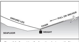
Figure 8-9. Ground Leg Configuration, Anchor on Up-Slope.
