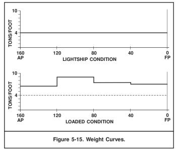
The following example develops the weight, buoyancy, load, shear, and bending moment curves for a rectangular barge.
