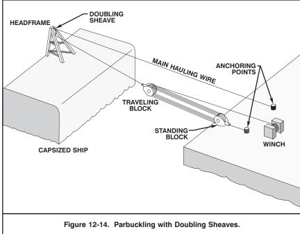
**12-7.2** <u>Utility of Doubling Sheave Systems</u>. Doubling sheave systems produce an increase in power that is useful where:
