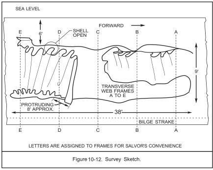
The survey does not produce an engineering specification for a salvage patch, although it does produce adequate information and measurements for the salvage engineer to calculate the strength of the patch and proceed with an initial design.
