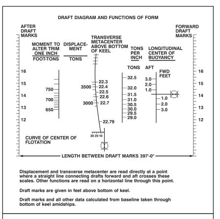
Figure 3-7. Draft Diagram and Functions of Form for the FFG-7 Class Frigate.
