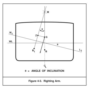
The length of the righting arm varies with the angle of inclination. The ratio of the righting arm to the metacentric height, GZ/GM, is equal to the sine of the angle for any small angle. If the sine of the angle is represented by Sin  $\theta$ , the equation can be written as:
