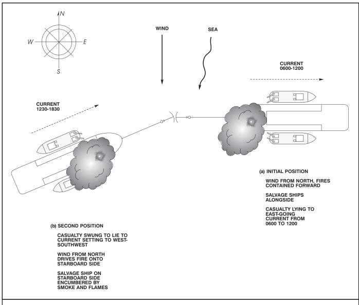
Figure 19-8. Effects of Major Alteration of Current on Fire Front Direction.
