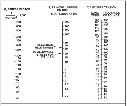
Figure 12-17. Hull Stress Nomogram.
