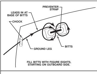
Figure 9-1. Making Up Pendants to Bitts Correctly.
