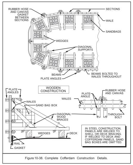
**10-3.2** Partial Cofferdams. Partial cofferdams surround hatches and large deck openings from which water must be excluded during pumping operations. This type of cofferdam is normally used in conjunction with conventional deck patches and other temporary watertight closures.
