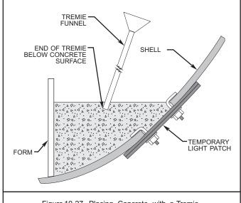
Figure 10-27. Placing Concrete with a Tremie.
