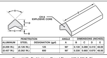
Figure 14-26. Flexible Linear Shaped Charge (125 & 600 Gr Ft).
