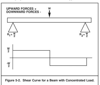
In the beam in Figure 5-2, the only force to the left of any point between  $R_1$  and W is the upward force (equal to +W/2) at the support; shear force at this point is therefore +W/2. The shear force can be calculated at several points along the length of the beam and plotted on a graph as a shear curve. Shear is determined for points immediately to the right and left of concentrated loads and assumed to change abruptly at the point of loading.
