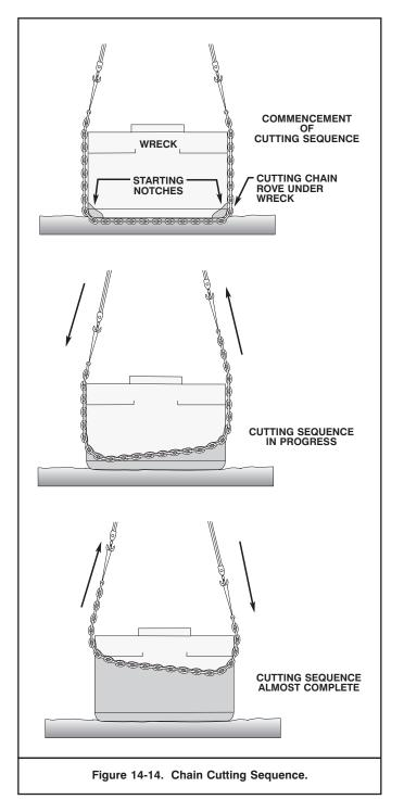
In some cases, starting notches may have been pre-cut by an advance team so crane barge crews and divers rig cutting chains into pre-cut notches or a previously attempted cut line. Some pre-cutting of heavy structural section, such as propeller shafts and machinery foundations, may be necessary and advisable if hull cuts are to be made in such areas. Chain cutting through machinery spaces should be avoided whenever possible.
