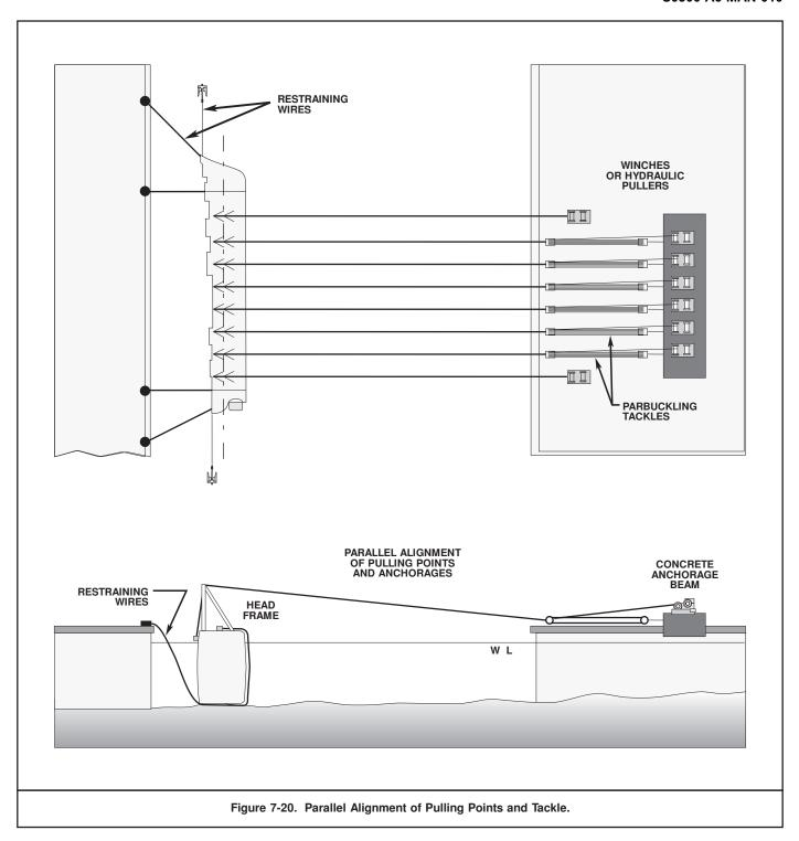
**7-8.4.1** <u>Headframe Attachment Position</u>. To ensure that each purchase or pulling system develops almost identical righting moments, headframe top and hauling system anchorage point baselines must be in the same plane. To achieve this, it is customary to locate all headframe attachment positions on the capsized ship's parallel midbody.
