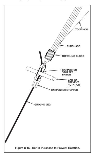
c. Carpenter stoppers. Carpenter stoppers are sliding wedge block wire rope stoppers that hold wire rope without damage up to breaking strength. Four Carpenter stoppers are used in each purchase beach gear leg. Two 5/8-inch stoppers are used for hauling and holding the purchase rope, and two 15/8-inch stoppers to haul on and hold the ground leg.
