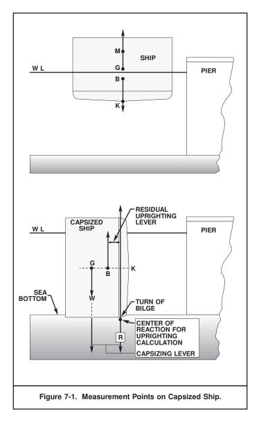
Refloating the ship in such a way that it rotates so it is totally
