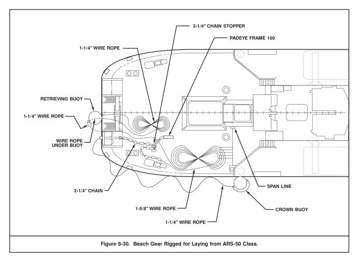
Direct pull and purchase ground tackle systems are carried in the ARS-50 Class. The primary pulling system uses linear pullers. Two of the pullers are operated with installed hydraulic power units, and two, with portable power units.
