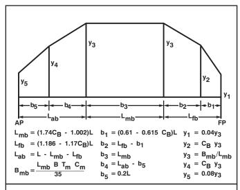
Figure 5-11. Approximate Buoyancy Curve for Full-Bodied Ship.
