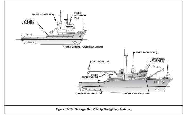
**17-3.2** Offship Delivery Capability. In addition to large-capacity pumping systems, salvage ships have specialized systems to deliver water and foam to a fire on the casualty. Delivery systems include
