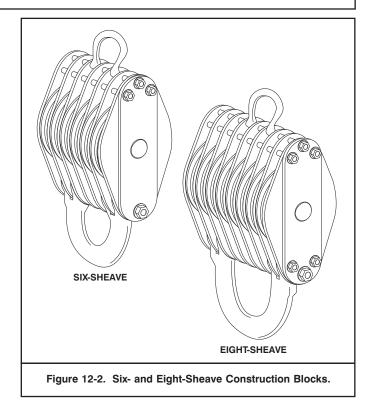
rope. The larger blocks are used in salvage operations only as permanent rigging on salvage sheer legs, crane barges, or pulling barges.
