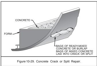
In larger patches, burlap bags of concrete may provide bulky keys in the patch as the concrete is poured.
