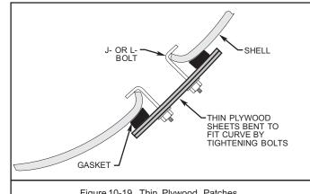
Figure 10-19. Thin Plywood Patches.
