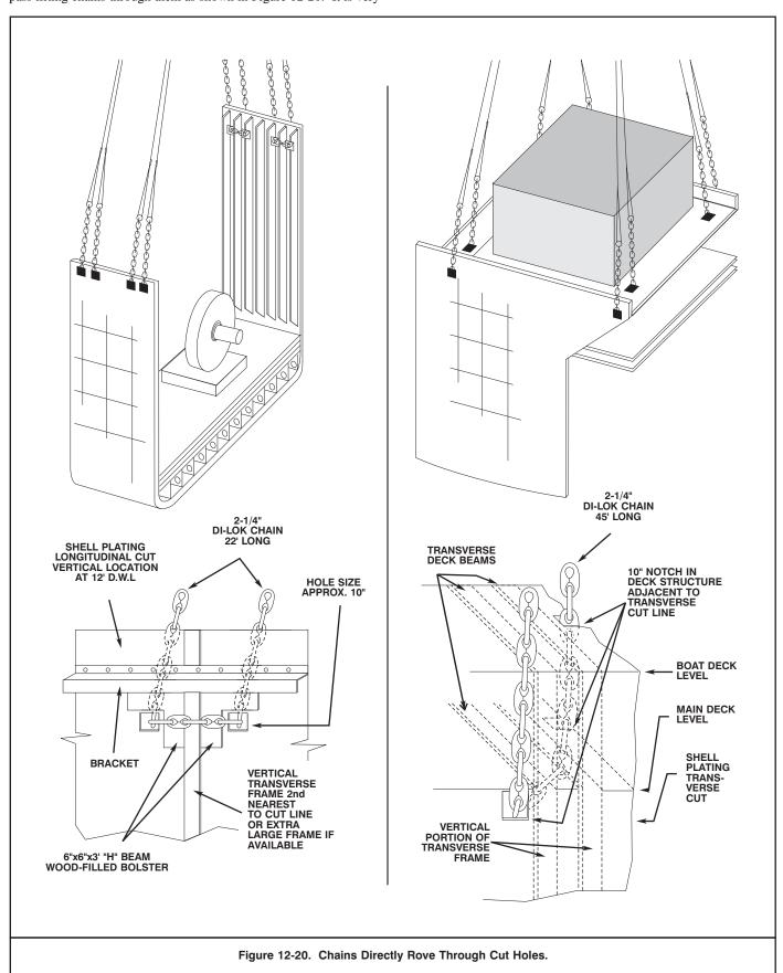
In harbor clearance operations, it may be necessary to cut holes and rig lift chains into the plating of small sunken ships or wrecks to be moved urgently.
