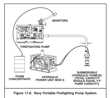
17-3.4 Navy Portable Firefighting Pump Module. NAVSEA has developed a portable firefighting pump module modeled after commercial fire pumps. The module is a complete, skid-mounted, firefighting package ready for deployment to a casualty from salvage ships, platforms of opportunity, or shore-based warehouses. The module, illustrated in Figure 17-8, may be set up as an independent system or tied into a salvage ship's offship firefighting manifold.
