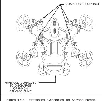
Figure 17-7. Firefighting Connection for Salvage Pumps.
