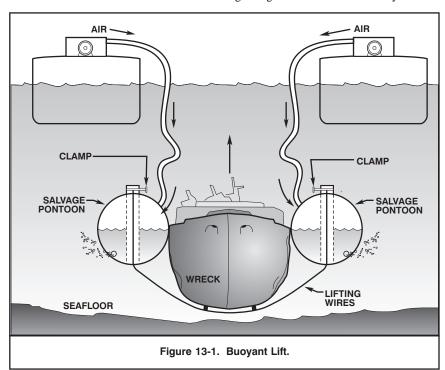
Collapsible, inflatable lift bags (variable-volume devices) and rigidsteel pontoons (fixed-volume devices) are the only buoyant lift devices that have been consistently successful in salvage.
