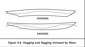
Hogging and sagging are two conditions that reflect weight and buoyancy distribution. When a ship is hogging, buoyancy exceeds weight in the midships region and weight exceeds buoyancy near the ends. The distribution of forces tends to bend the ends of the ship downward. The opposite condition is called sagging. These conditions are shown in Figure 5-8.
