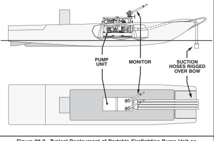
Figure 20-2. Typical Deployment of Portable Firefighting Pump Unit on Standard 35-Foot Salvage Work Boat.
