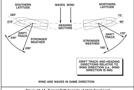
Figure 18-4A. Typical Drift Aspects of High-Freeboard Ships in Wind Force Beaufort 9.
