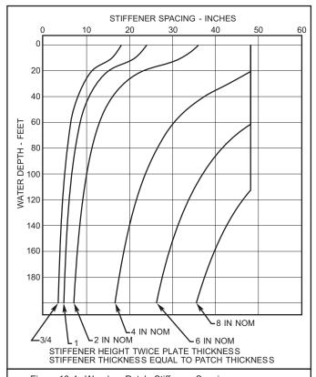
Figure 10-4. Wooden Patch Stiffener Spacing.
