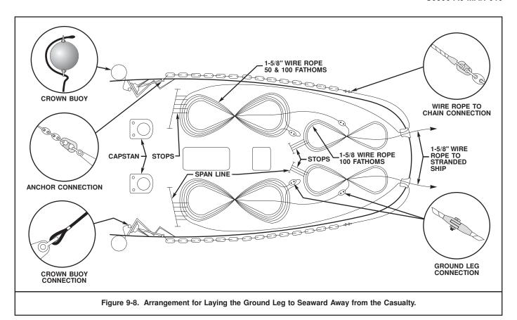
Beach gear can be laid to assist in wrenching or in holding the ship perpendicular to the beach. Wrenching and holding legs may make a contribution to the pulling effort. They should be tensioned when maximum pull is applied and slacked when the ship begins to move.
