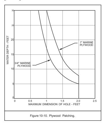
**10-2.2.2 Measurements and Templates for Patches.** This paragraph discusses techniques for measuring, planning, and checking the dimensions and contours of patches.
