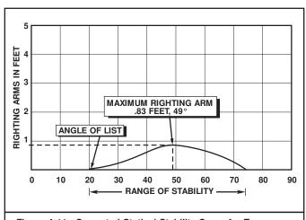
Figure 4-11. Corrected Statical Stability Curve for Transverse Shift in G.
