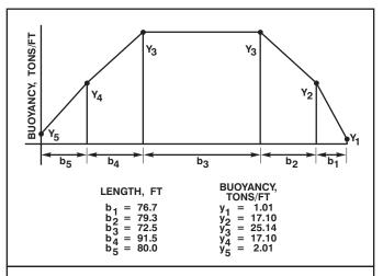
Figure 5-12. Approximate Buoyancy Curve for Example 5-4.
