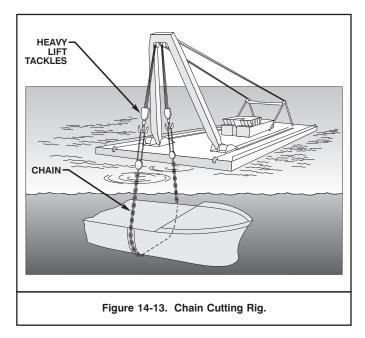
**14-5.1.1** Advantages and Disadvantages of Chain Cutting. Chain cutting of wrecks has advantages and disadvantages. The advantages include:
