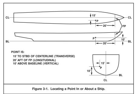
**3-2.1.2** <u>Location of Points</u>. The position of any point in the ship can be described by measuring its:
