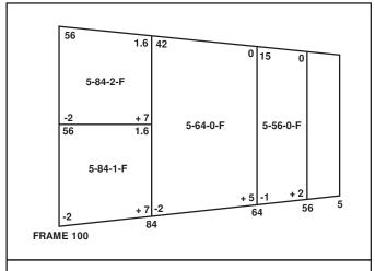
Figure 3-5. Sample Liquid-Loading Diagram Format.
