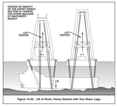
Most salvage sheer legs are designed so that their A-frames may be rigged down for tow. The A-frame is self-erecting.
