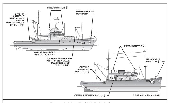
Figure 17-2A. Salvage Ship Offship Firefighting Systems.
