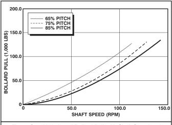
Figure G-1. Variation of Bollard Pull with Shaft Speed and Propeller Pitch for ARS-50 Class Ships.
