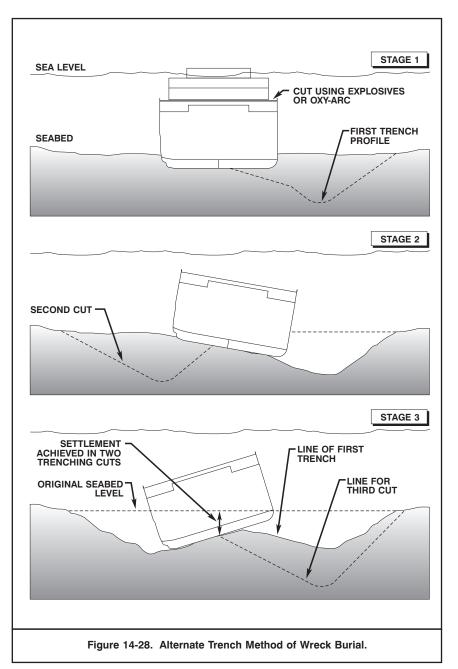
**14-7.2.1** Ship Settling. Ship settling is making a sunken wreck entrench itself deeper into the seafloor. Ship settling may be the sole method of lowering a wreck to increase depth over it, or may be done in conjunction with ship flattening or wreck dispersal. Suitable soil conditions must exist for explosive ship settling to be successful. Soft sand or muddy seafloors permit settling, but hard clay soil may present some difficulties. Wreck settlement is done by:
