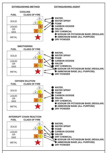
Figure 16-4. Actions of Extinguishing Agents on the Different Classes of Fire.
