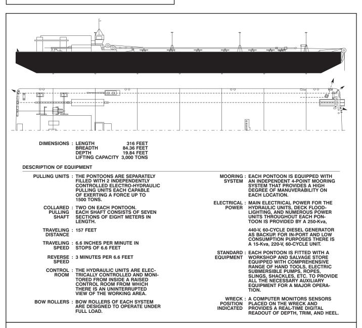
Figure 13-21. Pull and Lift Barge.
