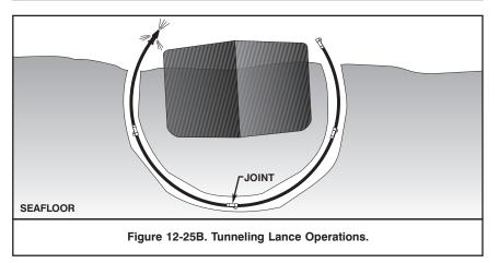
narrow defiles has considerable value for some salvage operations. Salvors have used dredges to cut and excavate lift and pulling wire tunnels on many occasions; the method should not be ignored if suitable dredging equipment is available.
