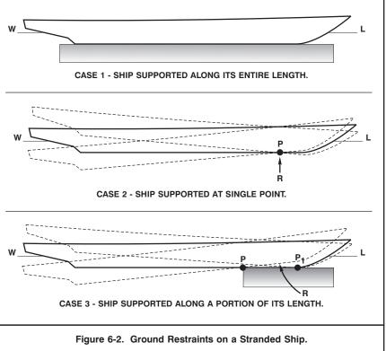
**6-3.3.1 The Neutral Loading Point.** A grounded ship often has a point where weight can be added or removed without changing the ground reaction; this point is the neutral loading point. The neutral loading point is the point at which weight addition causes parallel sinkage at the effective point of grounding that is exactly balanced by the change of trim, or:
