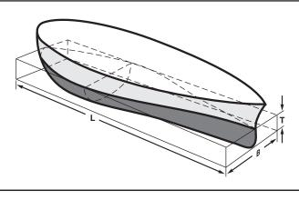
Figure 3-2. Block Coefficient Relationship.
