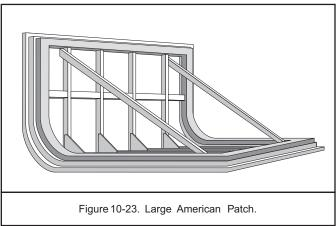
**10-2.2.6** <u>Built-up Patches.</u> The built-up, plate-on-plate, or plank-on-plank patch is a series of narrow strips—steel plates or wooden planks—laid in across the damage and fixed in-place individually. These patches are custom-built for the damage, and unlike box patches, require a lot of diving time.
