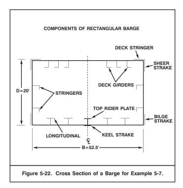
When the bending moment and section modulus have been calculated, the bending stress can be calculated using the method given in Paragraph 5-5.1.
