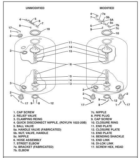
Figure 13-9. 8.4-ton Inflatable Salvage Pontoon.
