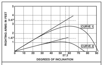
Figure 4-12. Metacentric Height from Statical Stability Curves.
