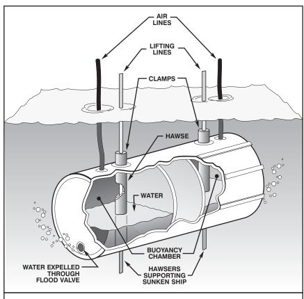
Figure 13-7. Partially Flooded Salvage Pontoon.
