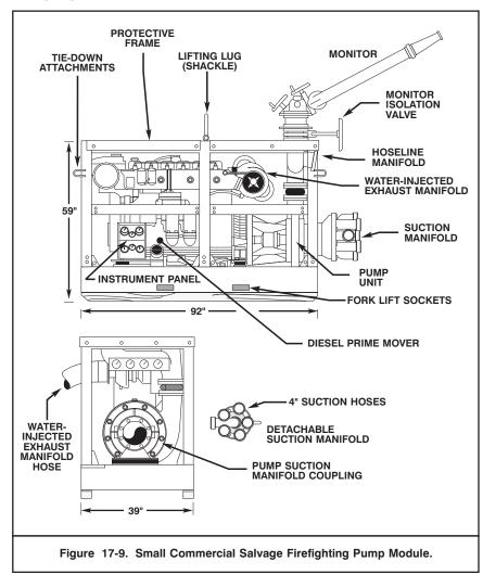
The complete module is packaged for air transport and helicopter slinging. The 6-inch hydraulic submersible pump can be rigged to the firefighting module to increase suction lift.
