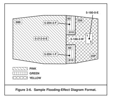
Each tank is colored to indicate its use in accordance with the color code given on the actual diagram. The data given for list and trim are based on a specified condition of loading and may not be applicable when the ship is unusually loaded or severely damaged.
