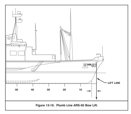
With two combinations of deck machinery, the ARS-50 Class ships can make bow and stern lifts of 75 tons per wire. These arrangements include:
