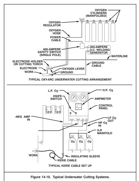
**14-4.1** <u>Underwater Manual Cutting.</u> Diver-operated manual cutting systems are used on almost every wrecking-in-place operation. Work assigned to underwater cutting teams ranges from cutting hull-section slinging holes to cutting entire hulls. The success and speed of underwater cutting depends upon several factors including:
