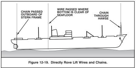
Cranes, bridges, and other sunken structures often encountered in harbor clearance operations are frequently directly rove. The open lattice and chord construction, and the inherent strength of crane and bridge sections, make them especially suitable for this method. A direct reeving method used in piecemeal demolition of wrecks is to cut lifting holes in the shell or deck several frame spaces apart and to pass lifting chains through them as shown in Figure 12-20. It is very
