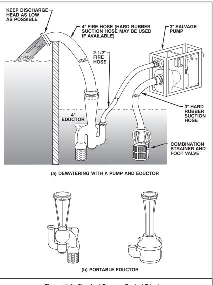
Figure 11-3. Standard Damage Control Eductor.
