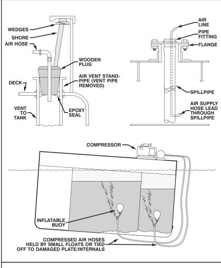
Figure 21-1. Emergency Compressed Air Fittings.
