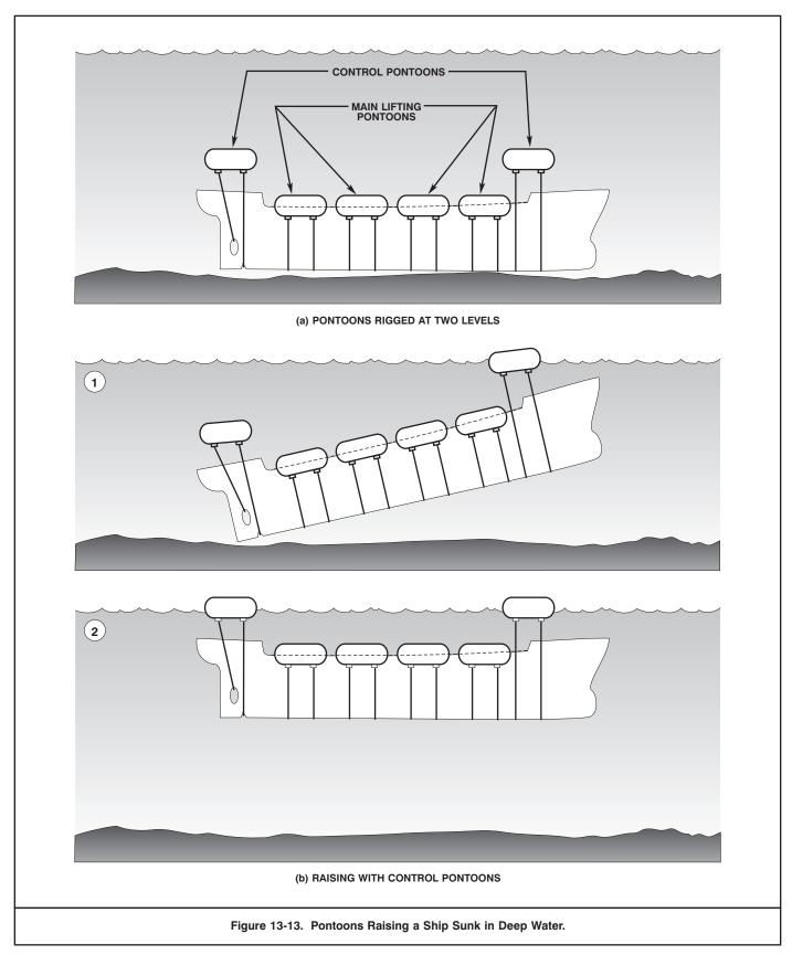
Deeply sunken ships raised with pontoons in one step accelerate as they rise and trim, despite the best efforts of salvors to balance the lift. Lack of control in such a raising often leads to damage to the ship or pontoons. Sometimes such an evolution results in the ship's surfacing only briefly before sinking again in a tangle of lift gear.
