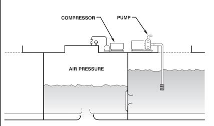
Figure 11-17. Combined Pumping and Blowing as the Most Appropriate Method for the Space Being Dewatered.
