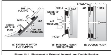
Figure 10-1. Placement of External, Internal, and Double Patches.
