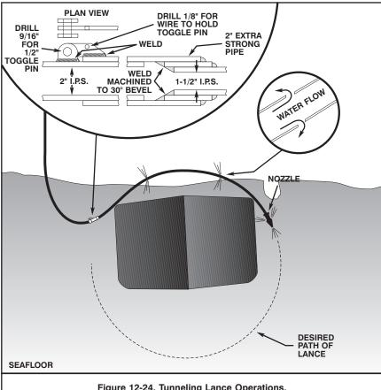
Figure 12-24. Tunneling Lance Operations.
