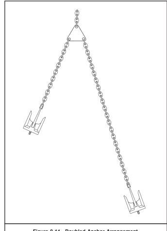
Figure 8-11. Doubled Anchor Arrangement.
