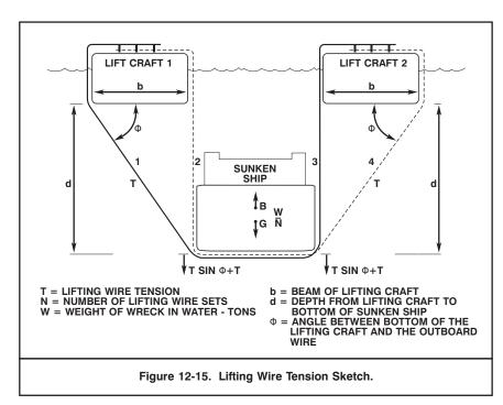
Figure 12-15 shows a typical lift configuration. Each wire is rigged from one lift craft under the wreck to the other lift craft. There is a pair of wires at each transverse location. Each pair of wires has four lifting parts. The total of the vertical components equals the wreck's weight in water. The wire tension may be calculated by:
