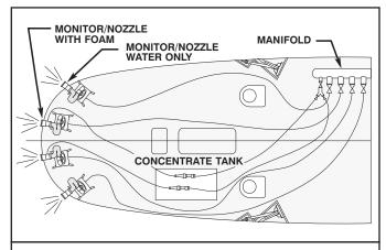
Figure 17-6. Offship Manifold and Portable Equipment.
