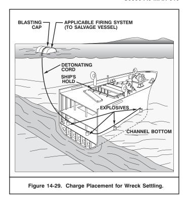
**14-7.3** <u>Cutting Down Wrecks</u>. Sometimes navigational obstructions can be reduced by cutting a wreck down to a specified depth below a specified water level. Clearance levels over wrecks are established by port or area operating authorities with regard to present and future traffic.
