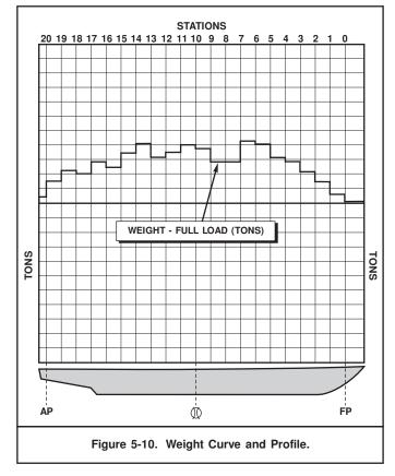
The positions of variable weights may be determined from arrangement and loading plans. Weights are placed in the proper position along the length of the hull. After all variable weights have been accounted for and subtracted from the displacement, the remaining weight is the lightship weight. The weights of major components, like superstructures and machinery, can be estimated and placed in position by
