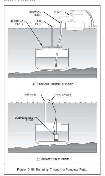
Construction of pumping plates for shallow water work is not a particularly difficult task. If the technique is applied in more than 6 feet of water, the deck and plate must be shored against the water pressure.
