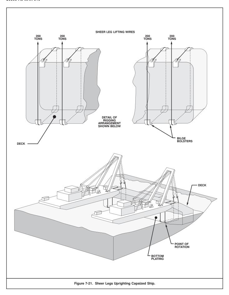
Salvage engineers will advise what areas of the hull have enough strength and will devise stiffening for on-site or shop fabrication. In some cases, internal pillaring, local shoring, or comprehensive stiffening may be necessary.
