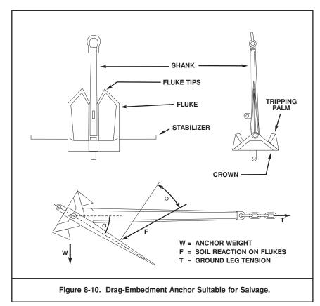
Drag-embedment anchors are manufactured in a wide variety of sizes and shapes, but all have common characteristics. As shown in Figure 8-10, drag-embedment anchors suitable for salvage are made up of the following parts:
