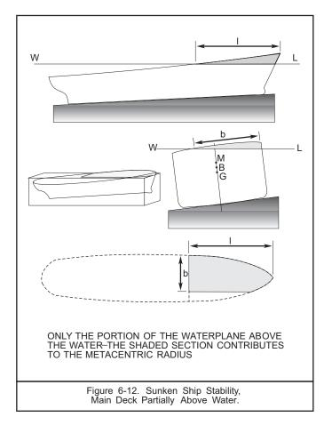
Because of the contribution of length to the longitudinal moment of inertia of the waterplane, ships with any significant length of waterplane are inherently longitudinally stable. In ships with little or no internal transverse subdivision, free surface may present a major problem while the ship is being raised.
