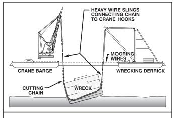
Figure 14-16. Two Crane Barges Operating a Sawing Chain.
