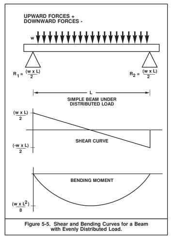
If the weight is evenly distributed along the length of the beam, the shear curve will pass through zero at the center of the beam and the bending moment curve will be a parabola with its maximum at center of the beam.
