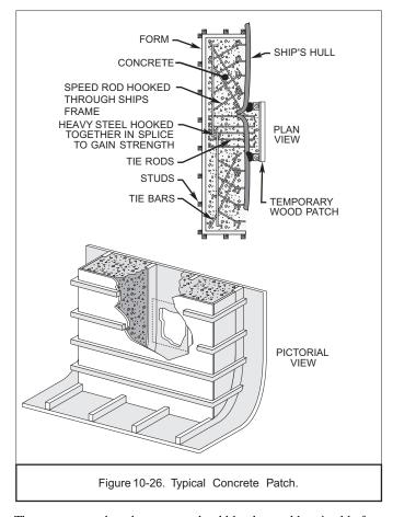
The cement, sand, and aggregate should be thoroughly mixed before the water is added. To produce the correct consistency, the final mixture of underwater cement should be stiff. It should be only soft and pliable enough for the diver to work the concrete into the corners of spaces to be filled.
