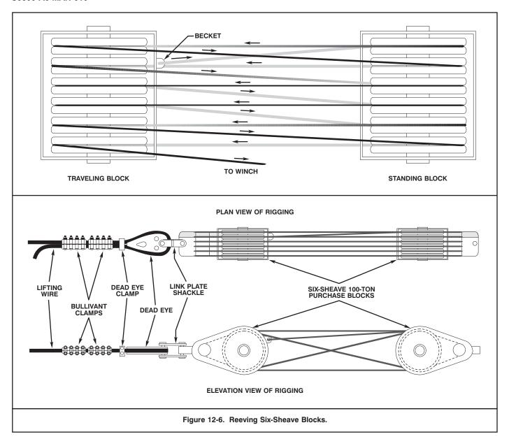
Large horizontal purchases usually are rove with reverse bends to counter the torque that twists the purchase and capsizes the traveling blocks. Figures 12-6 and 12-7 illustrate common reeving systems for six- and eight-sheave blocks. Both systems incorporate two reverse bends and have the bitter end of the purchase wire dead-ended to the traveling block.
