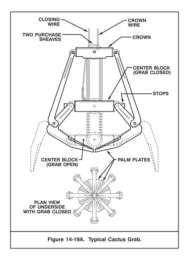
A typical cactus grab is shown is Figure 14-19A. This type of grab is useful on small wrecking-in-place projects and as an all-purpose rehandling grab on large wrecking projects. Orange peel grabs may have a different arrangement of grab leaves and tine points depending upon their design and origin.
