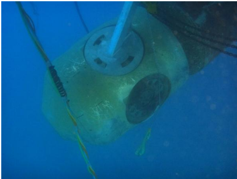
TAYLOR's old hub with blades removed and hub davit installed.
