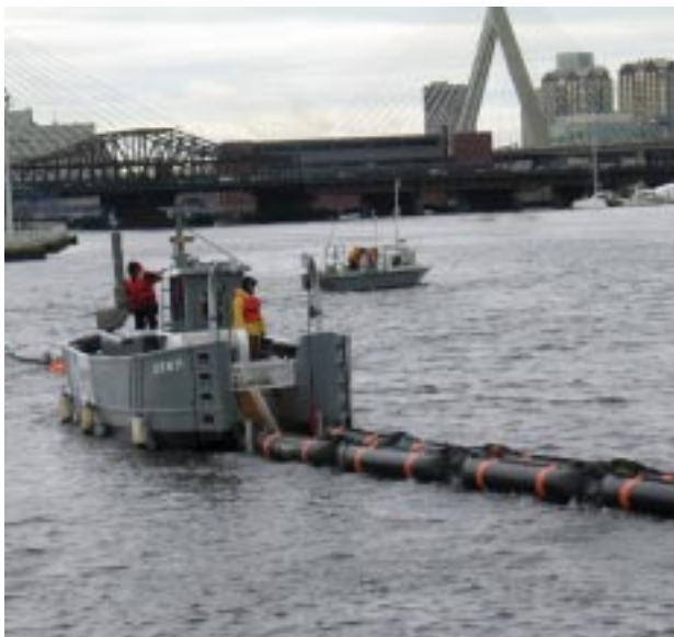
SUPSALV’s MARCO Class V Skimmer System herds the oil with its 300-foot boom legs and picks up the oil via a belt system seen here. The oil is then pumped into the oil storage bladder shown in tow behind the vessel.
