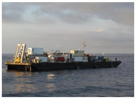
**Saturday May 5 2012.** SATFADS diving system loaded on a barge and moored in the Gulf of Mexico. That afternoon, the team performed unmanned testing at 490fsw and on 6 May the diving bell was tested at 1100fsw.
