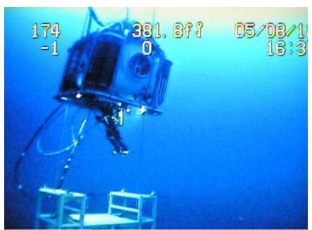
**Tuesday, May 8:2012.** With 6 divers in the saturation complex habitat, the system was pressurized to a depth of 350fsw (feet of seawater). A dive bell excursion was conducted locking out all 3 bell divers to a depth of 392fsw. This image shows the first diver exiting the diving bell and lowering himself to the diver's stage.
