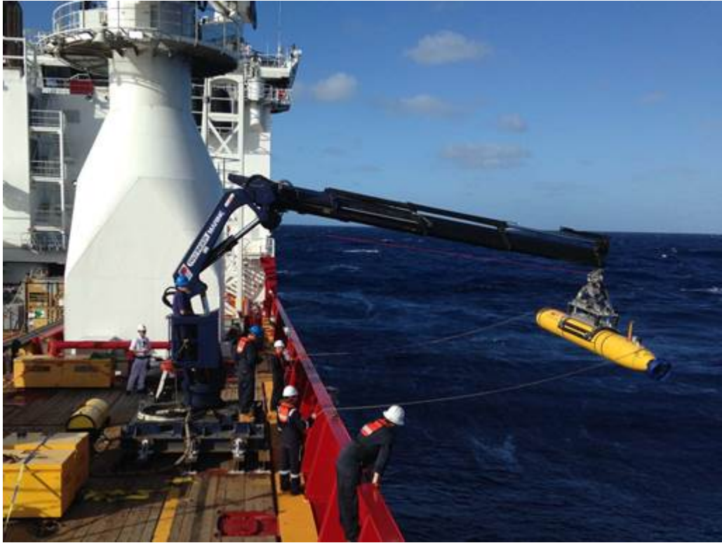
Phoenix's Autonomous Underwater Vehicle (AUV) "Artemis" is lowered into the sea for testing on 1 April. The AUV is supplementing the Navy's TPL in the search for Malaysian Air Flight 370. The AUV is capable of diving a preprogrammed route and searching using side scan sonar device and would be deployed if the TPL picks up a possible signal.
