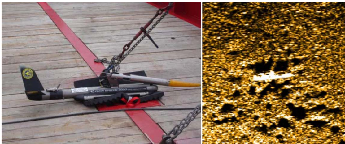
Pictured left, SUPSALV's side scan sonar – SWISS on deck of the M/V Marie Elise. On the right is a side scan image of the MALD vehicle on the ocean floor.
