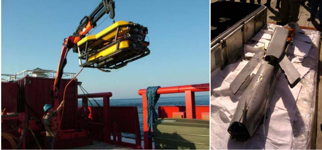
On the left is the ROV used to recover the MALD. At right, the MALD on deck after recovery.
