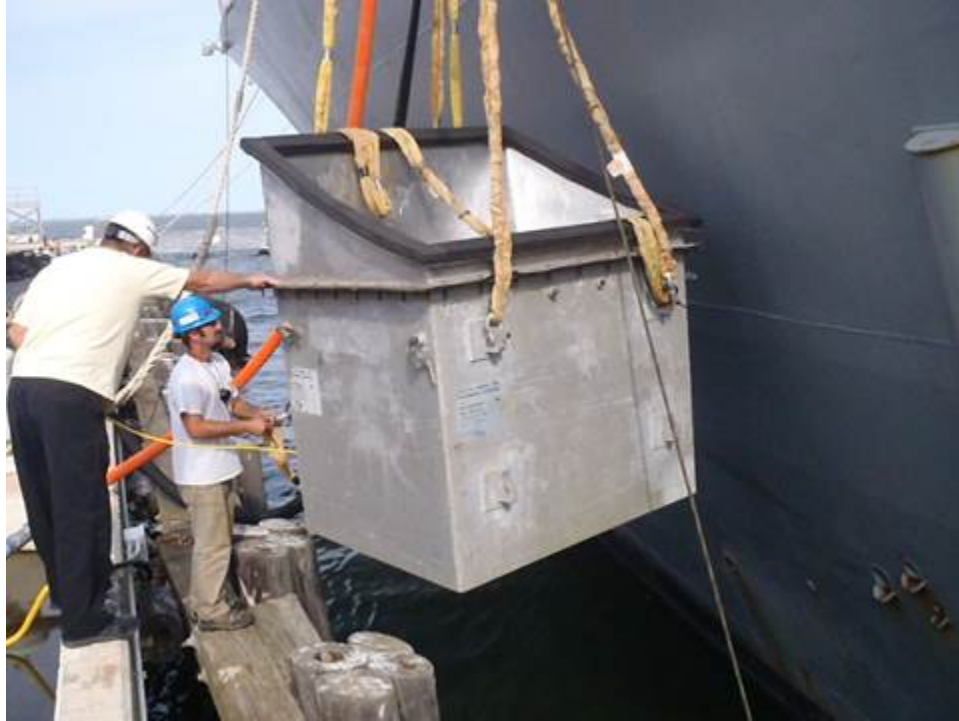
An example of a habitat being deployed from the pier. After the dry chamber is positioned against the hull of the ship and blown down with air, the diver enters from the bottom.
