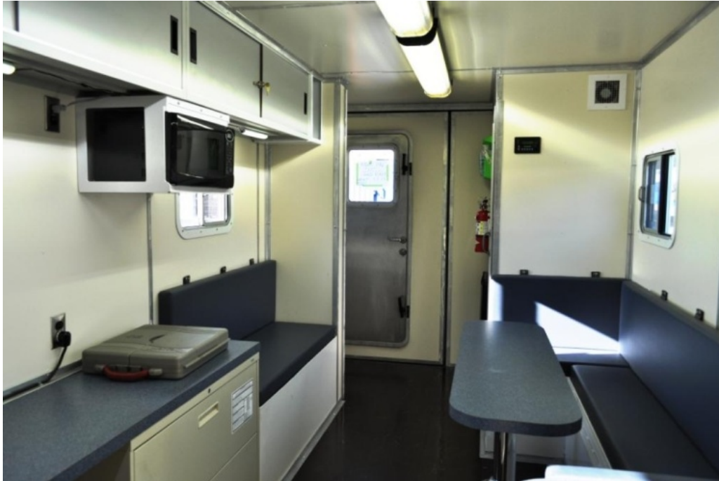
Figure 3. View looking toward the Van entrance showing additional work areas, microwave oven, power converter meter (on right wall), storage areas, and seats that store the Li ion batteries. The advanced battery monitoring and electrical distribution system is housed in the locker to the right of the van's entrance.
