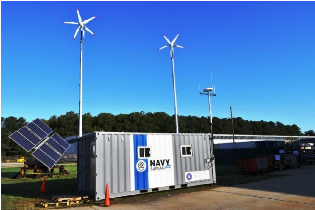
Figure 1. The complete exterior setup: Command Van with wind turbines, satellite, antennas and solar panels.
