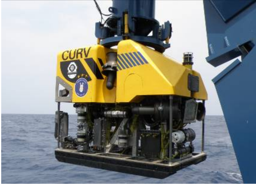
File photo of CURV-21, a 6,400-pound Remotely Operated Vehicle (ROV) that is designed to meet the US Navy's deep ocean salvage requirements to a maximum depth of 20,000 feet of seawater.
