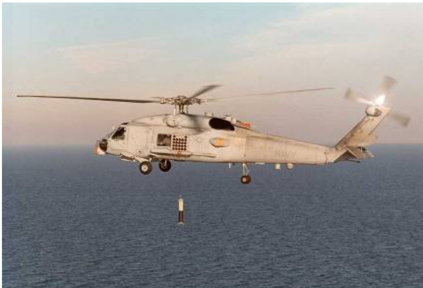
File photo of Navy SH-60 LAMPS helicopter with the AN/AQS-22 Airborne Low Frequency Sonar (ALFS) suspended from it. NAVAIR tasked SUPSALV to find a missing ALFS that was lost in the Atlantic Ocean.
