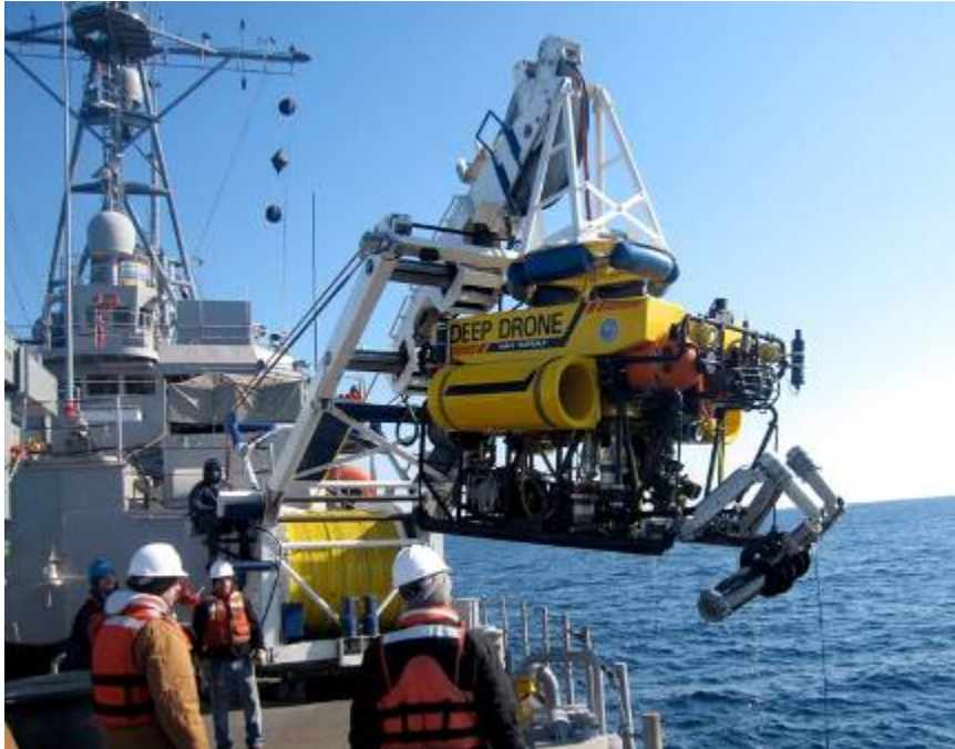
Deep Drone being retrieved onto USNS GRAPPLE the morning of 29 January, 2011. In Deep Drone's manipulators is the ALFS which was recovered within 14 minutes of being at search depth near the sea floor.
