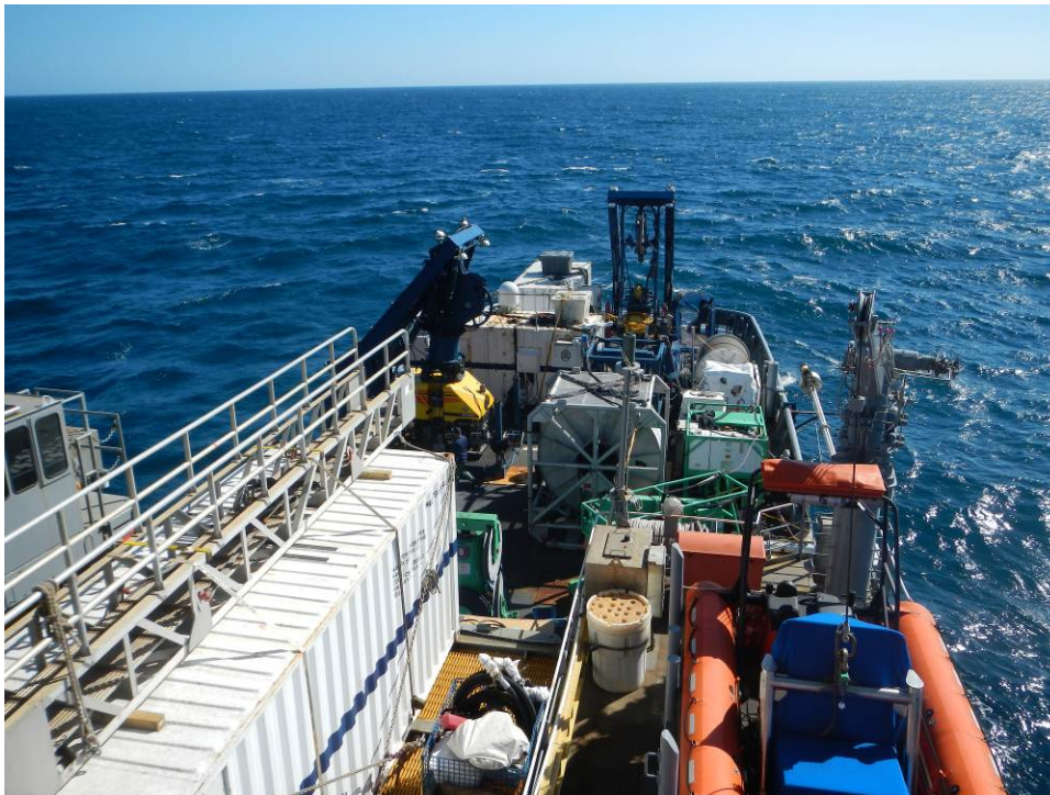
Stern deck of USNS NAVAJO at sea, enroute OPAREA. Major systems on deck include: FADOSS, just astern of rigid inflatable hull (RIB) boat, CURV to left, astern of white control van and Orion side scan sonar at stern.
