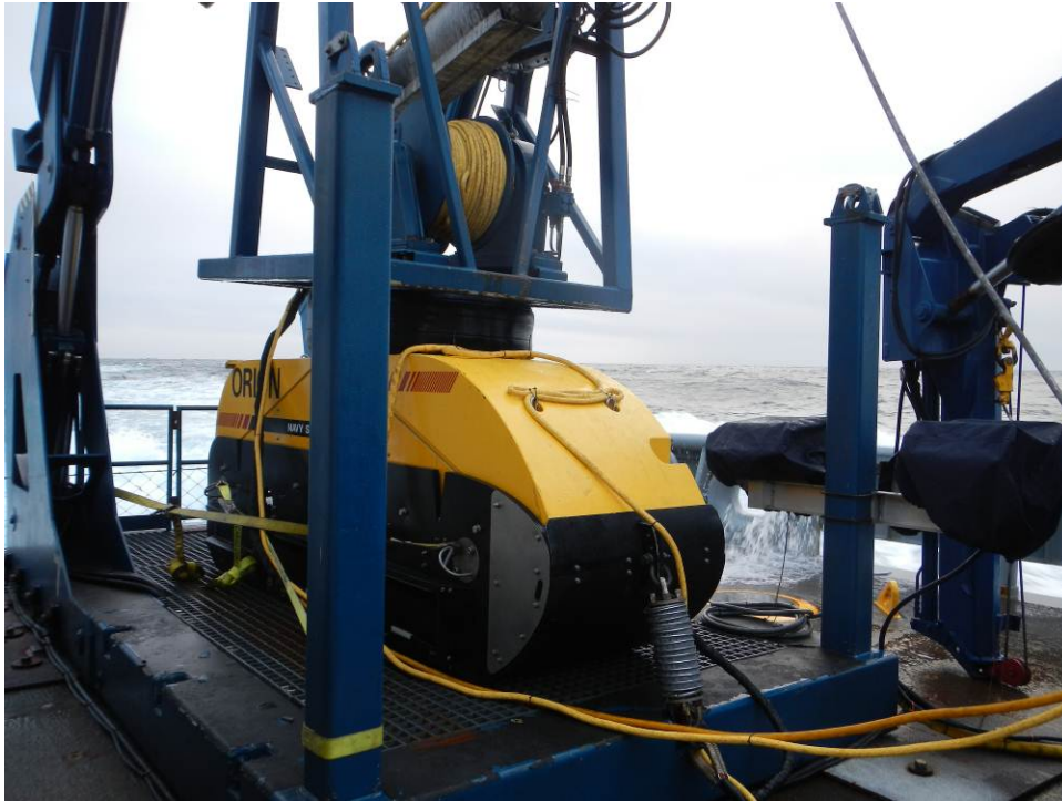
Side Scan Sonar, Orion at the stern of USNS NAVAJO ready for launching on 1 September 2012
