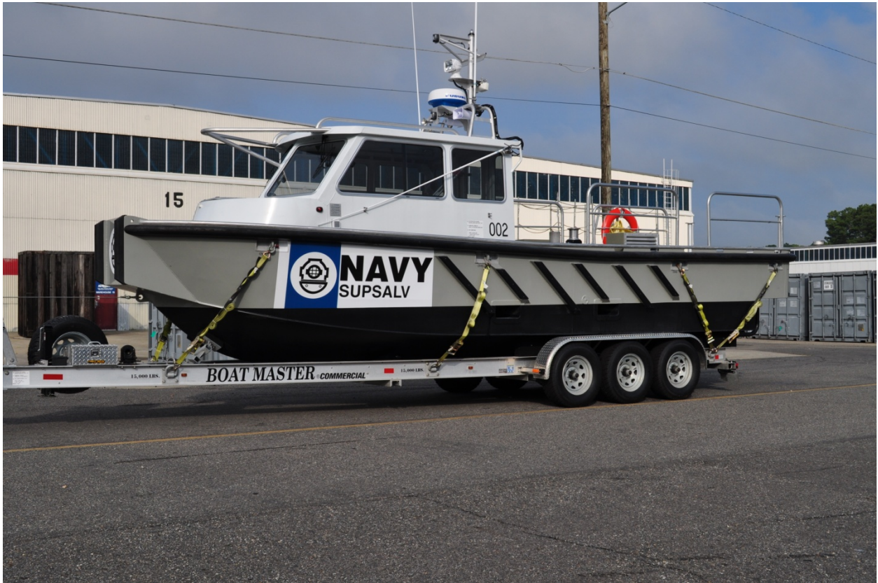
Figure 10-12. 30' Boom Handling Boat
