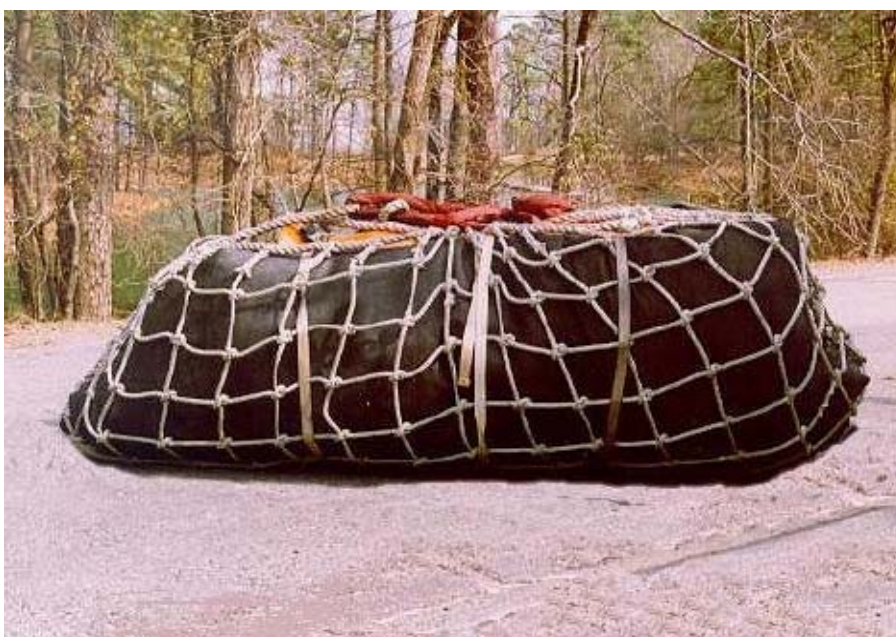
Figure 10-5. 21–26K Gallon Spill Recovery Bladder
