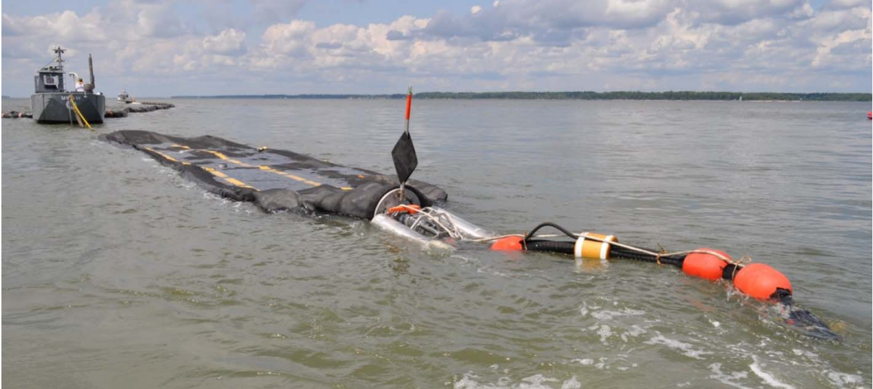
Figure 10-6. At Sea Bladder Pumping System Attached to a 21K Gallon Oil Storage Bladder
