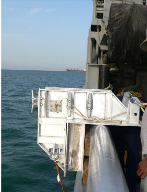
Figure 10-52. Tabernacle Mounted on T-ATF Bulwark
