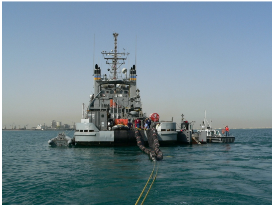
Figure 10-44. Deploying Skimmer Boom
