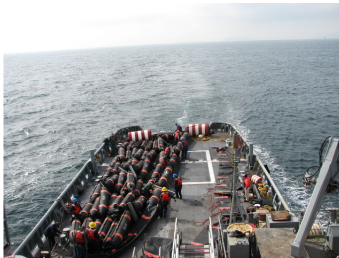
Figure 10-63. Boom and Mooring Systems Positioned for Deployment Aboard a T-ATF
