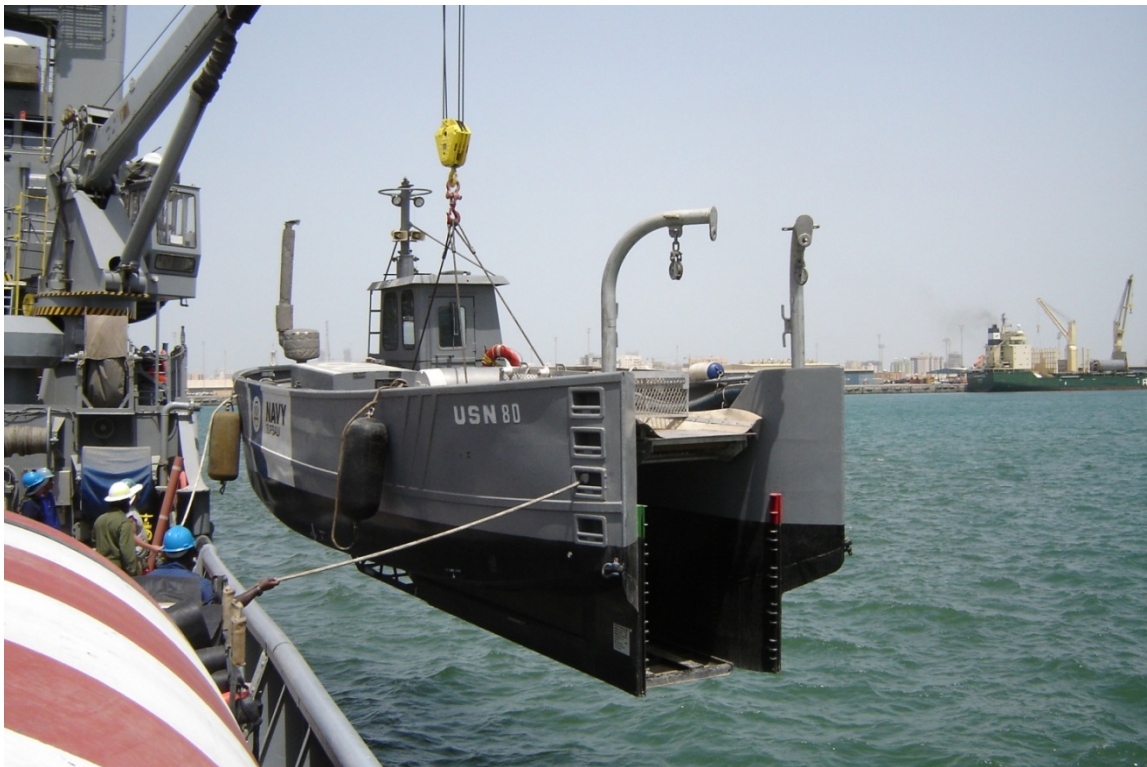
Figure 10-40. Offloading Class V Skimmer Over the Side of the T-ATF
