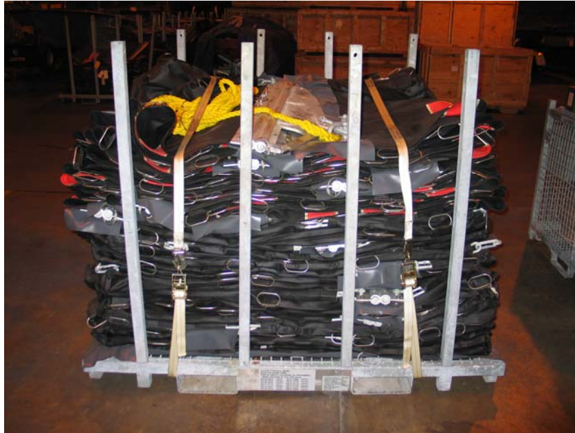
Figure 10-4. USS-42 42" as used with the Marco Class V on the Boom Storage Pallet
