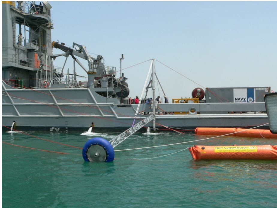
Figure 10-51. King Post with Outrigger Fully Deployed
