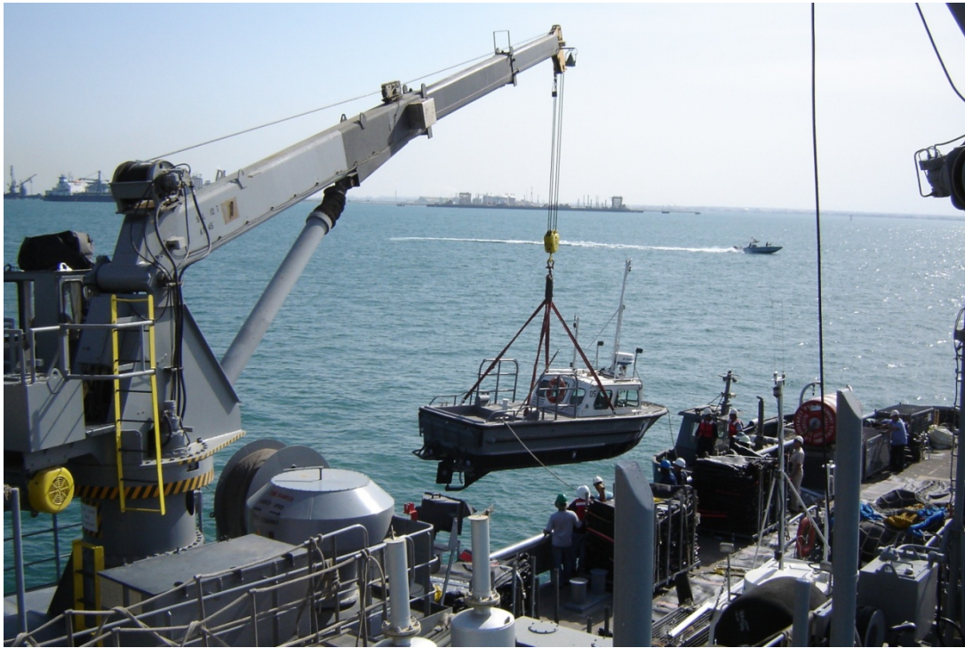
Figure 10-43. Offloading Boom Handling Boat
