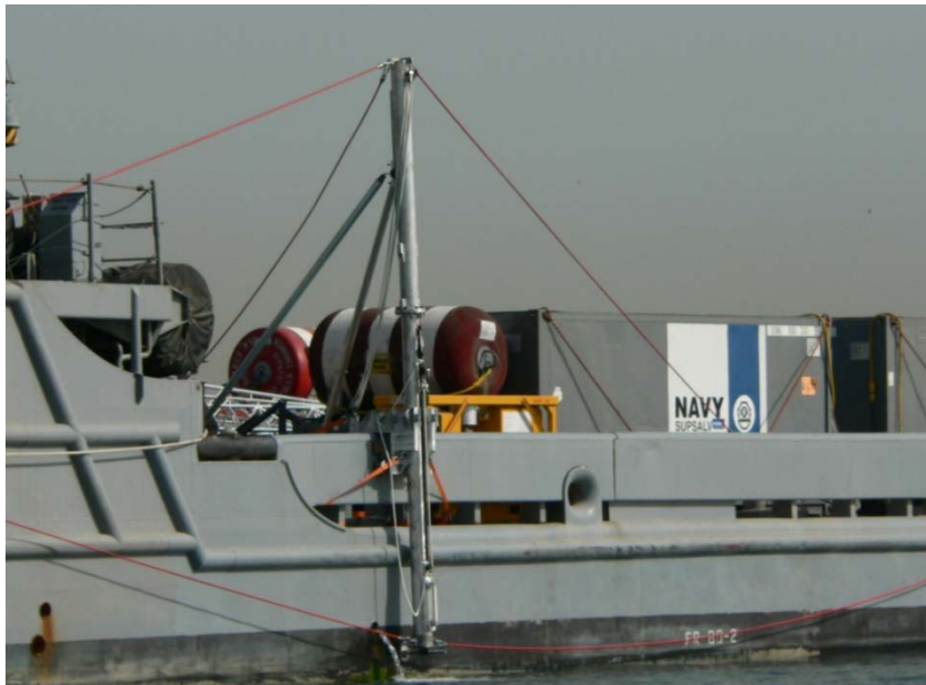
Figure 10-53. Outboard View of the Assembled King Post on the T-ATF
