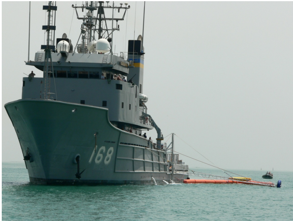
Figure 10-57. T-ATF with High Speed Current Buster Skimmer Underway
