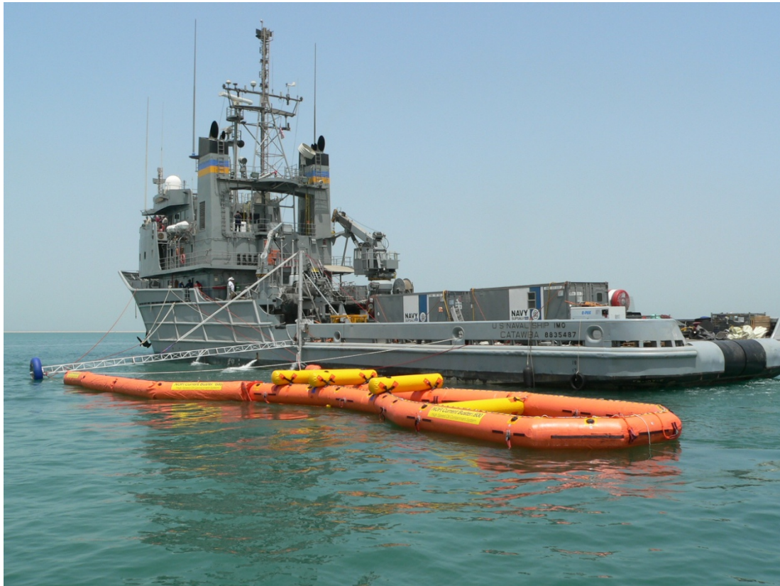
Figure 10-49. T-ATF with High Speed Current Buster Deployed
