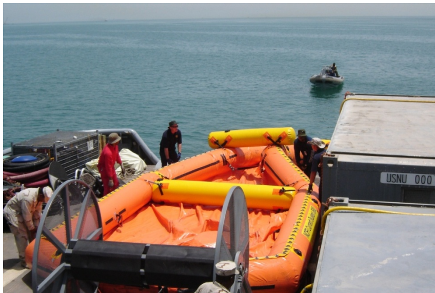
Figure 10-59. Deploying the High Speed Current Buster from the T-ATF
