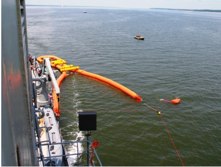
Figure 10-60. Fully Deployed High Speed Current Buster with Paravane
