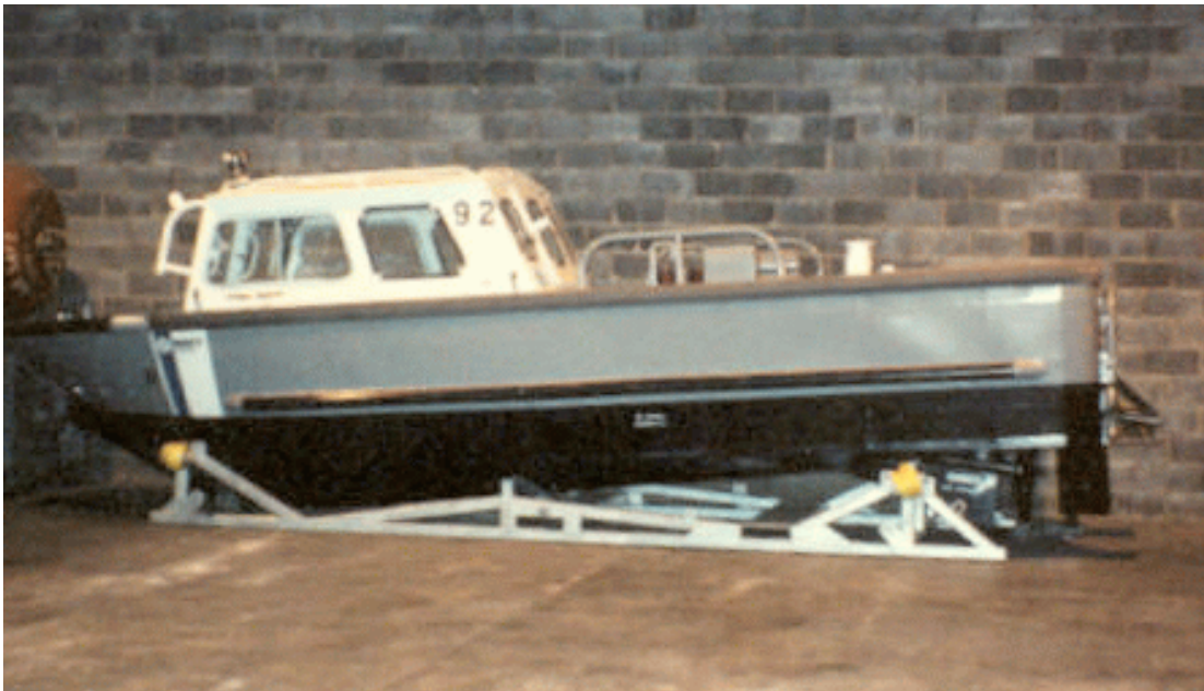
Figure 10-11. 24' Boom Handling Boat
