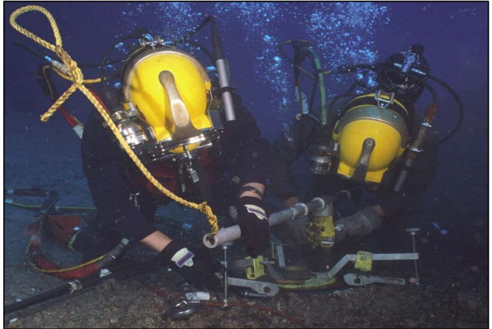
The process begins with identifying an ideal, high suction point on the ship's hull where product is known to be located that is clear of hull features (frames, tank tops, etc.). After identifying the proper location for the hot tap to take place, the hull is thoroughly cleaned of marine growth to ensure the flange gasket can seal properly against the hull, preventing weeping of the petroleum product.
