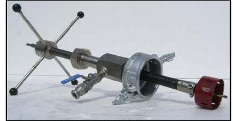
The Lightweight Hot Tap System is designed for tapping in mild steel hull plating up to 1-inch thick. The Tap machine has the capability of tapping a 5 ½ inch hole through a 6 inch knife valve; however, the most practical size of tap is either a 2 5/8 inch hole through a 3 inch full port ball valve or a 3 ½ inch hole through a 4 inch full port valve.
