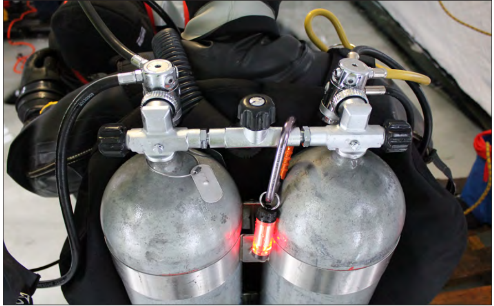
Figure 11-1. Two SCUBA cylinders fitted with two actual redundant first-stage regulators with GLO-TOOB attached.
