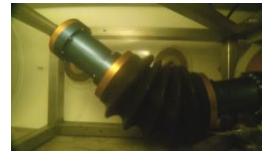
Midé Joint Prototype and Robotic Test Arm During High Pressure Testing at NSWPCD
