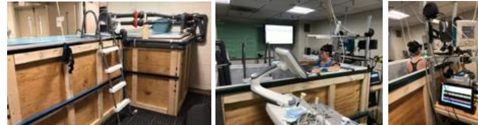
Custom built rapid filling water immersion tanks will allow us to perform complex physiological measurements, such as muscle sympathetic nerve activity, during the studies.
