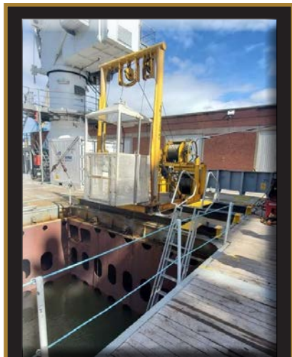
Contracted A-Frame Diver Launch and Recovery System (LARS) installed onboard vessel Olympic Artemis VOO in support of North Sea salvage operations.
