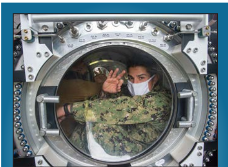
Equipment Operator 1st Class Joseph Rodriguez and Navy Diver 2nd Class Juan Ramirezvelez, both assigned to Underwater Construction Team (UCT) 1, sit in the multi occupant flexible recompression chamber (MORFC) also known as the FLEX chamber, during an equipment demonstration with UCT 1 and Mobile Diving and Salvage Unit (MDSU) Two.
