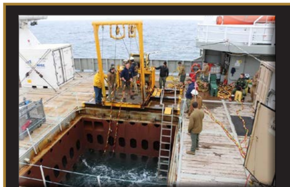
MDSU TWO divers utilizing commercial LARS system during salvage operations in the North Sea.
