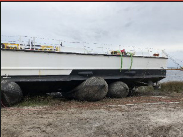
Continued to add bags until running gear was clear of the mud.
