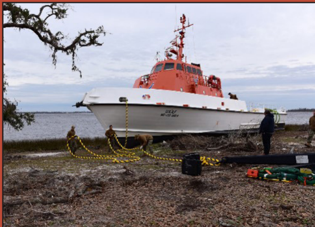
6,000 lb STATO anchor staged on beach for bow restraint.
