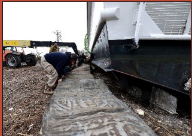
2 bags placed at the stern longitudinally with ship.
