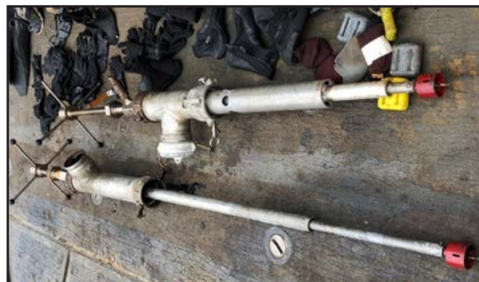
Hot tap extension tool for internal tanks.
