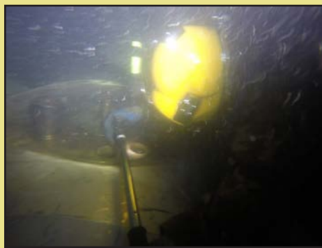
ND2 Noblit (SERMC) torqueing the bolts after a Controllable Pitch Propeller blade replacement on the USS STOCKDALE (DDG 106).
