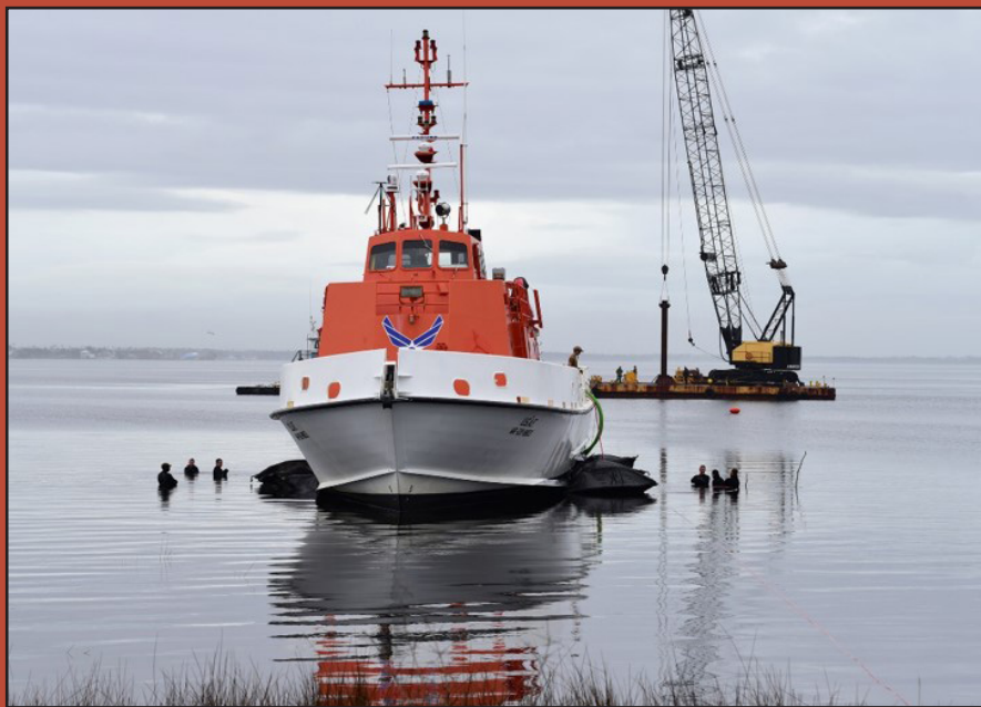
MDSU 2 and SUPSALV personnel using roller bags to refloat USAF MR 8803.
