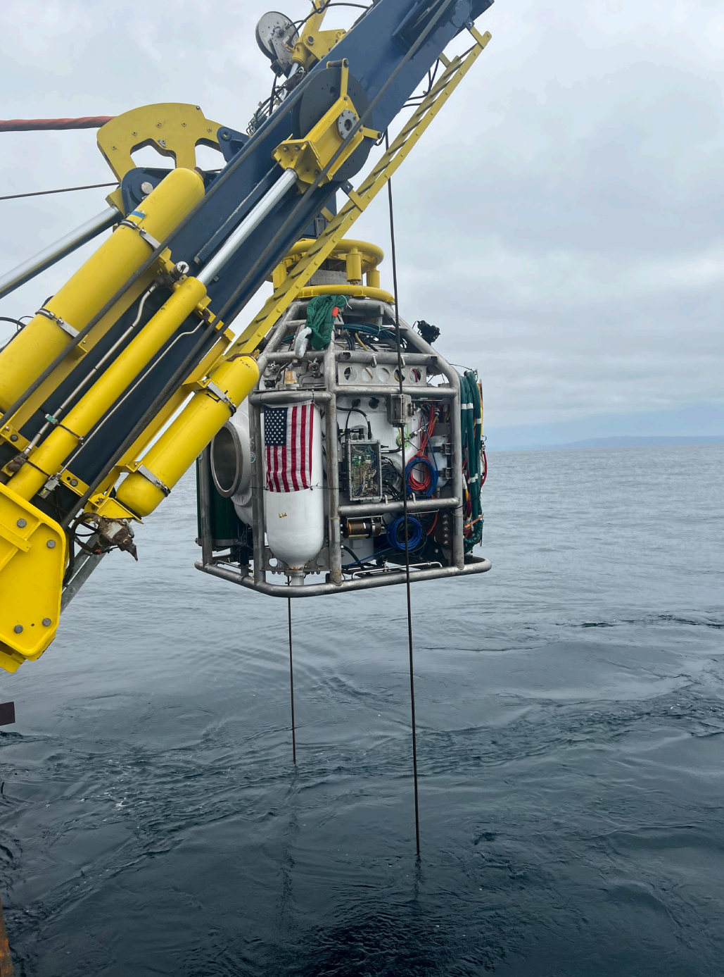
SATFADS dive bell being deployed off the aft deck of the HOS Dominator off the coast of Catalina Island, CA during NSD and URC dual tether saturation and ROV diving operations. Photo by: NDCM Bryan McCurley.
