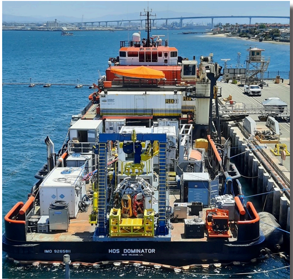
SATFADS assembled and loaded on the aft deck of the HOS Dominator in preparation for at saturation diving operations. Photo by: EMC Shuler.
